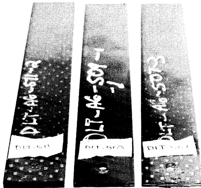
Figure 5-6. Bearing and Shear-Out Failures of Wide DLT Specimens ( W/D = 6 )
