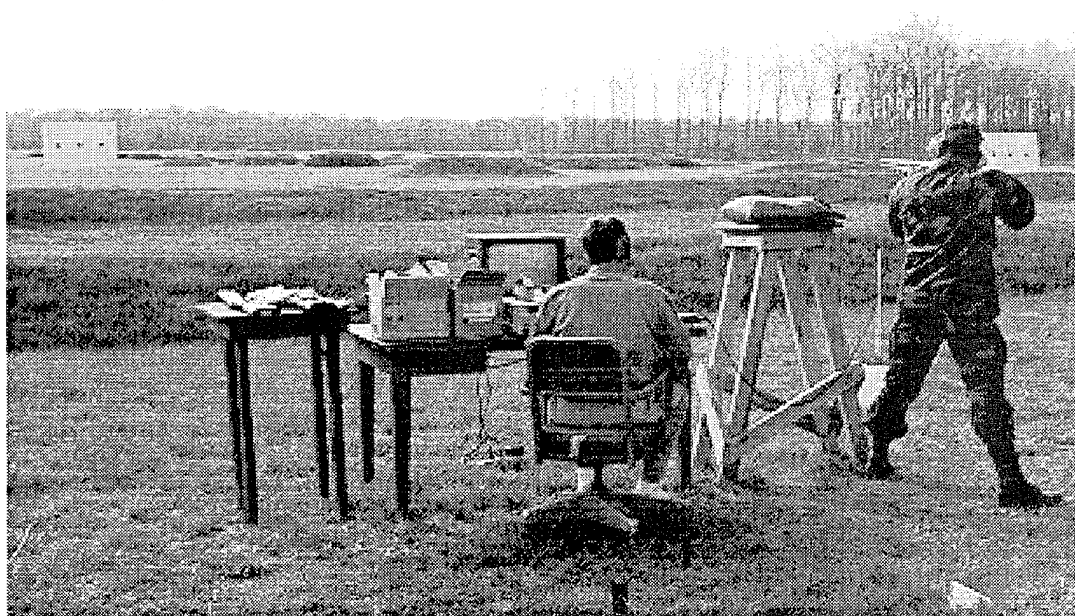
Figure 2. Test setup. (The test subject aimed at the center target of the target board and fired the weapon. Gun-mounted camera and video recording equipment recorded the aiming performance.)
