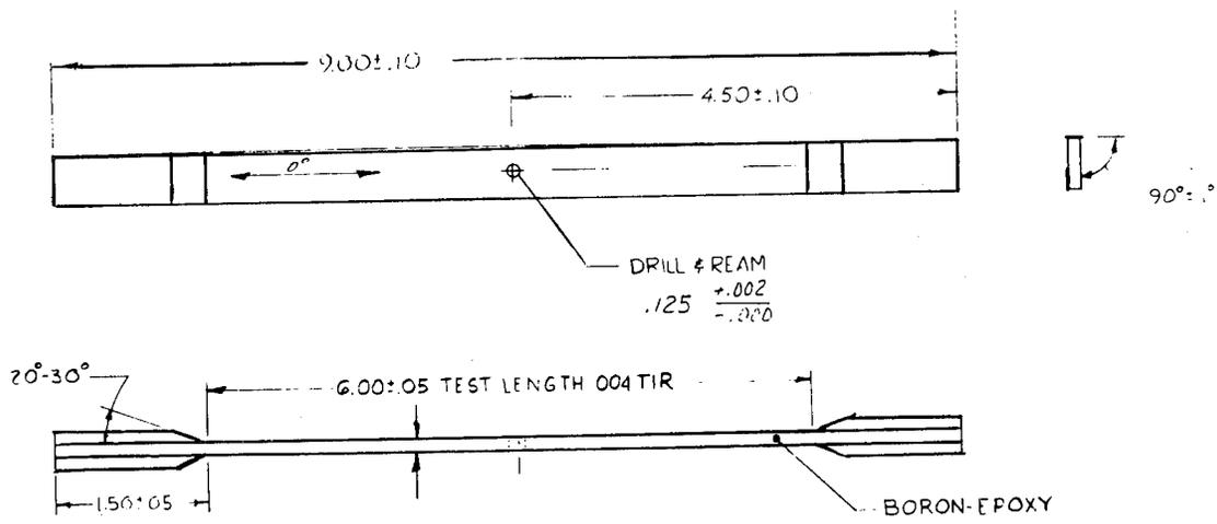
FIGURE 3-23. NOTCHED FATIGUE SPECIMEN<sup>(104)</sup>
