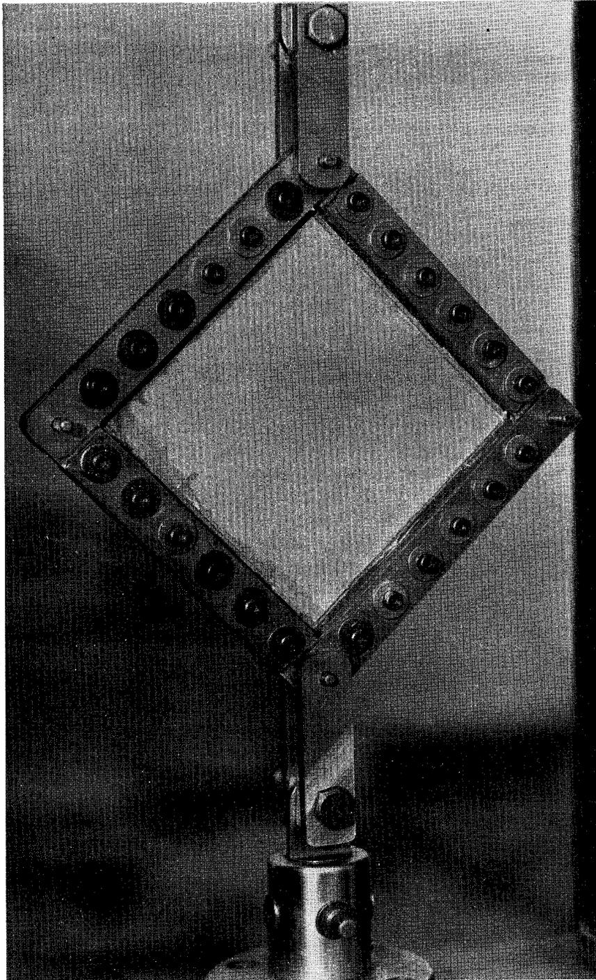
FIGURE 3-11. PICTURE FRAME FIXTURE WITH TEST ASSEMBLY
