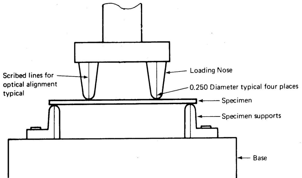
FIGURE 2-15. FLEXURE TEST FIXTURE<sup>(46)</sup>
