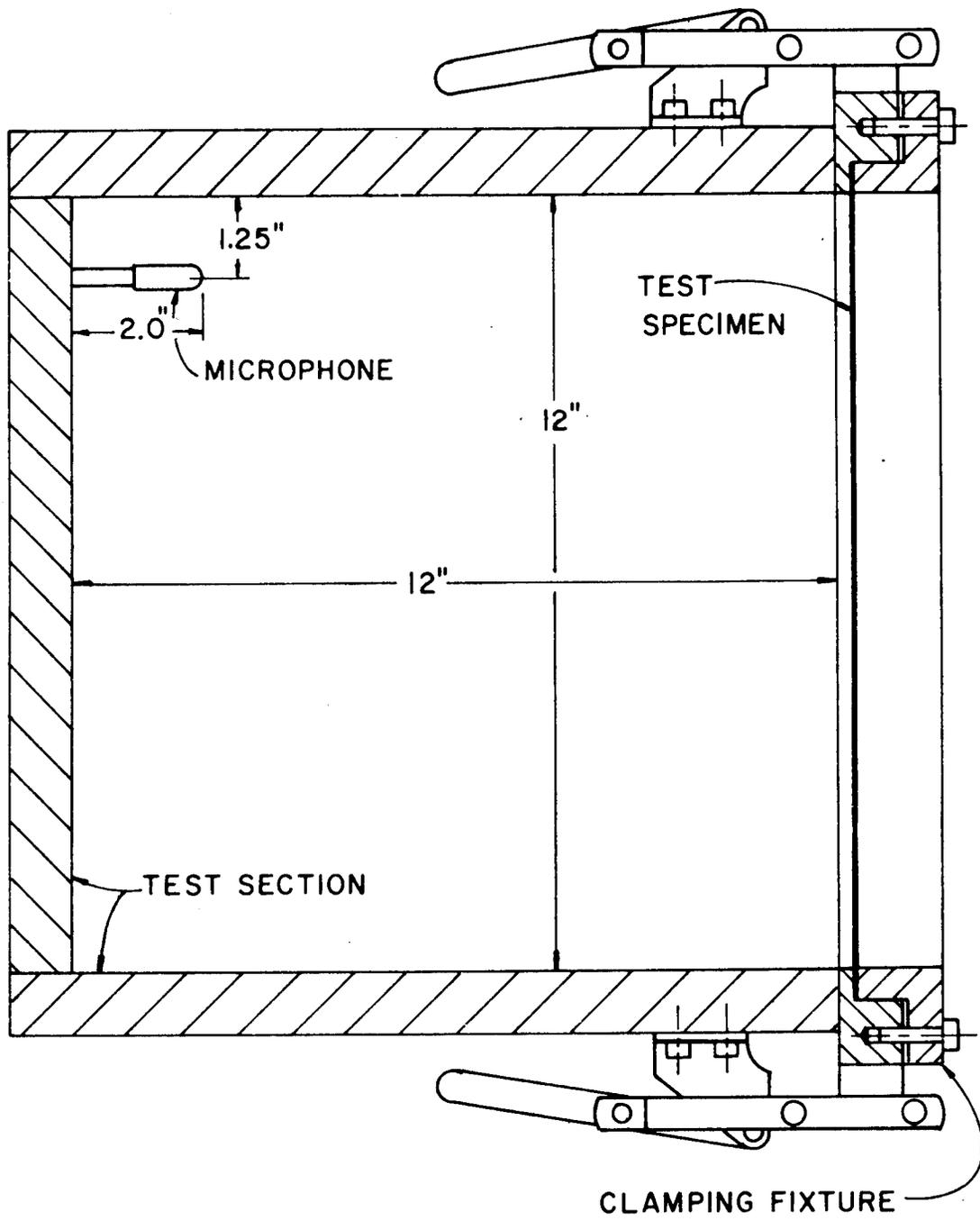
FIGURE 3-45. COMPOSITE PANEL TEST SPECIMEN INSTALLED IN ONE FOOT SQUARE TEST SECTION FOR GRAZING INCIDENCE IMPINGEMENT<sup>(111)</sup>
