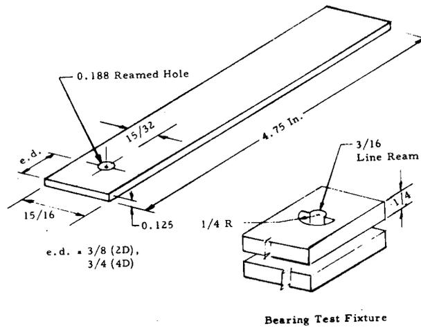
FIGURE 3-18. BEARING TEST SPECIMENS<sup>(44,71,102)</sup>
