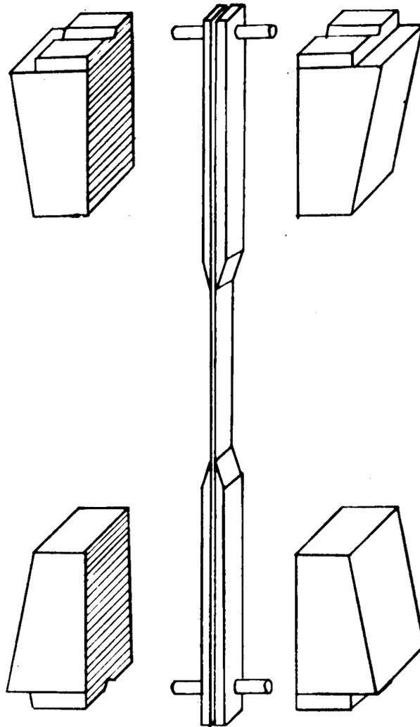
FIGURE 2-27. TEST CONFIGURATION INCLUDING SELF-ALIGNING FIXTURE<sup>(104)</sup>
