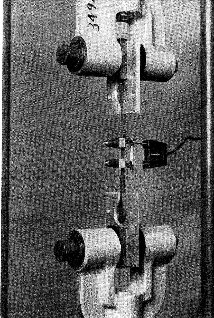
FIGURE 2-5. TOW TENSILE COUPON, WITH ATTACHED STRAIN GAGE EXTENSOMETER, AS MOUNTED IN SPECIALIZED FIXTURES FOR TENSILE TESTING<sup>(27)</sup>
