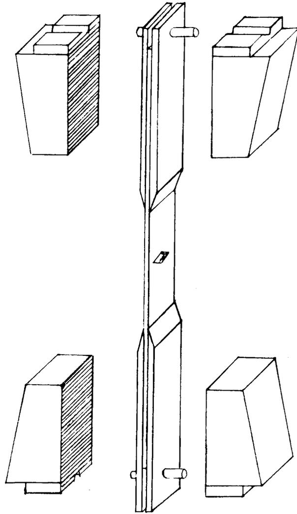
FIGURE 3-41. TEST CONFIGURATION INCLUDING SELF-ALIGNING FIXTURE<sup>(104)</sup>
