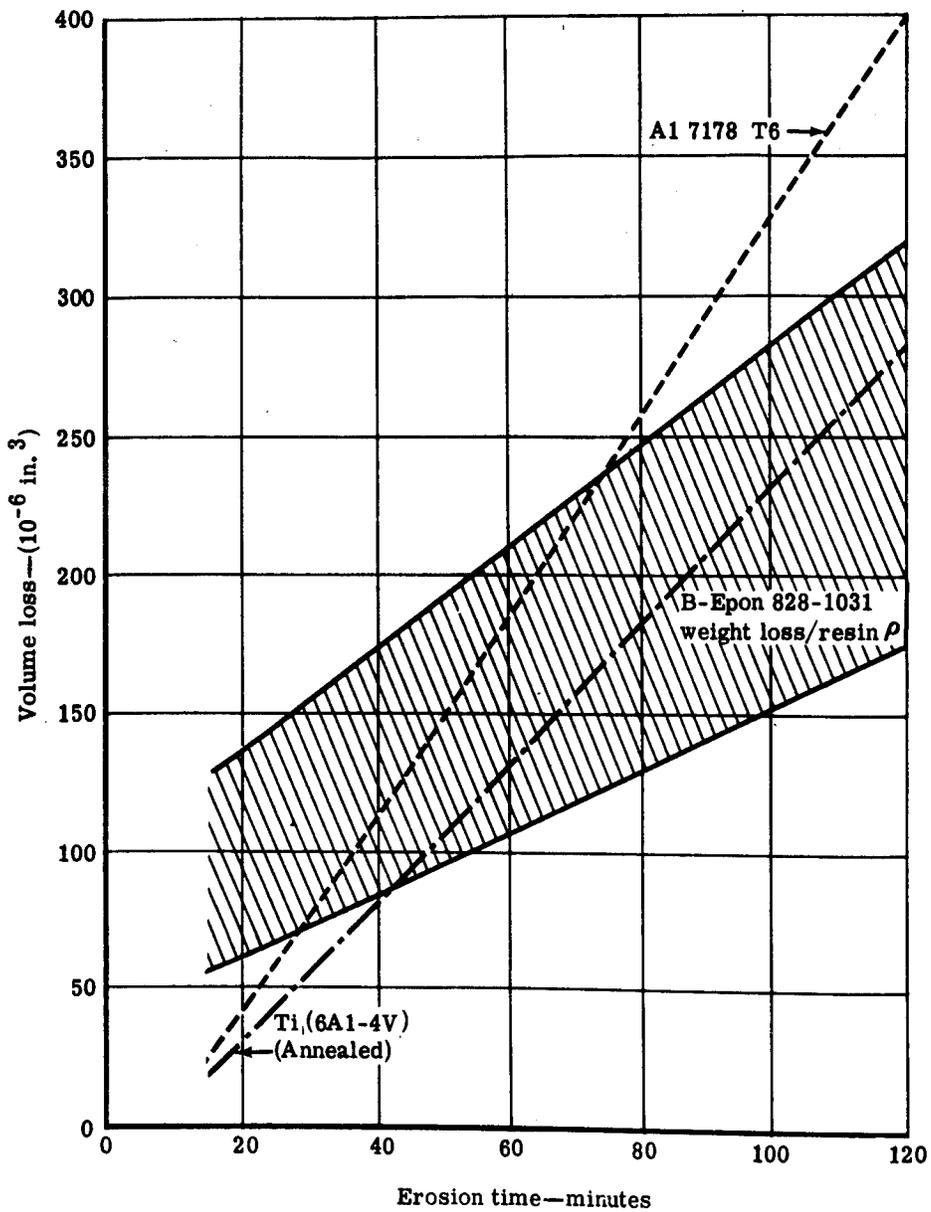
FIGURE 3-43. EROSION RATES FOR Al 7178 T6, Ti 6Al-4V AND B-RESIN COMPOSITE MATERIALS<sup>(47)</sup>
