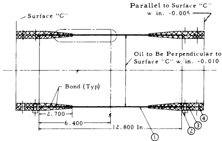
FIGURE 3-4. TUBULAR TYPE AXIAL TENSION SPECIMENS<sup>(81, 82)</sup>
