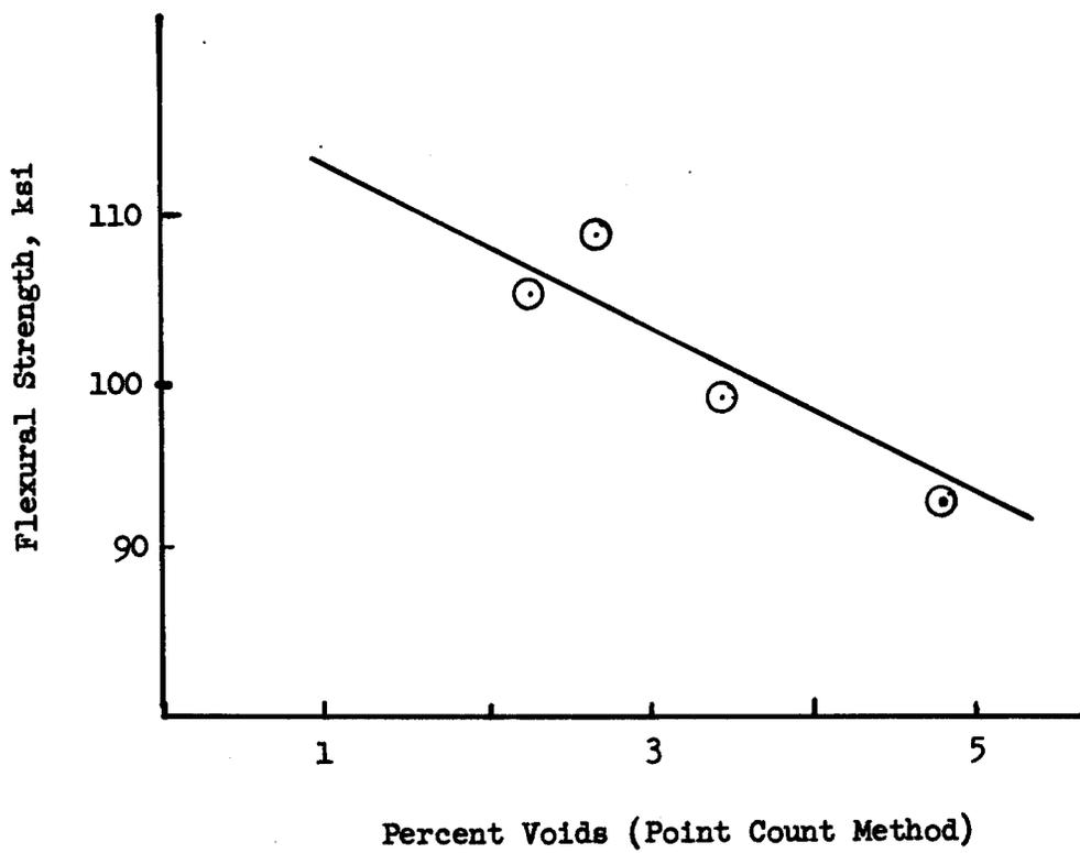
FIGURE 2-17. EFFECT OF VOID CONTENT ON COMPOSITE FLEXURAL STRENGTH<sup>(56)</sup>
