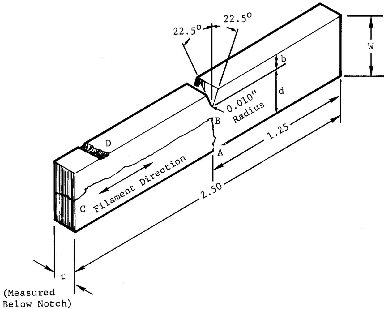
FIGURE 3-17. IZOD IMPACT SPECIMEN CONFIGURATION<sup>(64)</sup>
