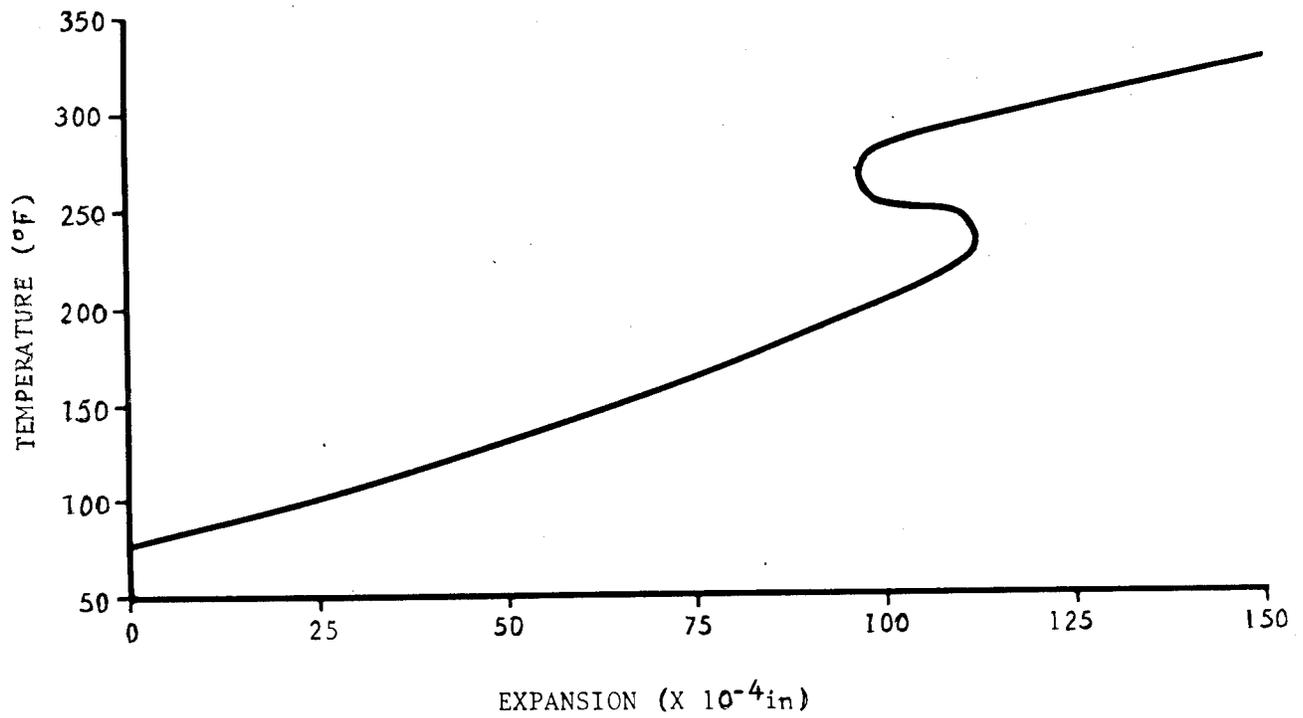
FIGURE 2-18. TYPICAL EXPANSION CURVE OF E-798 CAST RESIN PRIOR TO POSTCURE<sup>(63)</sup>
