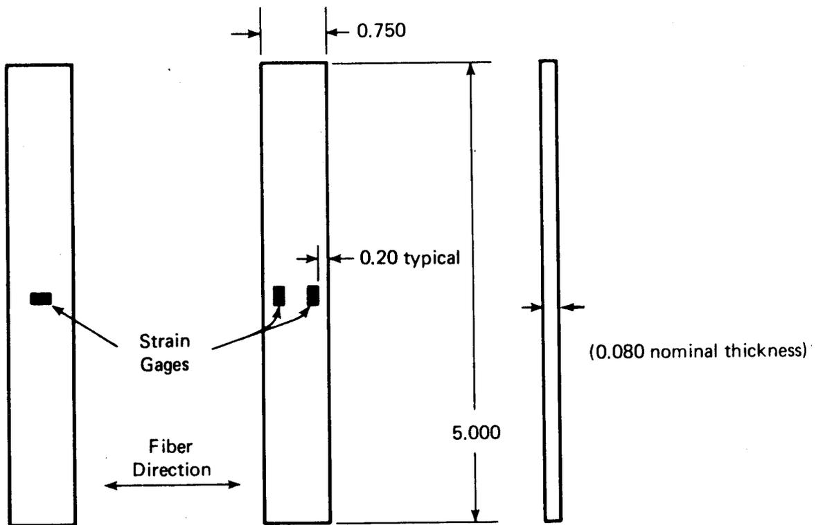
FIGURE 2-29. TRANSVERSE TENSILE TEST SPECIMEN
