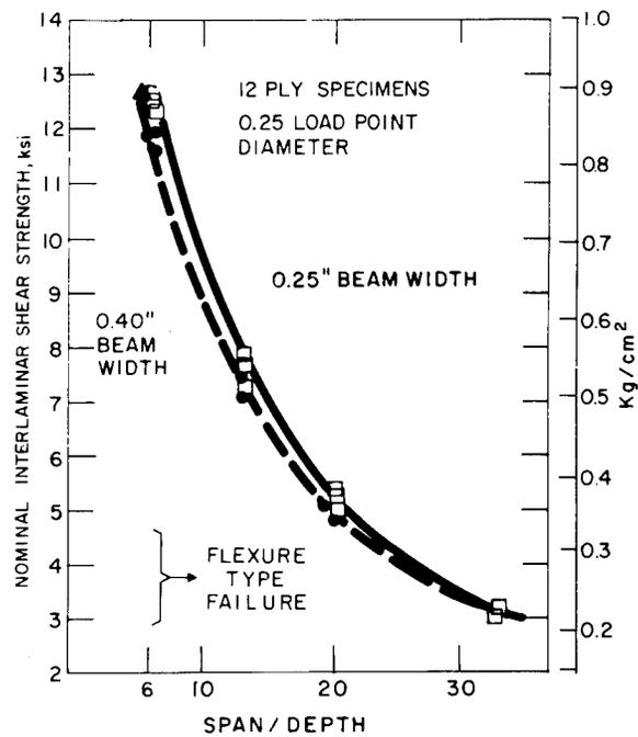
FIGURE 2-40. INFLUENCE OF SPAN TO DEPTH AND BEAM WIDTH ON NOMINAL INTERLAMINAR SHEAR STRENGTH OF UNIDIRECTIONAL BORON EPOXY<sup>(65)</sup>
