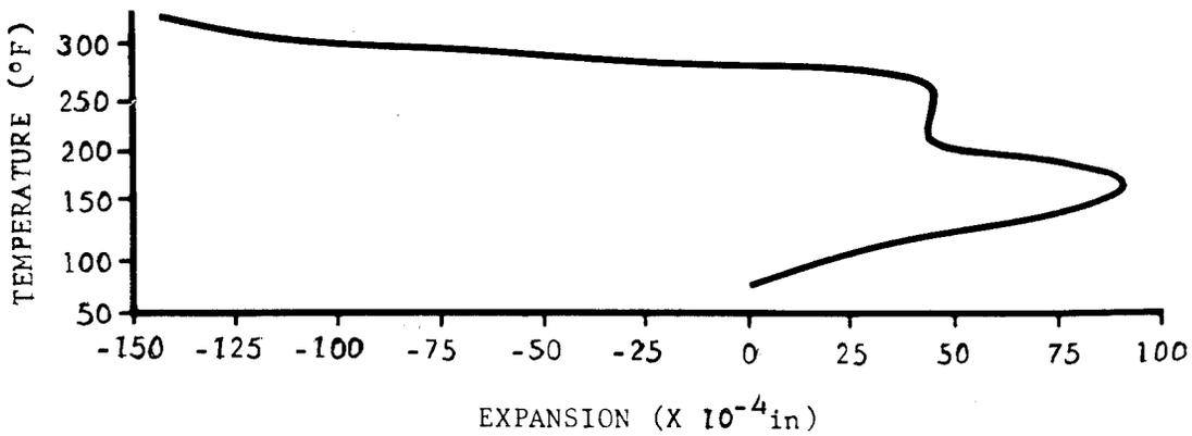
FIGURE 2-19. TYPICAL EXPANSION CURVE OF TRANSVERSE SPECIMEN OF THORNEL 50/E-798 EPOXY LAMINATE PRIOR TO POSTCURE<sup>(63)</sup>
