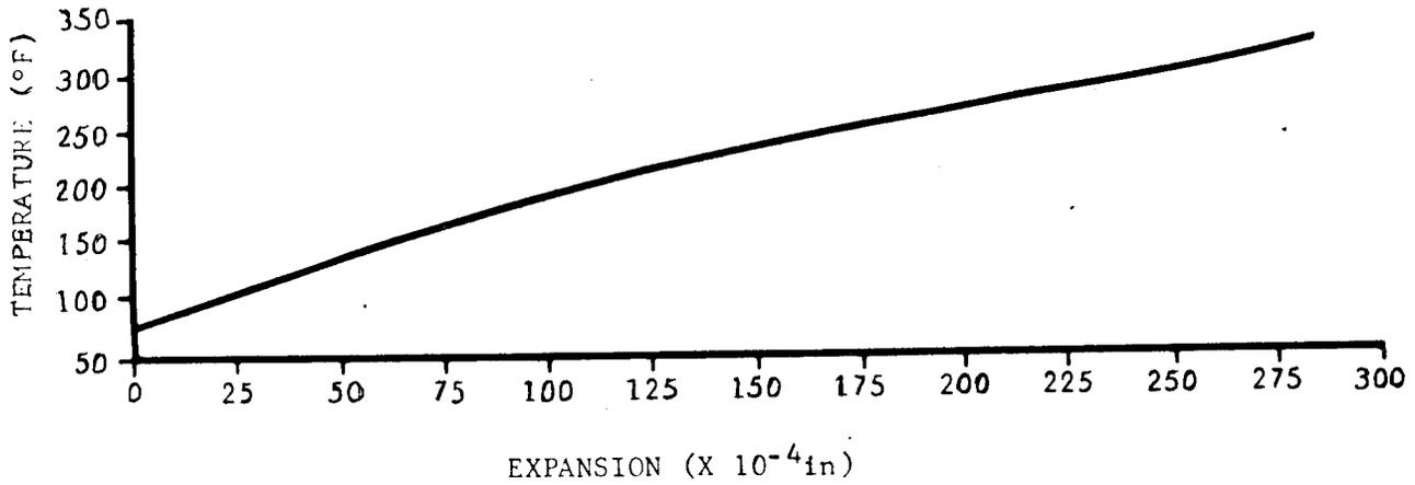
FIGURE 2-20. TYPICAL EXPANSION CURVE OF E-798 CAST RESIN AFTER POSTCURE<sup>(63)</sup>
