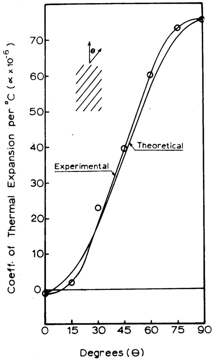
FIGURE 2-23. ANGULAR VARIATION OF THERMAL EXPANSION COEFFICIENTS FOR UNIDIRECTIONAL GRAPHITE-EPOXY COMPOSITES<sup>(1)</sup>
