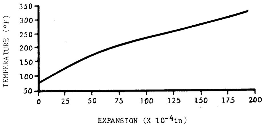
FIGURE 2-21. TYPICAL EXPANSION CURVE OF TRANSVERSE SPECIMEN OF THORNEL 50/E-798 EPOXY LAMINATE AFTER POSTCURE<sup>(63)</sup>
