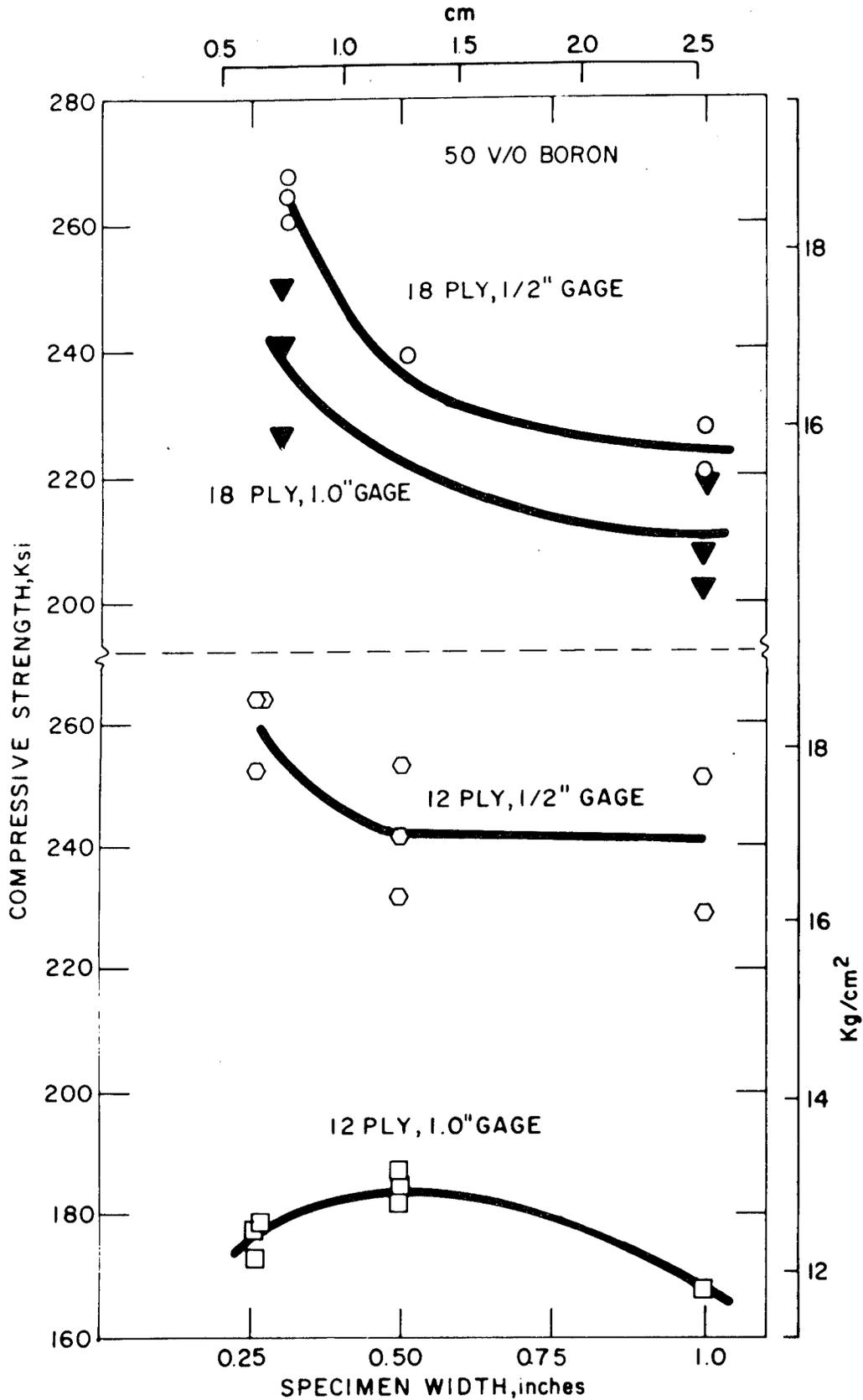
FIGURE 2-34. INFLUENCE OF SPECIMEN WIDTH, LENGTH, AND NUMBER OF PLYS ON COMPRESSIVE STRENGTH OF UNIDIRECTIONAL BORON EPOXY<sup>(65)</sup>
