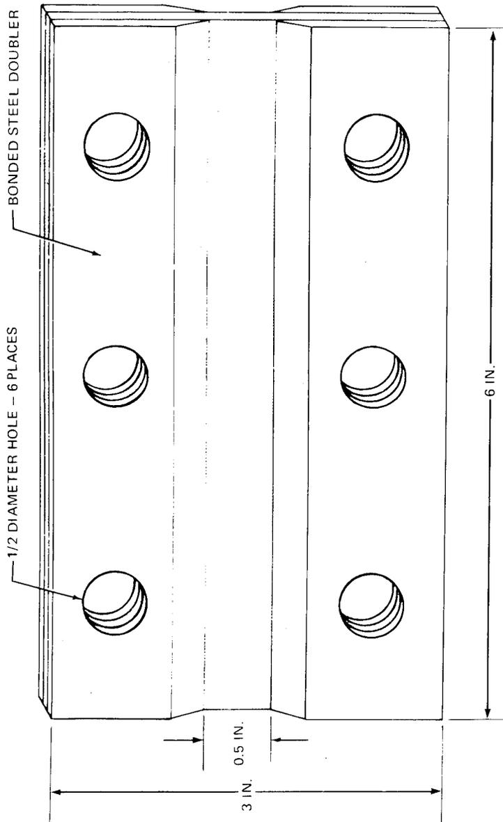
FIGURE 3-14. MODIFIED RAIL SHEAR SPECIMEN WITH BONDED DOUBLERS (79)
