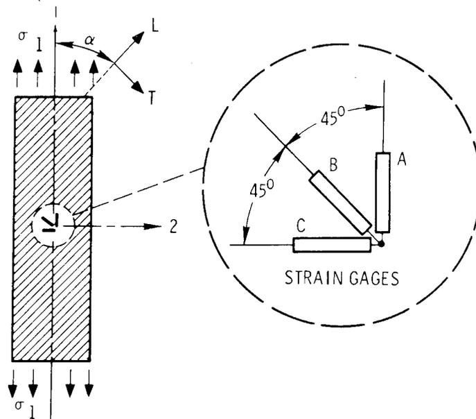
FIGURE 3-15. SHEAR MODULUS SHEAR SPECIMEN TENSILE COUPON WITH ORIENTED FIBERS<sup>(100)</sup>
