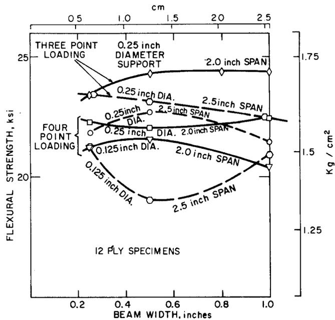
FIGURE 2-37. INFLUENCE OF BEAM WIDTH, LOAD SUPPORT DIAMETER, SPAN, AND LOADING MODE ON TRANSVERSE FLEXURAL STRENGTH OF UNIDIRECTIONAL BORON EPOXY<sup>(65)</sup>
