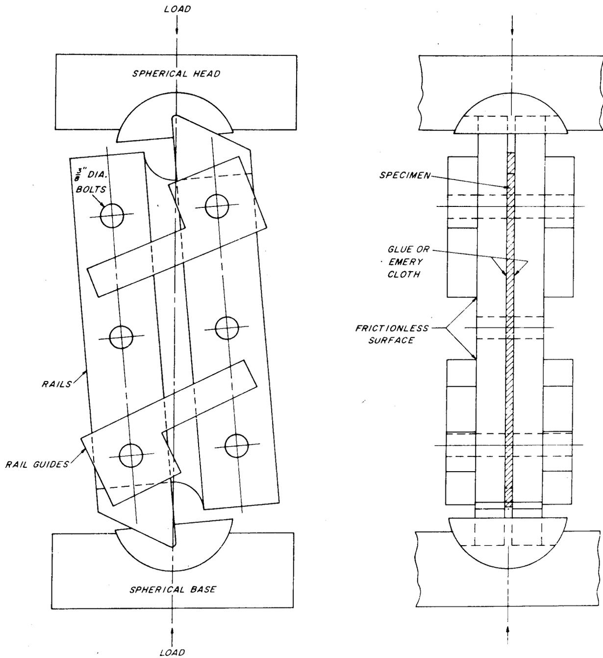
FIGURE 3-12. RAIL SHEAR TEST APPARATUS<sup>(96)</sup>
