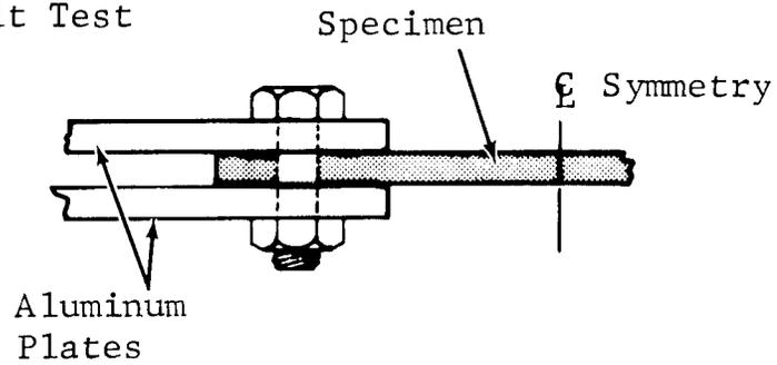
Countersunk Bolt Test
