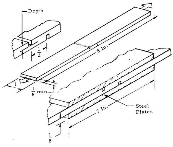
FIGURE 2-38. THREE TYPES OF COMPOSITE NOTCH-SHEAR SPECIMENS (68, 70, 72, 73)
