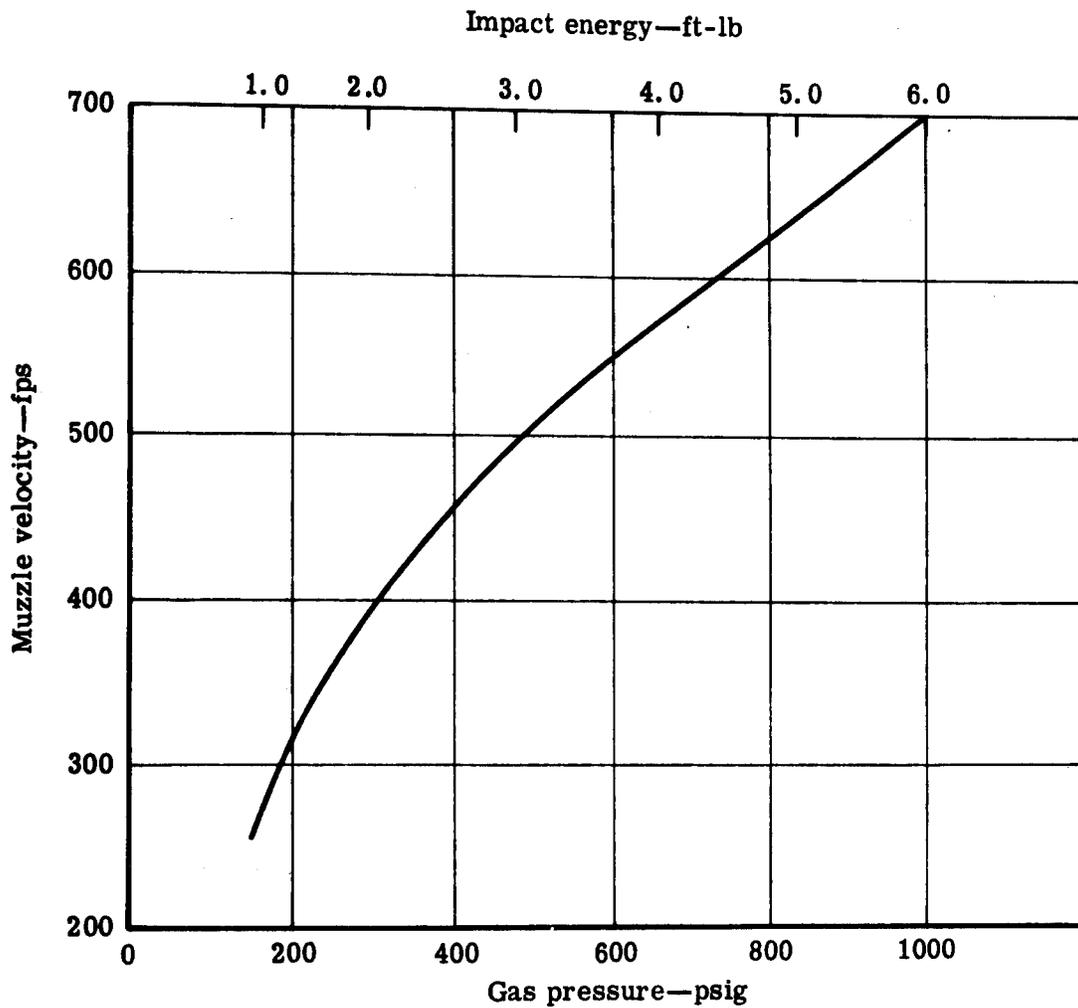
FIGURE 3-49. CALIBRATION CURVE FOR BALLISTIC IMPACT RIG. CROSSMAN 160 PELLGUN, 0.36 GRAM SPHERICAL STEEL BALL<sup>(46)</sup>
