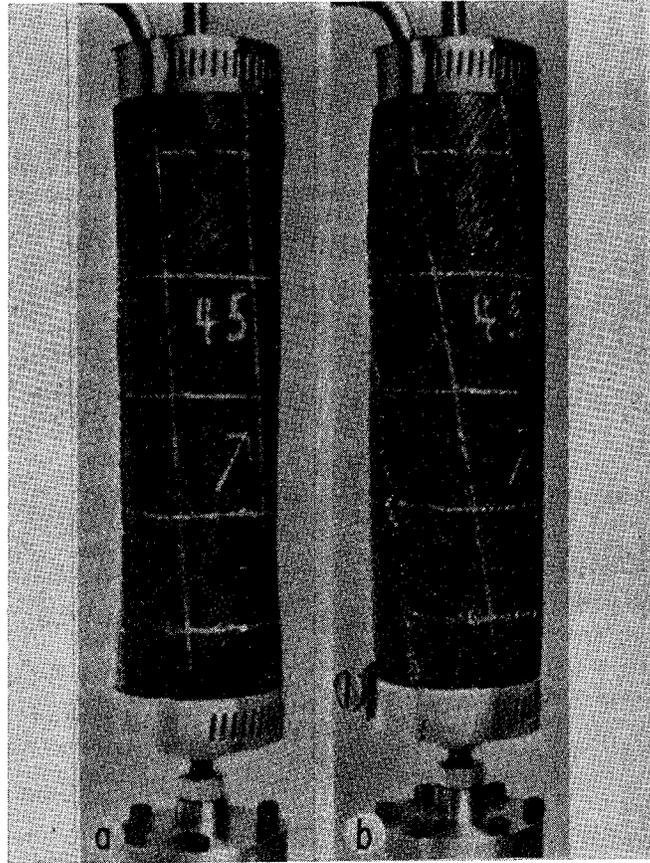
FIGURE 3-7. HELICAL WOUND THIN-WALLED TUBE UNDER (A) UNIFORM TENSION AND (B) INTERNAL PRESSURE<sup>(85)</sup>
