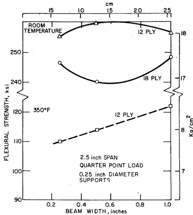
FIGURE 2-36. INFLUENCE OF BEAM WIDTH, NUMBER OF PLYS, AND TEST TEMPERATURE ON FLEXURAL STRENGTH (2.5-IN. SPAN) OF UNIDIRECTIONAL BORON EPOXY<sup>(65)</sup>
