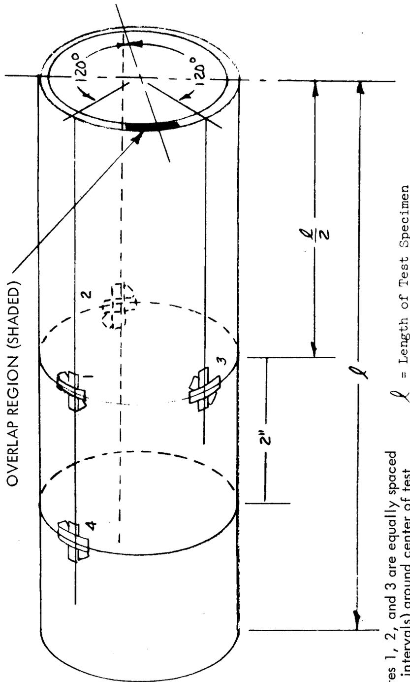
Note: Rosettes 1, 2, and 3 are equally spaced ( $120^\circ$  intervals) around center of test section; rosette 2 is approximately  $180^\circ$  from overlap region. Rosette 4 is spaced on a section 2 inches (or other specified distance) from the center section.
