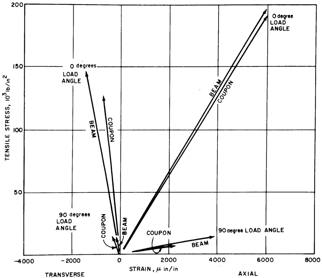
FIGURE 3-2. TYPICAL STRESS-STRAIN RESPONSE 0-DEGREE LAMINATES BORON/SP272 6-PLY COMPARISONS OF BEAM AND COUPON TESTS
