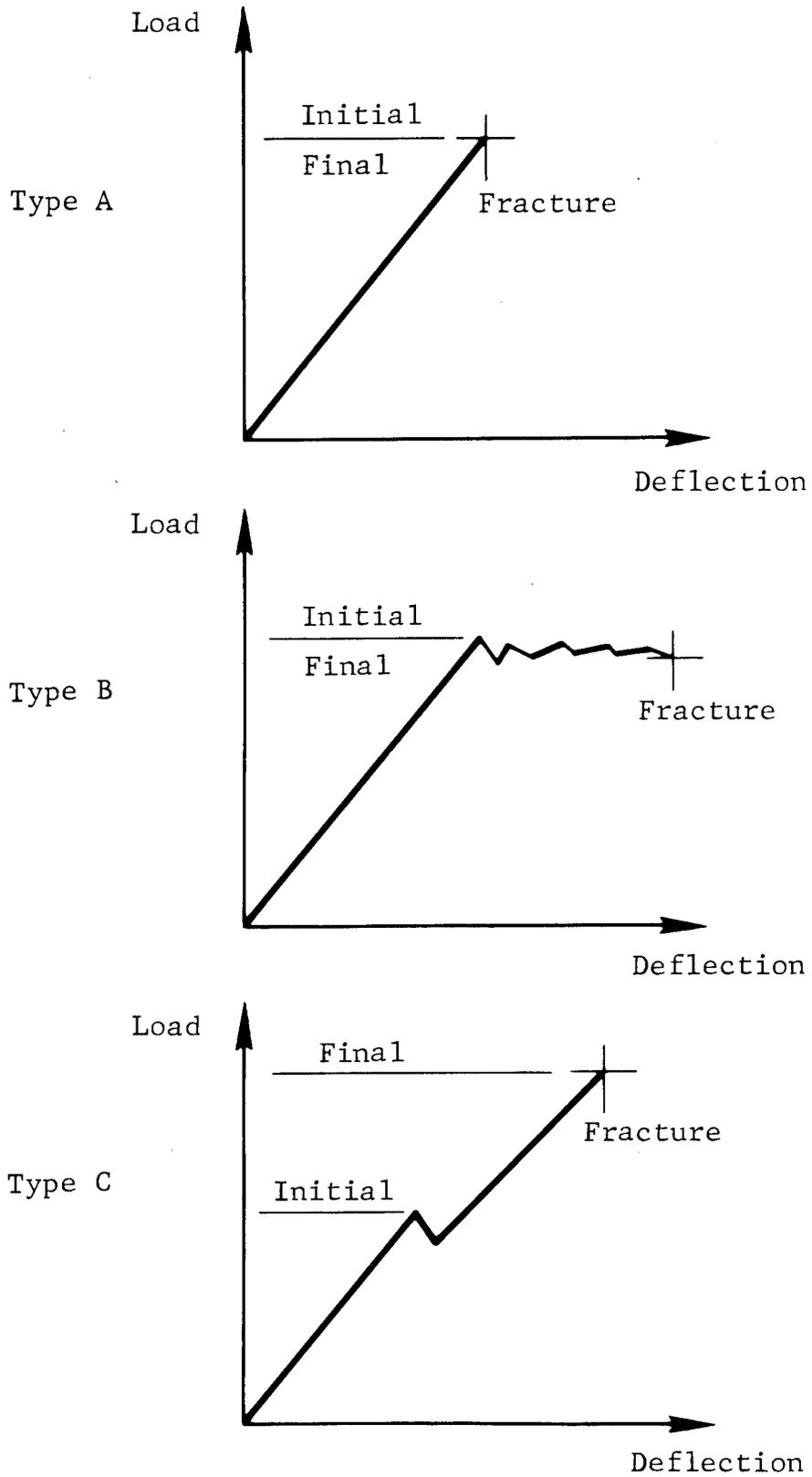
FIGURE 3-20. LOAD/DEFLECTION BEHAVIOR OF BORON/EPOXY BEARING SPECIMENS<sup>(103)</sup>
