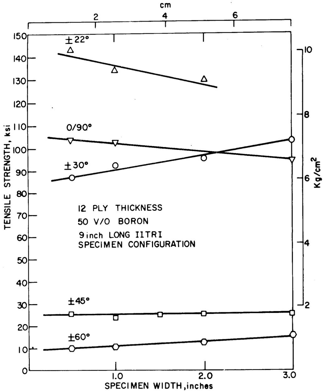
FIGURE 2-32. INFLUENCE OF SPECIMEN WIDTH ON TENSILE STRENGTH OF CROSS-PLY AND ANGLE-PLY BORON EPOXY<sup>(65)</sup>
