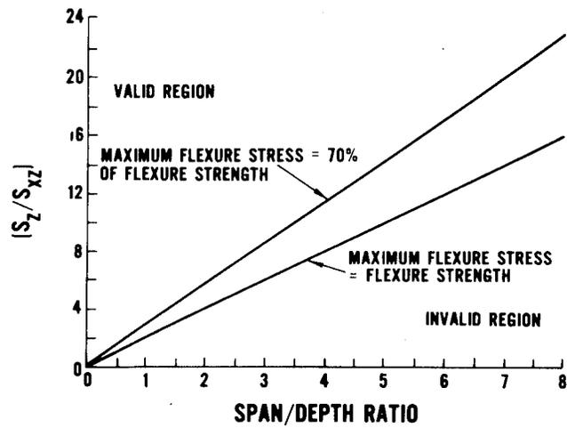
FIGURE 2-41. RATIO OF FLEXURAL STRENGTH-TO-SHEAR STRENGTH VERSUS SPAN-TO-DEPTH RATIO<sup>(74)</sup>
