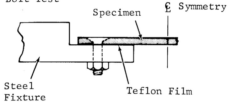
FIGURE 3-19. BOLT BEARING SPECIMENS AND TEST APPARATUS<sup>(103)</sup>
