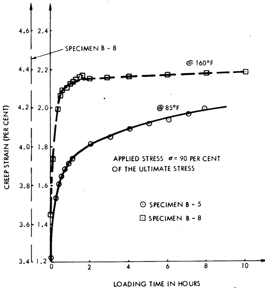
FIGURE 3-33. THE EFFECT OF TEMPERATURE ON THE CREEP STRAIN OF (30 DEG -60 DEG) LAMINATES STRESSED AT 90 PERCENT OF ITS ULTIMATE<sup>(106)</sup>
