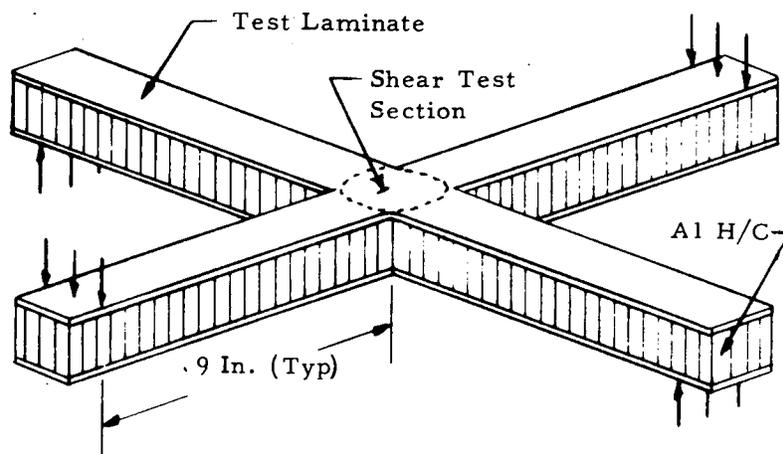
FIGURE 3-16. SHEAR LOADING OF CROSSBEAM SPECIMEN<sup>(83,84)</sup>
