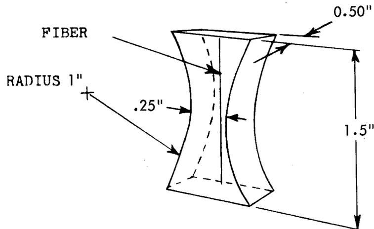
FIGURE 3-39. SINGLE FIBER TEST SPECIMEN, RADIAL TENSILE STRENGTH DETERMINATION<sup>(56)</sup>
