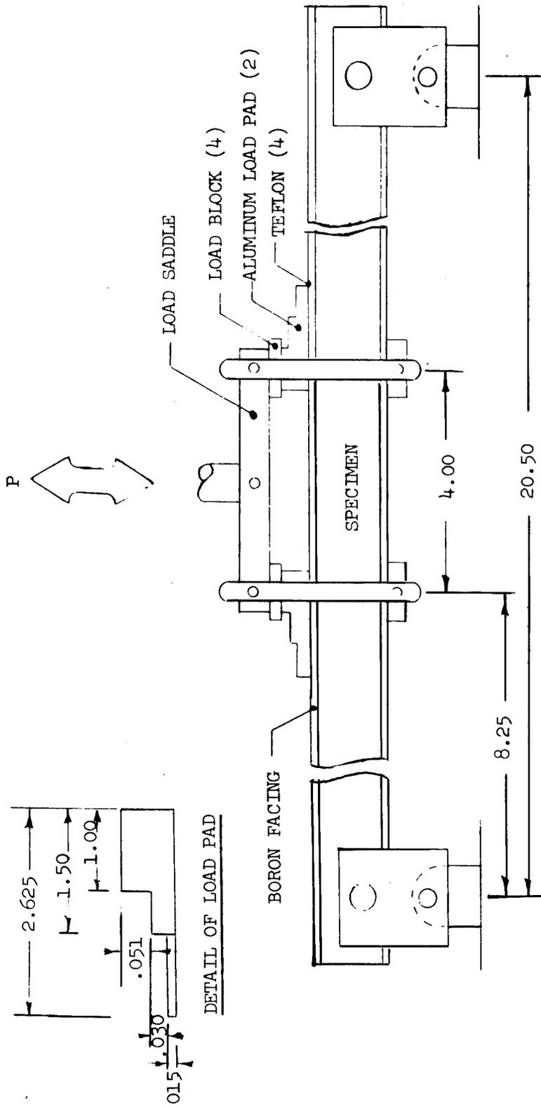
FIGURE 3-26. LOADING AND SUPPORT FOR BEAM SPECIMEN<sup>(104)</sup>
