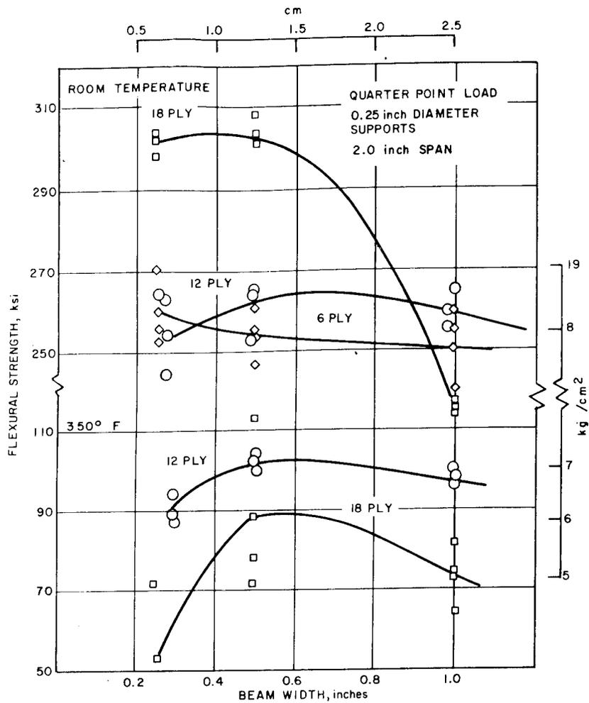
FIGURE 2-35. INFLUENCE OF BEAM WIDTH, NUMBER OF PLYS, AND TEST TEMPERATURE ON FLEXURAL STRENGTH (2.0-IN. SPAN) OF UNIDIRECTIONAL BORON EPOXY<sup>(65)</sup>
