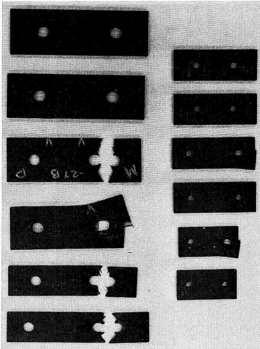
FIGURE 3-22. GRAPHITE/EPOXY BOLT BEARING SPECIMENS<sup>(103)</sup>
