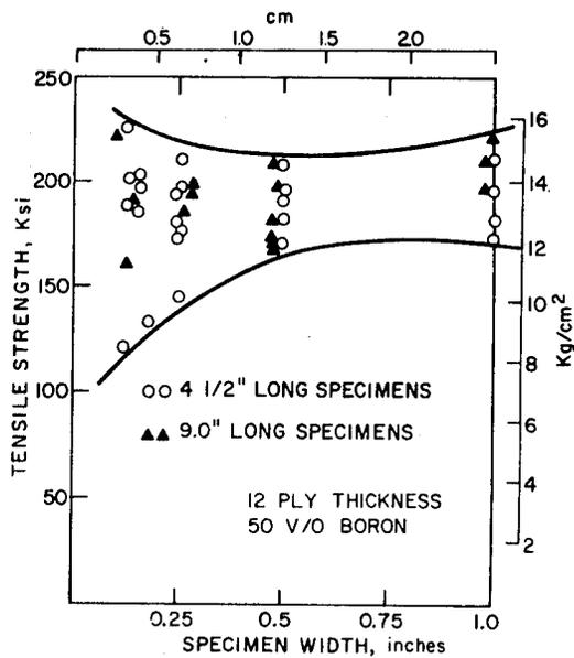
FIGURE 2-30. INFLUENCE OF SPECIMEN WIDTH AND LENGTH ON TENSILE STRENGTH OF UNIDIRECTIONAL BORON EPOXY<sup>(65)</sup>
