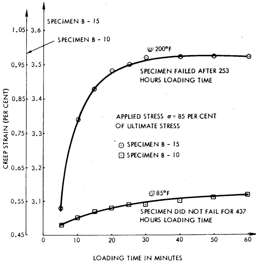
FIGURE 3-34. THE EFFECT OF TEMPERATURE ON THE CREEP STRAIN OF (30 DEG -60 DEG) LAMINATES STRESSED AT 85 PERCENT OF ITS ULTIMATE<sup>(106)</sup>
