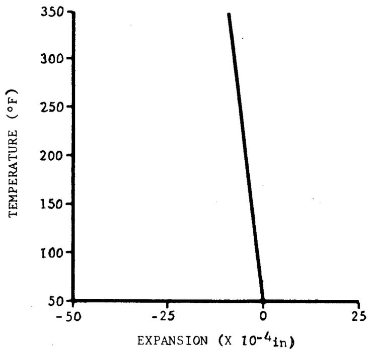
FIGURE 2-22. EXPANSION CURVE OF LONGITUDINAL SPECIMEN OF THORNEL 50/E-798 EPOXY LAMINATE
