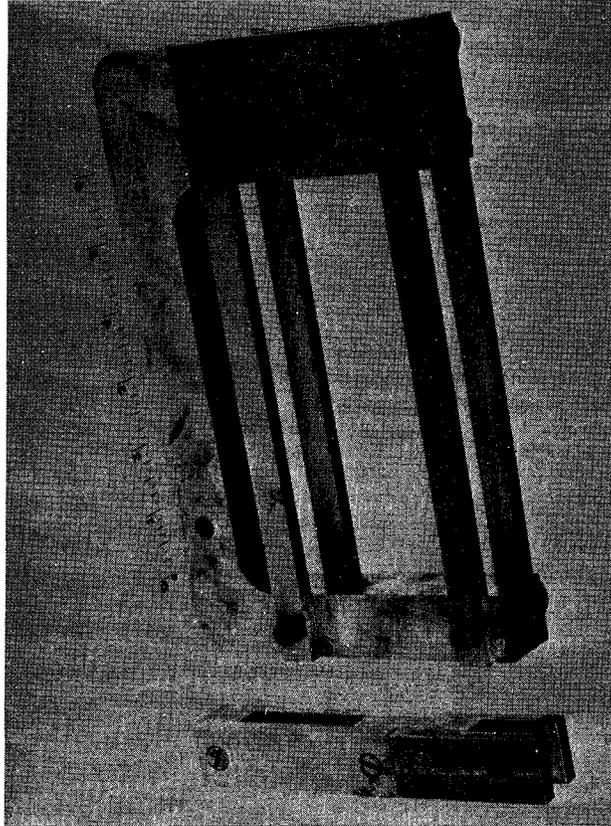
FIGURE 3-38. CRACK PROPAGATION TEST FIXTURE<sup>(56)</sup>
