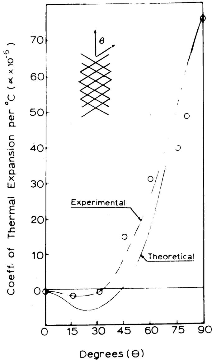
FIGURE 2-24. THERMAL EXPANSION COEFFICIENTS OF ANGLE-PLY GRAPHITE-EPOXY COMPOSITES AS A FUNCTION OF PLY ANGLE<sup>(1)</sup>
