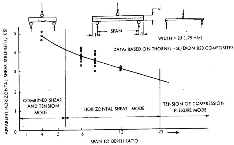
FIGURE 2-39. GENERAL CHARACTERISTICS OF INTERLAMINAR TEST FOR GRAPHITE/EPOXY COMPOSITES<sup>(66)</sup>
