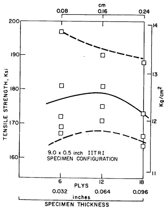
FIGURE 2-31. INFLUENCE OF PLY THICKNESS ON TENSILE STRENGTH OF UNIDIRECTIONAL BORON EPOXY<sup>(65)</sup>
