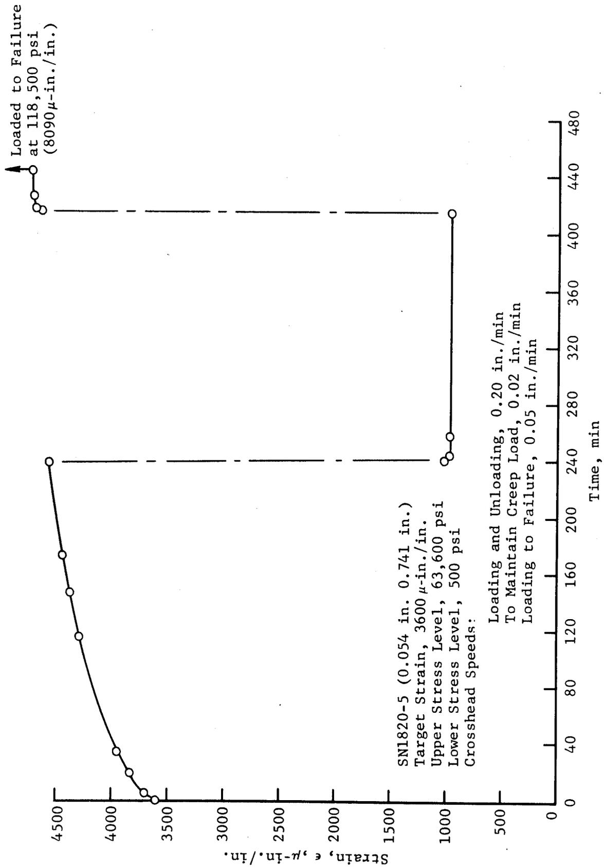
FIGURE 3-32. CREEP TEST, 0°/±45° ORIENTATION AT 270°F
