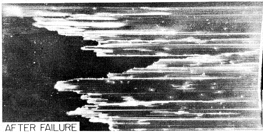
Figure 34e. Typical Sequence of Photographs of Tensile Failure Specimen Showing Distribution of Fiber Breaks Prior to Failure (Specimen A-7)
