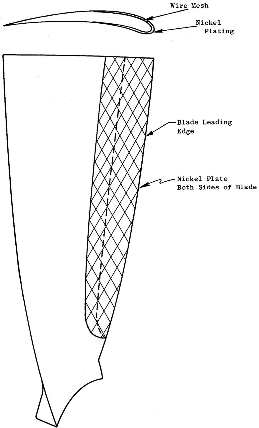
Figure 4. Nickel-Plated Areas on TF39 Polymeric Composite Blades.
