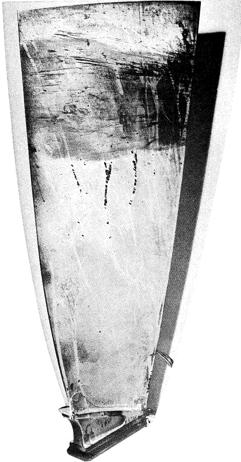
Figure 43. Titanium Blade after Impact
