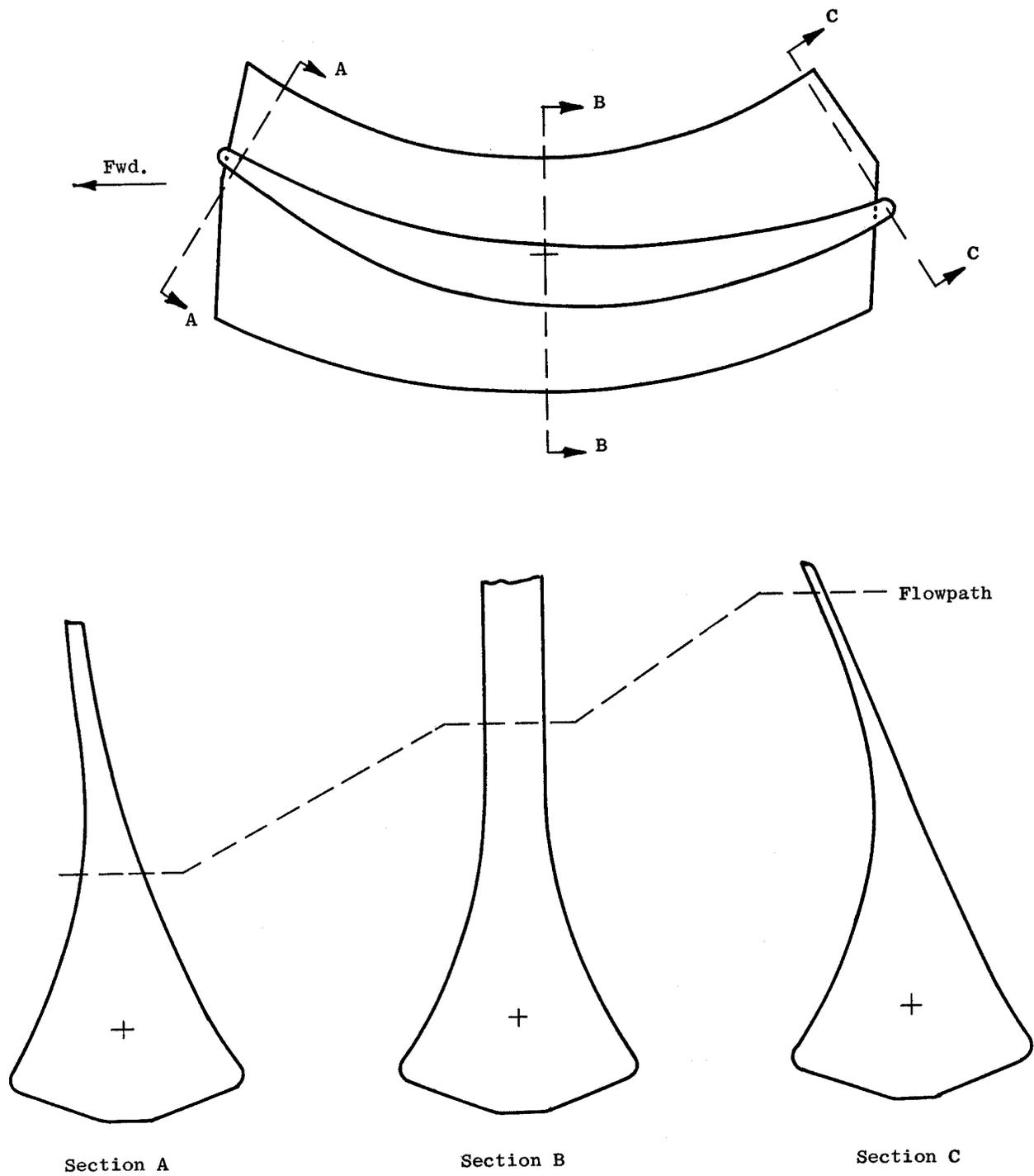
Figure 3. Composite Fan Blade Dovetail.
