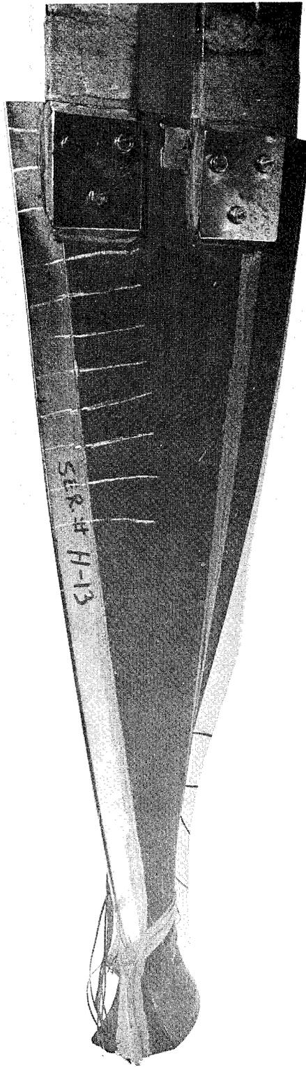
**Figure 38.** NG5 Graphite/Epoxy Blade
