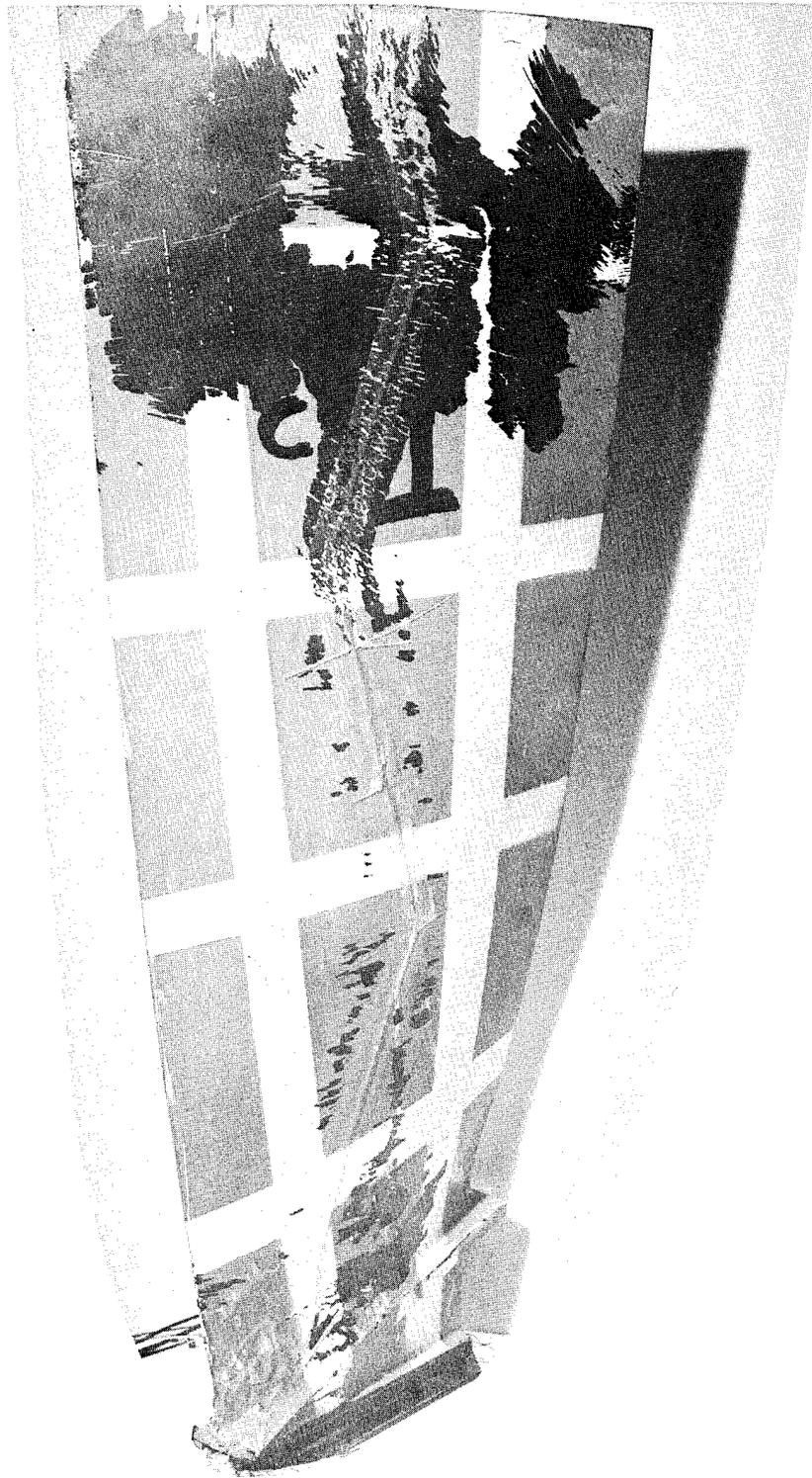
Figure 42. Titanium Blade after Impact
