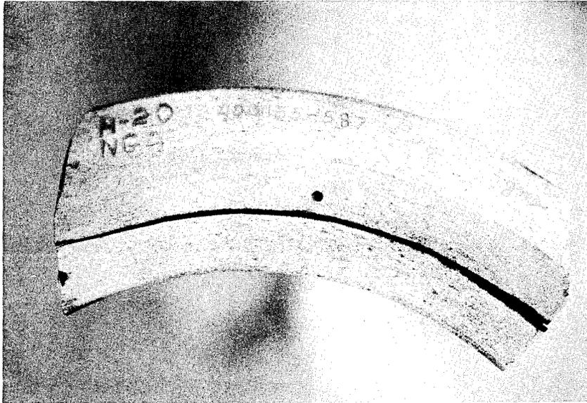
Figure 37. Dye Penetrant Inspection of Dovetail
