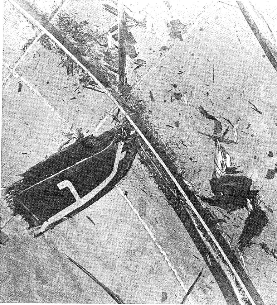
NASA-FOD Impact Resistance Test
