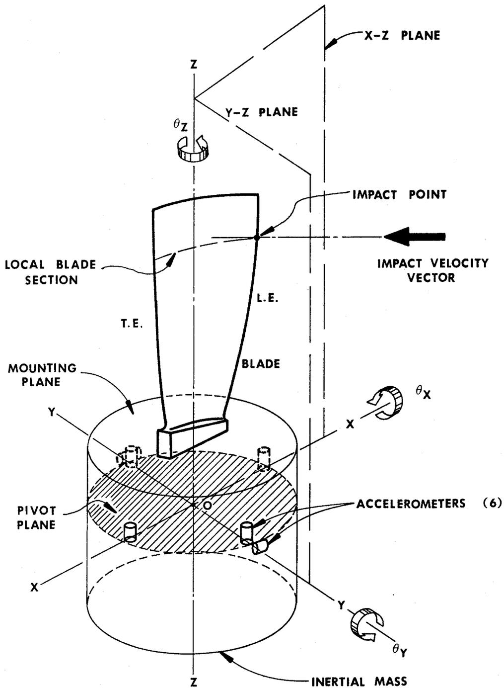
Figure 18. Instrumentation Coordinate System.
