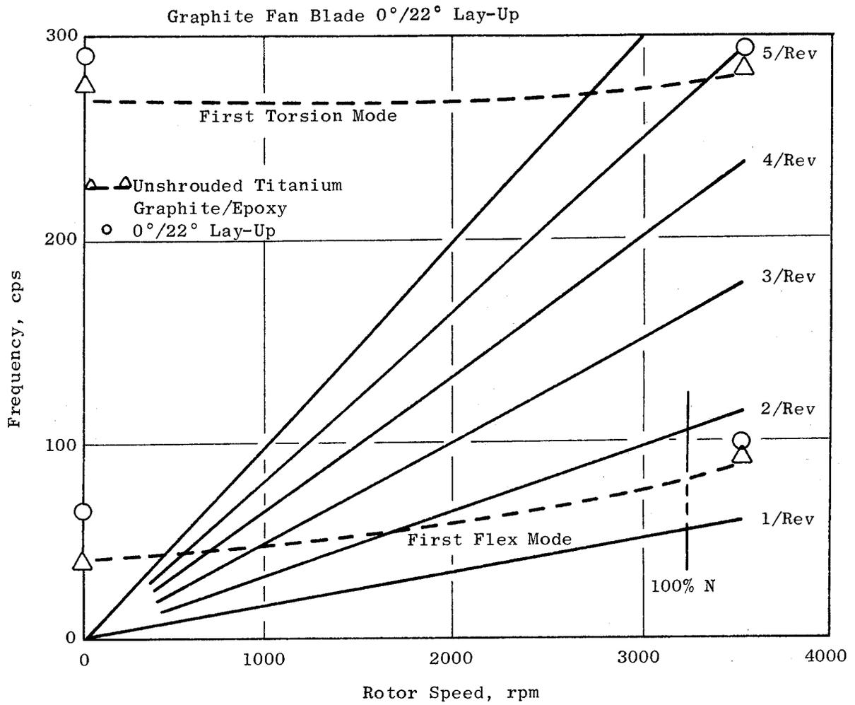
Figure 1. Frequency Characteristics of TF39 Phase II Design Blade.
