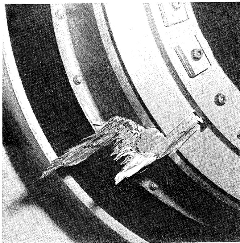
NASA-FOD Impact Resistance Test
