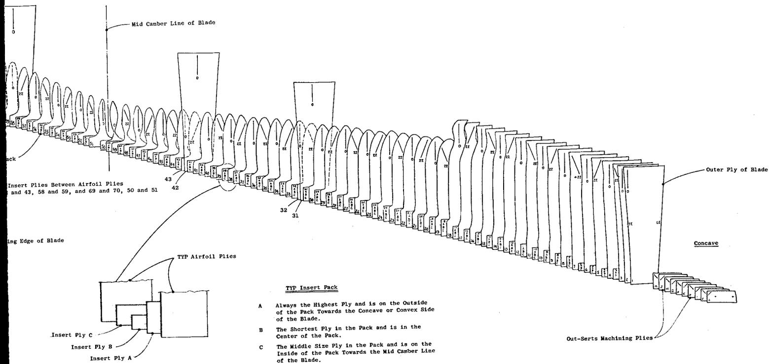
Laminate Ply Configuration for TF39IIB Blade.
