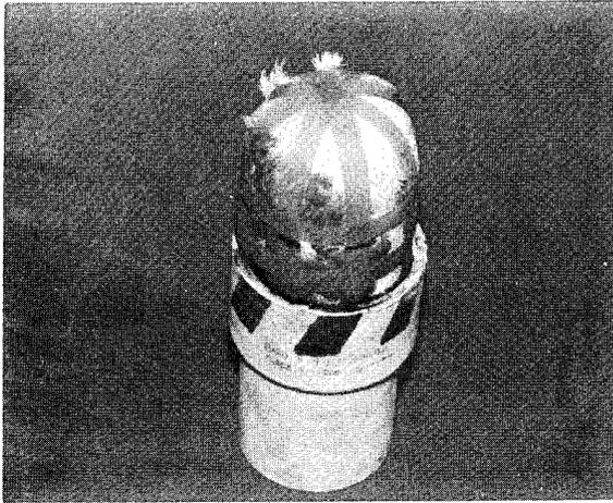
Typical Real Pigeon as Used in NASA-FOD Tests. Pigeon Weight 454 g (16 oz). Held in Carrier by Glass Straps and Cement.
