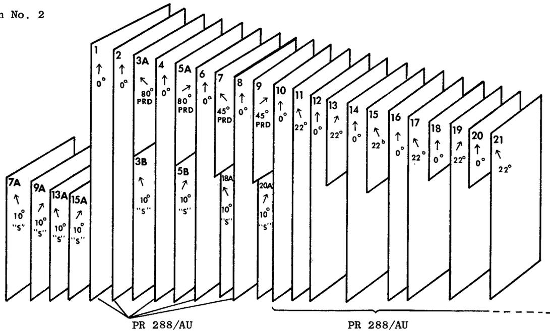
Figure 53. Manufacturing Layup of Selected Design Whiriligig Test Blades.
