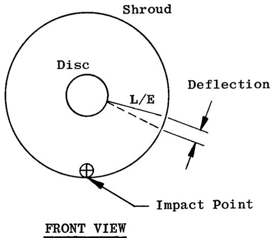
Front and side views show position of blade leading edge before and after impact typical for 5 and 3 o'clock positions.
