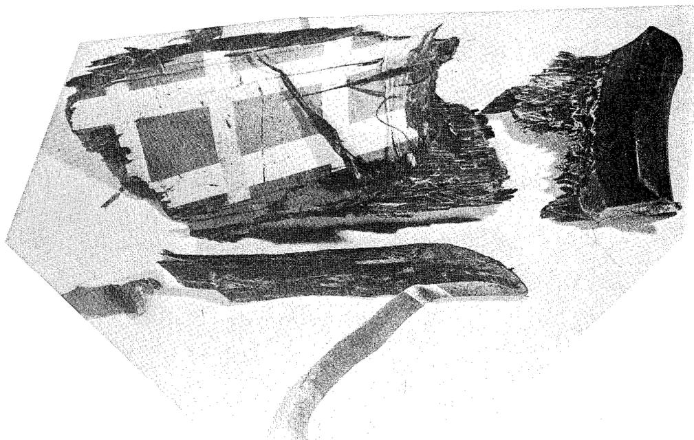
Figure 29. Blade S/N NB4 after Impact
