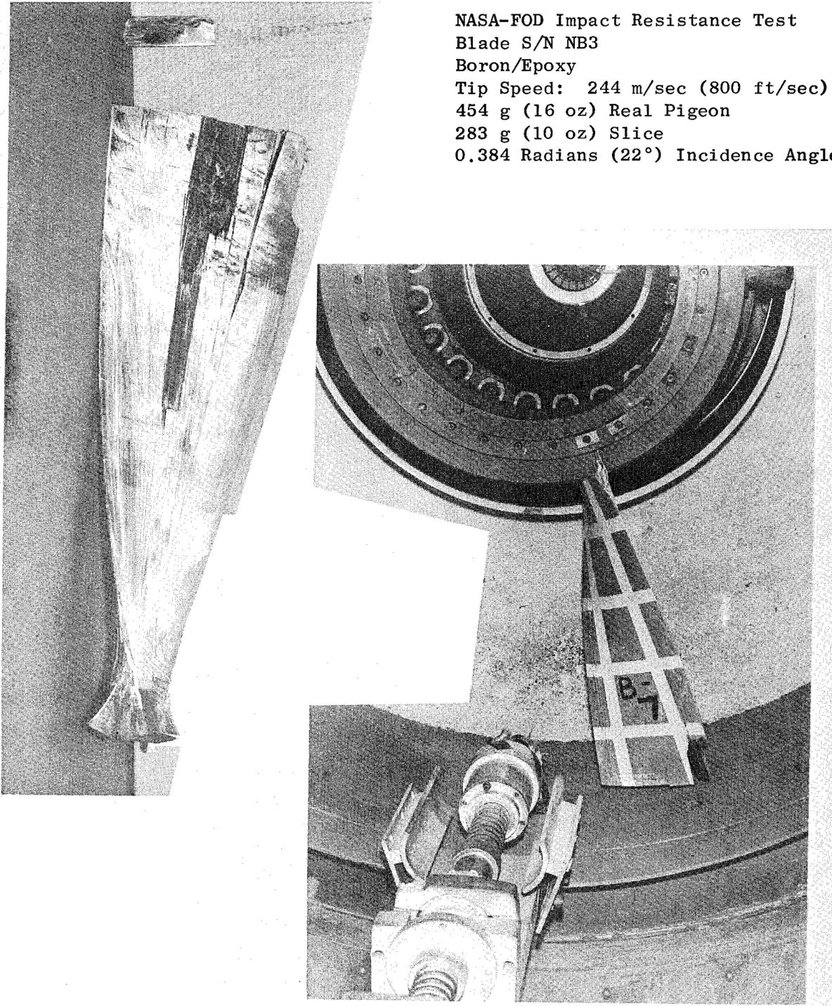
Figure 26. Blade S/N NB3 after Impact.
