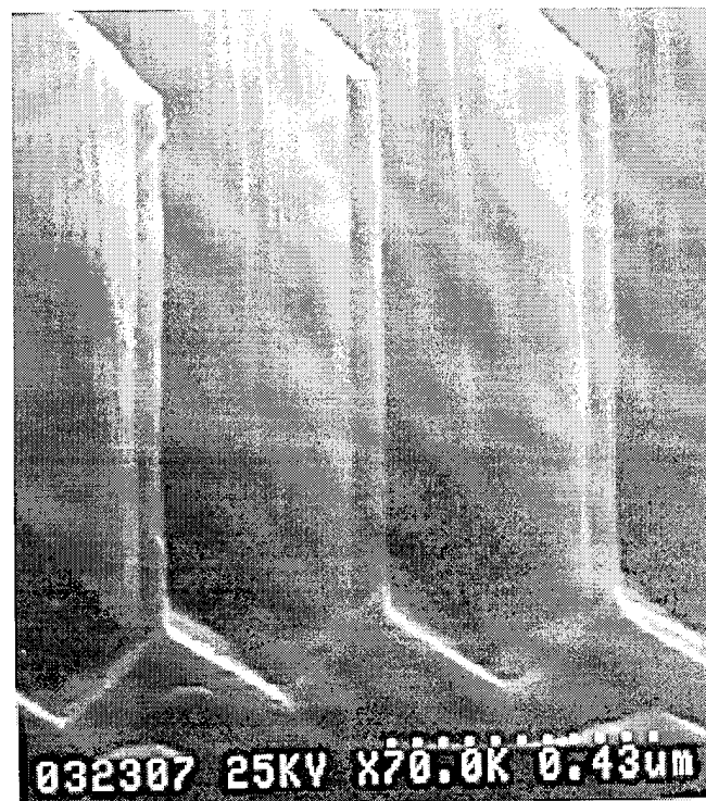
Fig. 3 SEM picture of a 0.36- \mu\text{m} period, 50-nm linewidth (110) Si structures fabricated by KOH etching.
