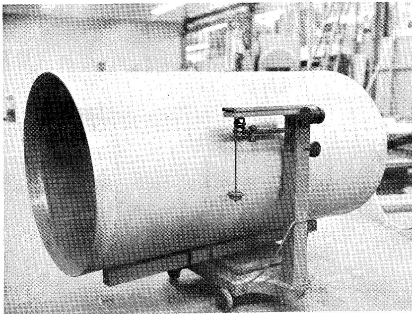
**Fig. 31 Tank Test Section, 2219 Aluminum Shell, P/N 1269331**
