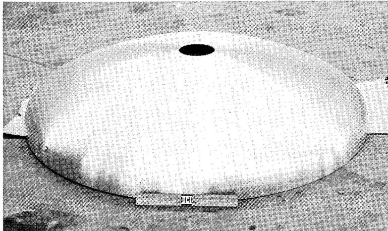
**Fig. 33 Bottom End Closure Assembly 6061 Aluminum Head**
