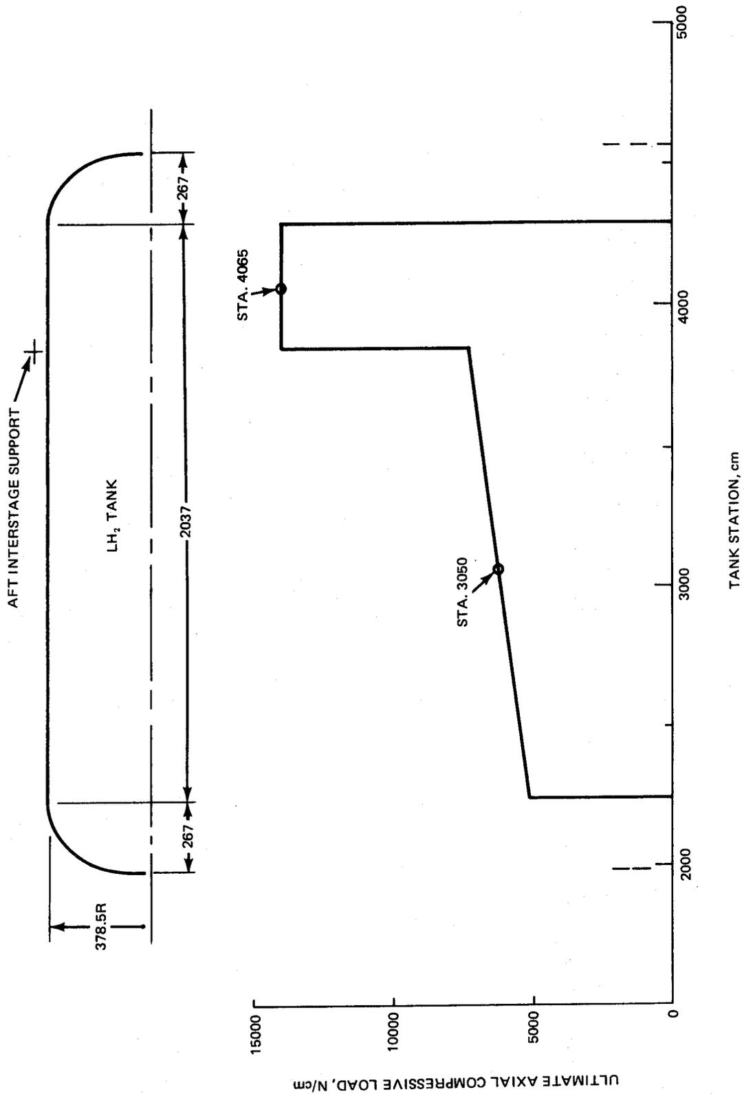
Fig. 3 LH<sub>2</sub> Tank Ultimate Load Intensity at End Boost
