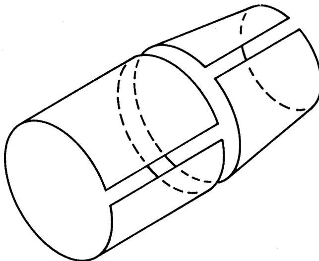
**Fig. 61 Developable Surfaces Premachined in Flat for Concept 1, Orbiter LO<sub>2</sub> Tank**
