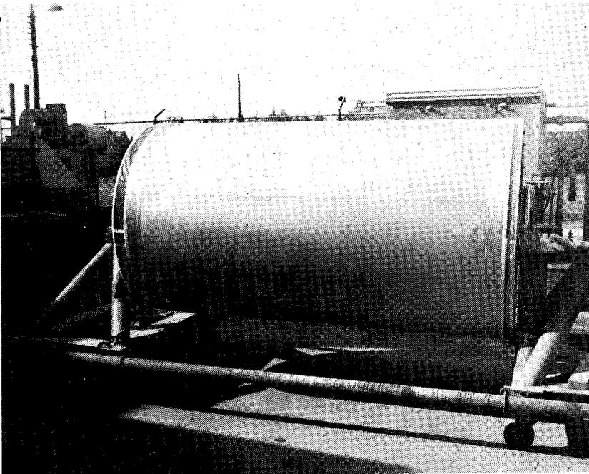
**Fig. 38 Aluminum Shell Assembled to Mandrel Support Fixture**
