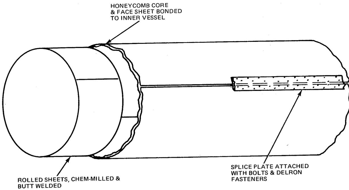
Fig. 65 Sandwich Construction, Method #1 for Concept 5, Orbiter LH<sub>2</sub> Tank
