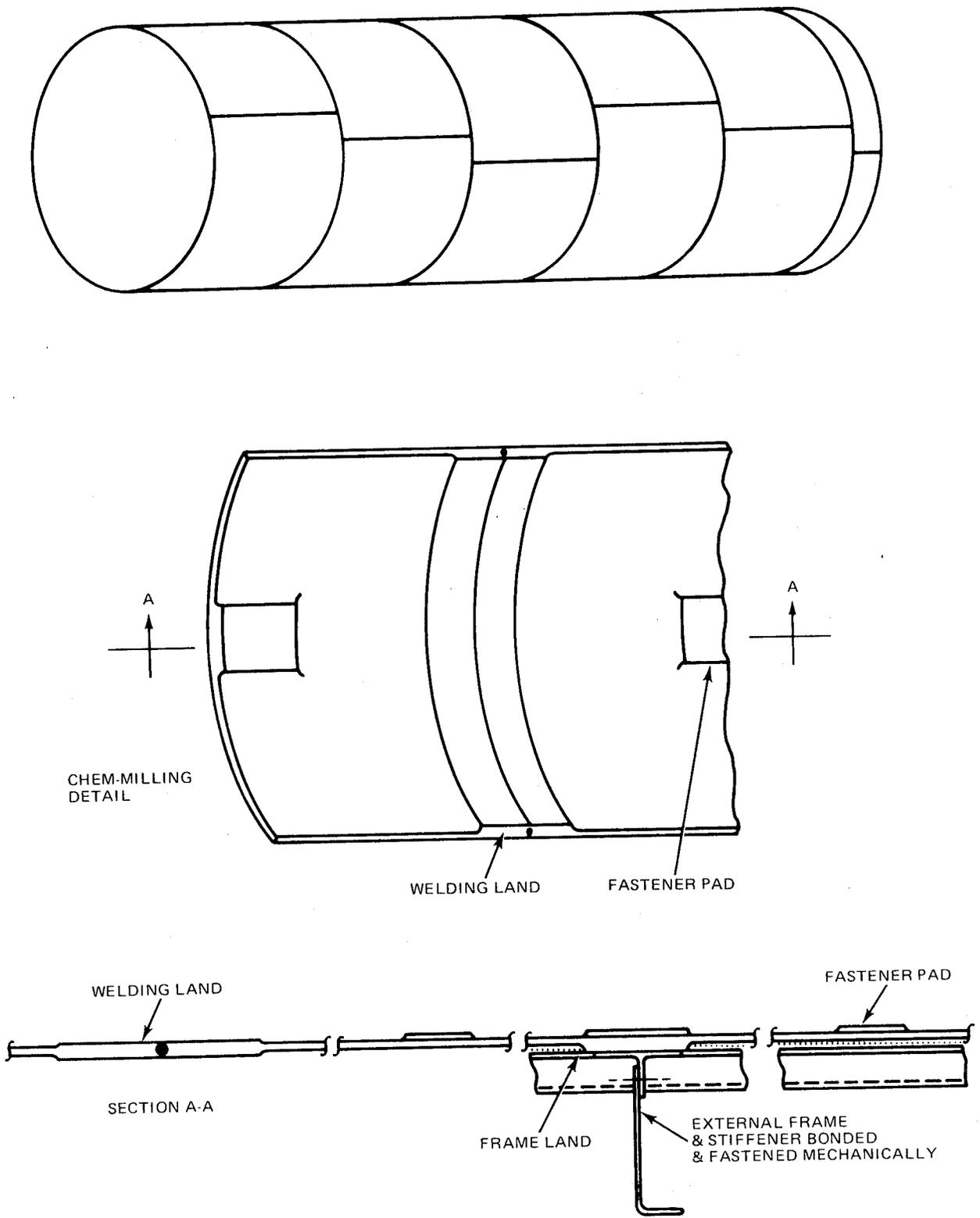
Fig. 16 Plates Rolled, Chem-Milled and Welded for Bonded "Z" Concept Orbiter LH<sub>2</sub> Tank
