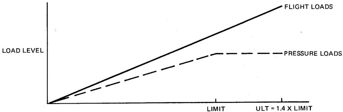
1.4 x flight load is combined with the axial load corresponding to minimum system pressure to determine ultimate axial load. Where internal pressure adds to tensile flight loads, 1.4 x flight load is combined with the axial load corresponding to maximum system pressure. Pressure vessels will be designed for a pressure of 1.4 times maximum limit pressure as a separate design condition.
