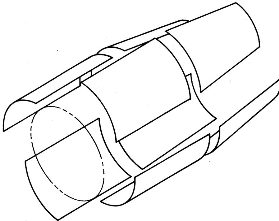
**Fig. 60 Plates Rolled and Welded Longitudinally for Concept 1, Orbiter LO<sub>2</sub> Tank**
