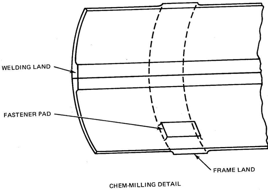
Fig. 62 Plates Rolled and Welded Longitudinally for Concept 2, Orbiter LH<sub>2</sub> Tank
