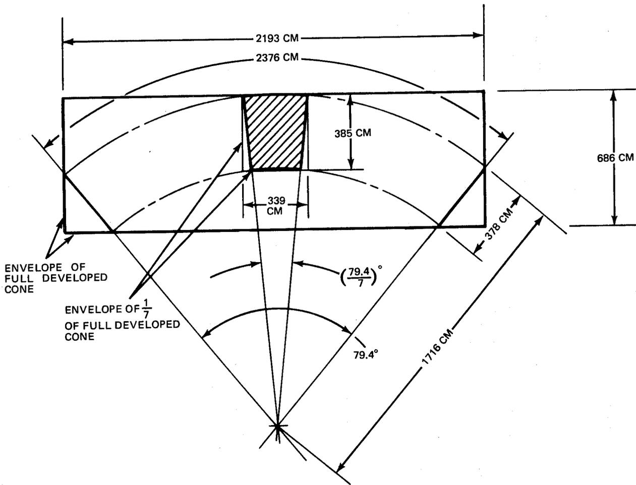
Fig. 9 Developed Cone Surface of Orbiter Lox Tank
