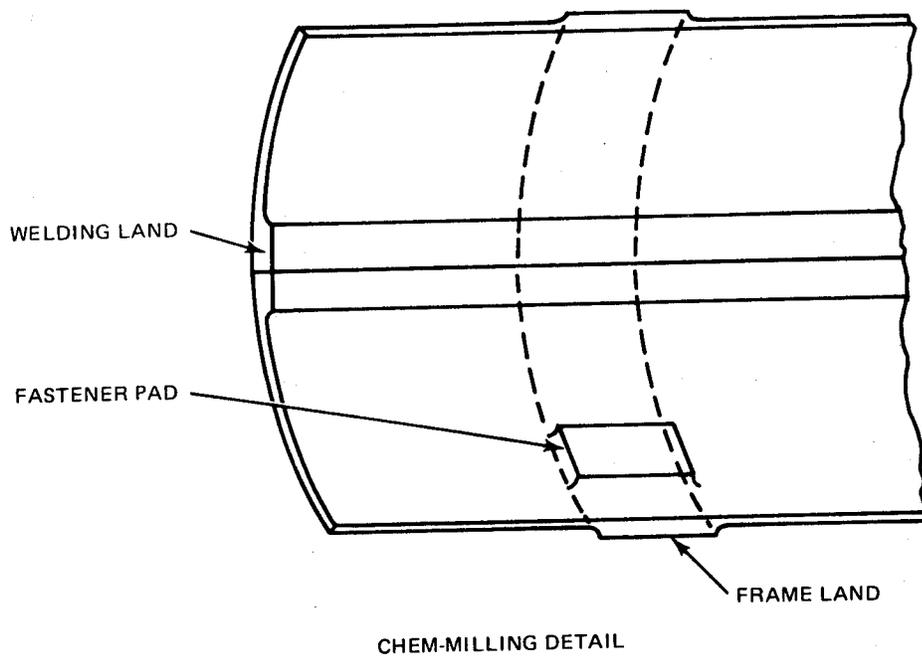
Fig. 15 Plates Rolled and Welded Longitudinally for Bonded "Z" Concept Orbiter LH<sub>2</sub> Tank
