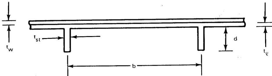
BASED ON 50.8cm RING SPACING FOR THE ORBITER,  $I = 42.7\text{cm}^4$ ,  $A = 4.24\text{cm}^2$ ,
