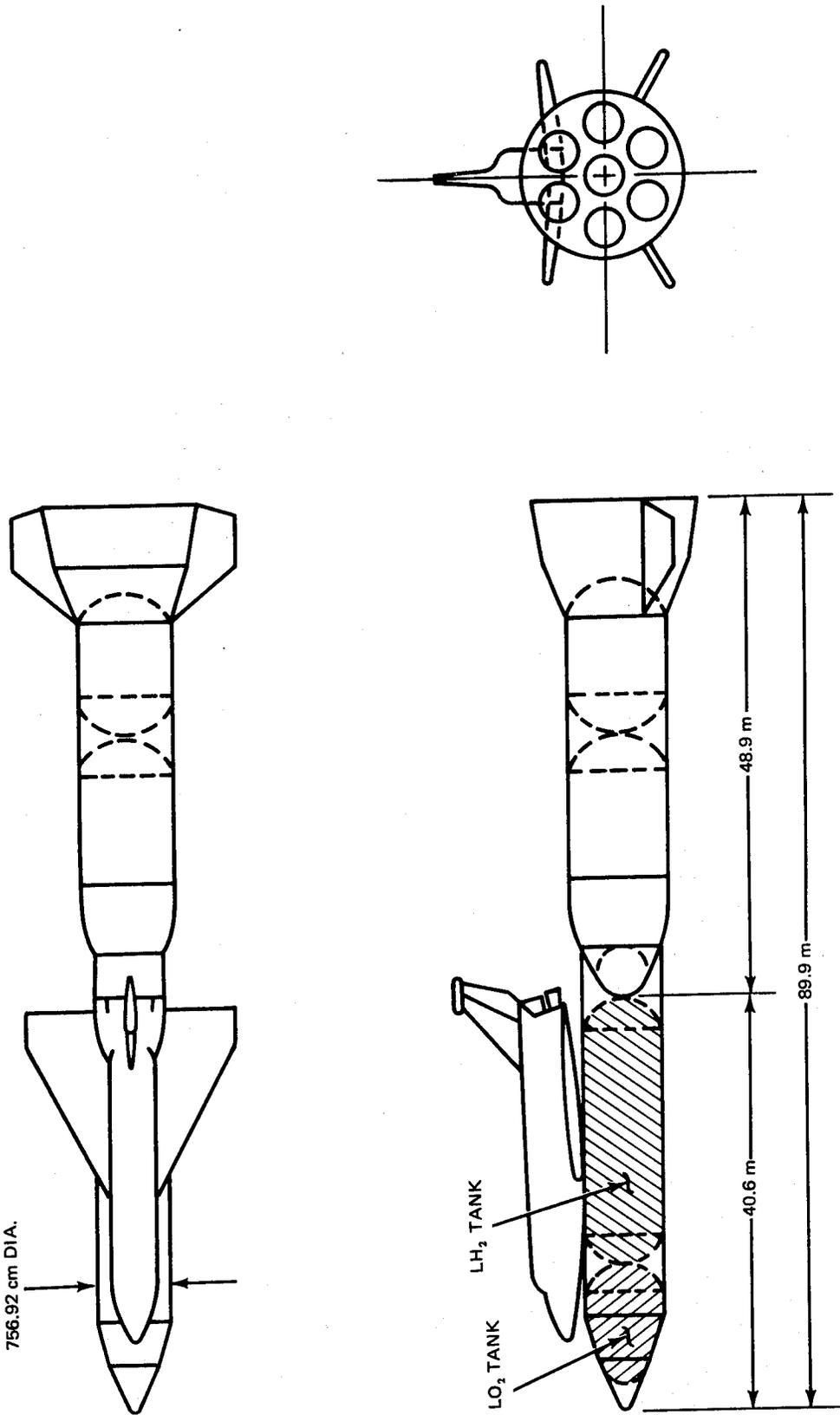
Fig. 1 Series Ballistic Recoverable Configuration External Tanks
