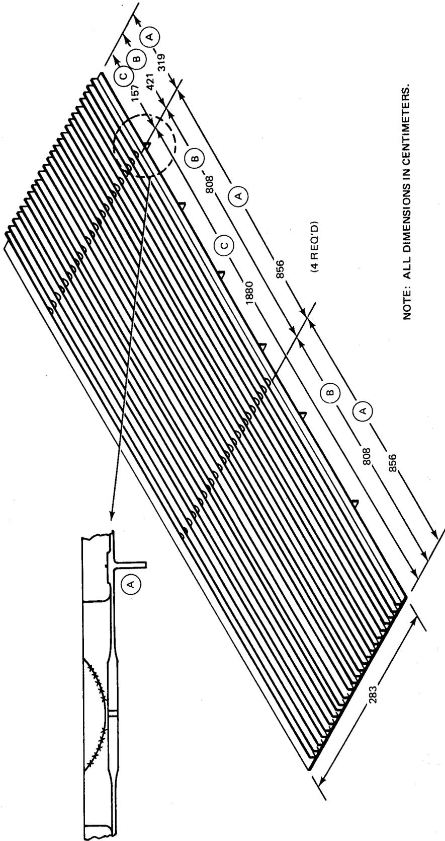
Fig. 11 Longitudinally Machined Flat Plate for Orbiter LH<sub>2</sub> Tank
