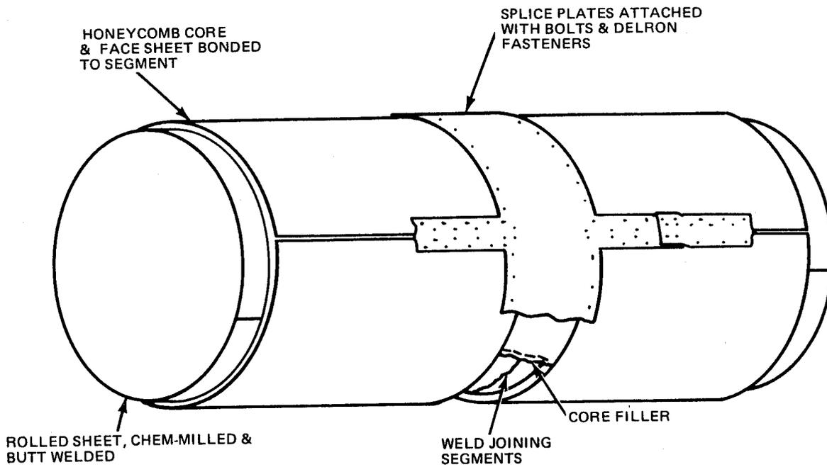
Fig. 66 Sandwich Construction, Method #2 for Concept 5, Orbiter LH<sub>2</sub> Tank
