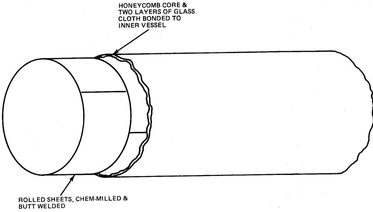
**Fig. 17 Sandwich Construction, Method #1, Orbiter LH<sub>2</sub> Tank**
