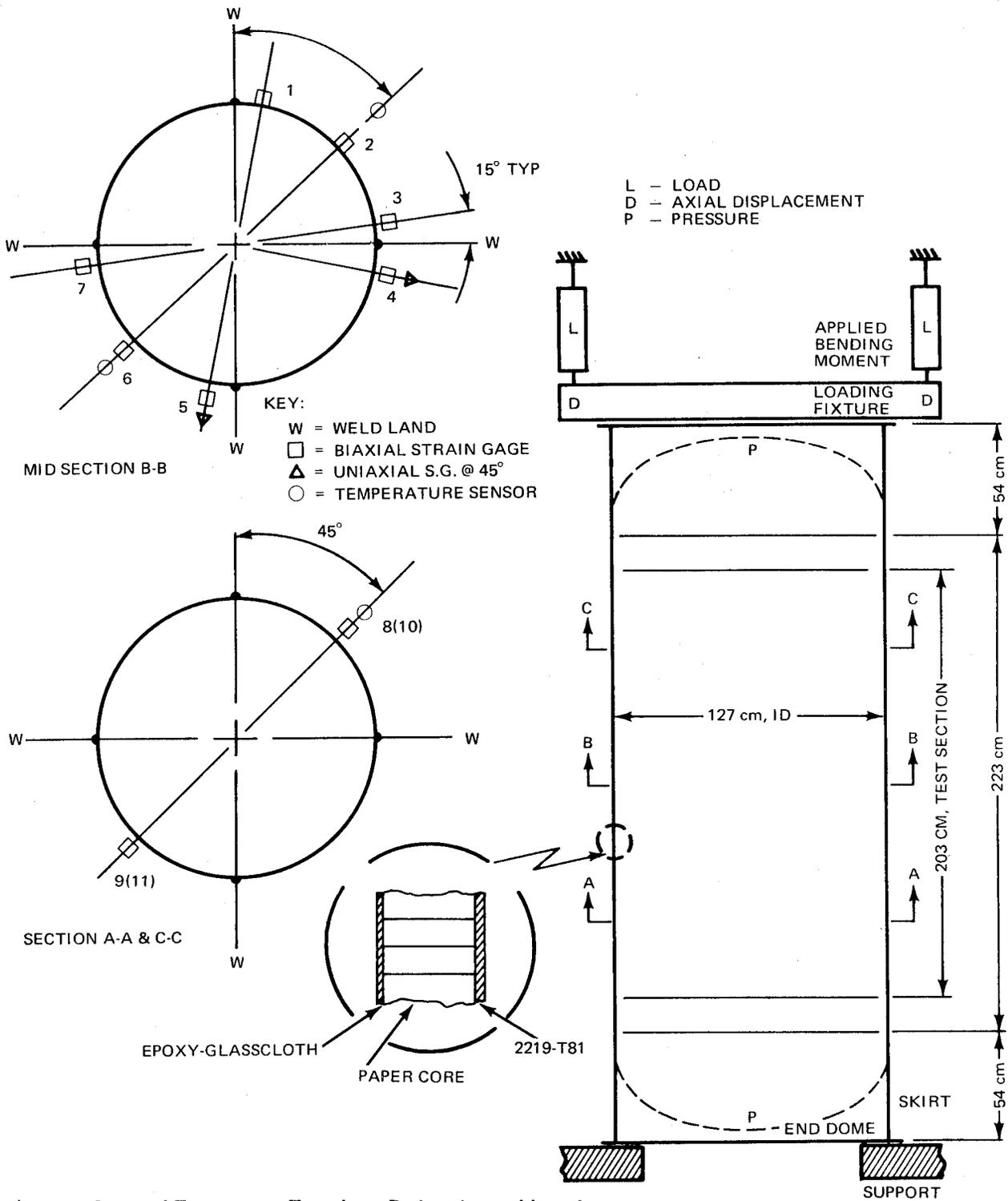
a) Strain Gage and Temperature Transducer Designation and Location
