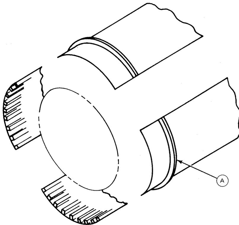
Fig. 12 Plates Rolled and Longitudinally Welded for Orbiter LH<sub>2</sub> Tank
