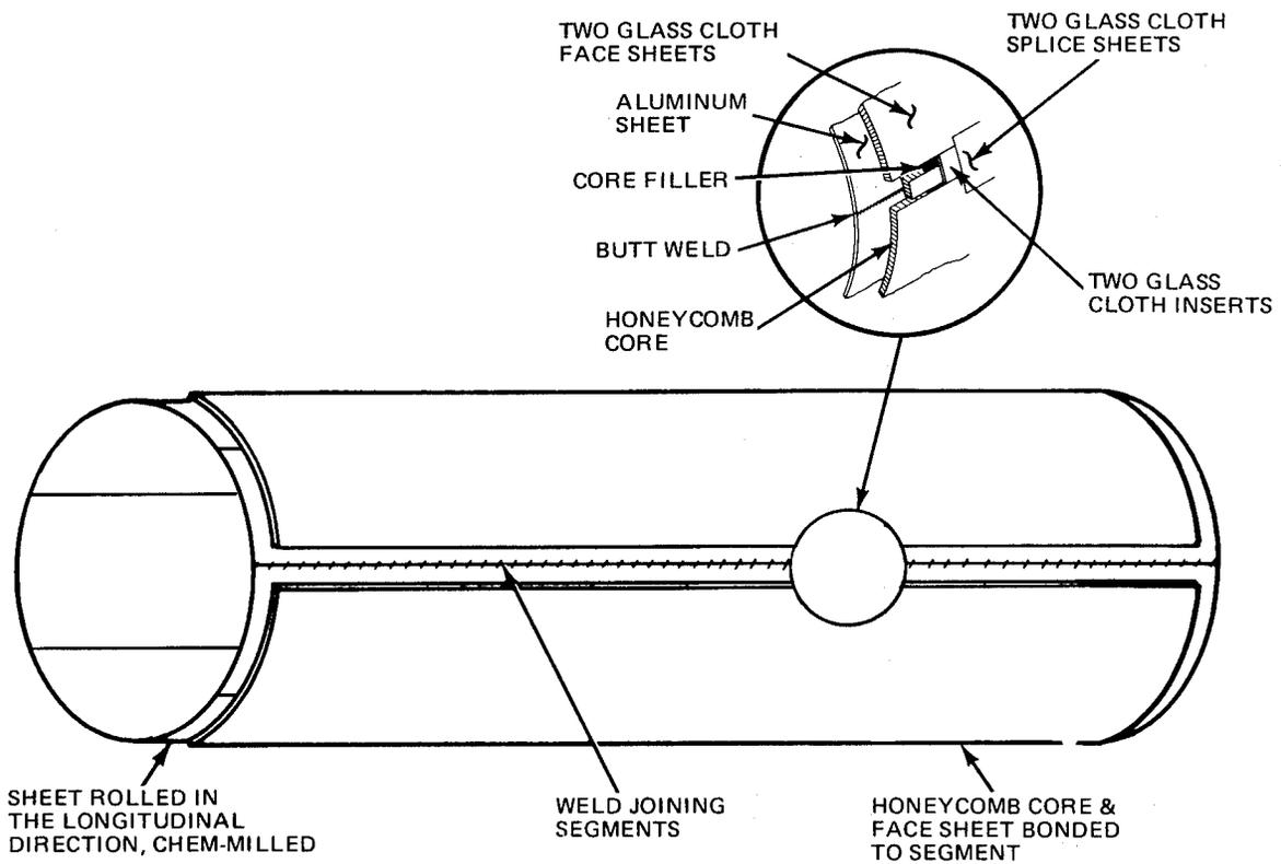
Fig. 19 Sandwich Construction, Method #3, Orbiter LH<sub>2</sub> Tank
