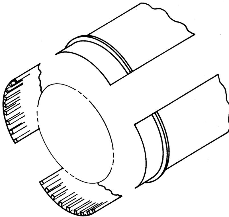
Fig. 56 Plates Rolled and Longitudinally Welded for Concept 1, Orbiter LH<sub>2</sub> Tank
