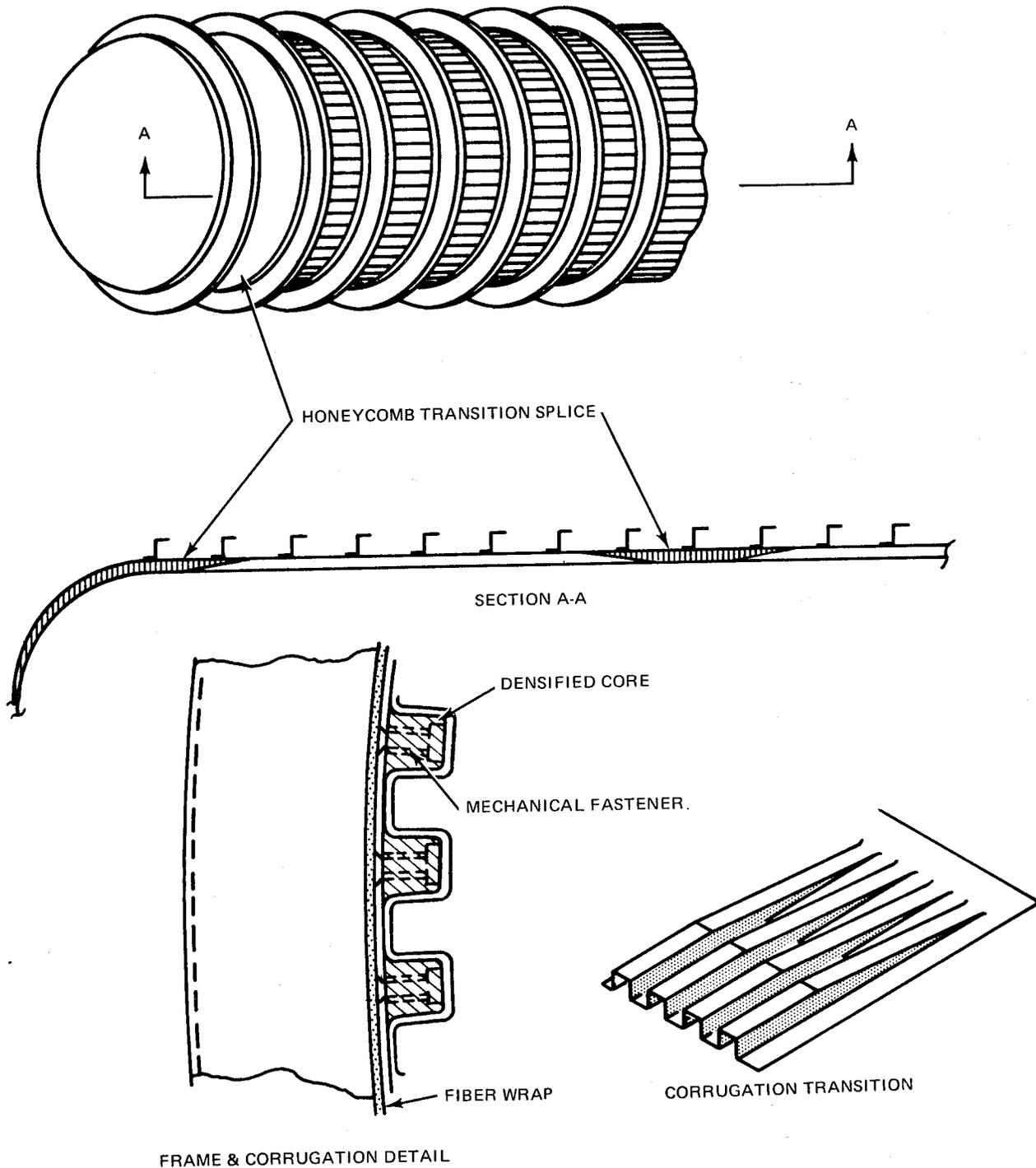
Fig. 68 Concept 6, Corrugated Sheet and Ring Frames
