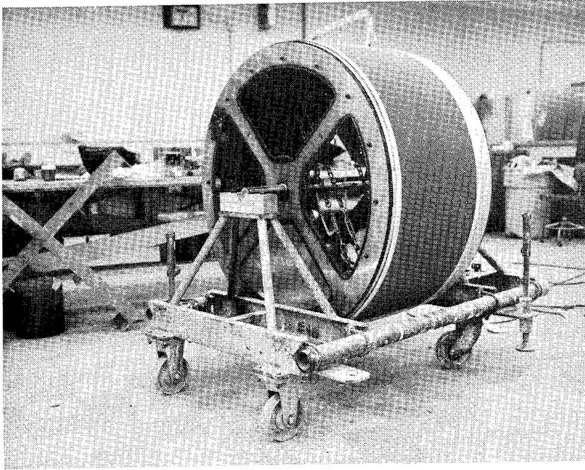
**Fig. 24 Honeycomb Core Applied to Prototype Test Cylinder**
