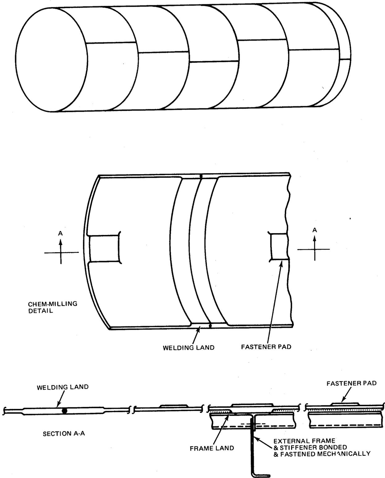
Fig. 63 Plates Rolled, Chem-Milled and Welded for Concept 2, Orbiter LH<sub>2</sub> Tank
