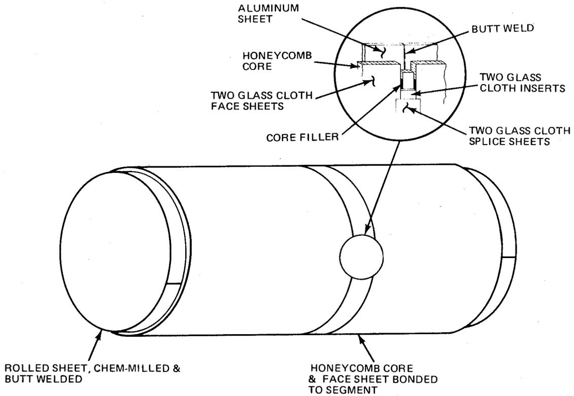
Fig. 18 Sandwich Construction, Method #2, Orbiter LH<sub>2</sub> Tank
