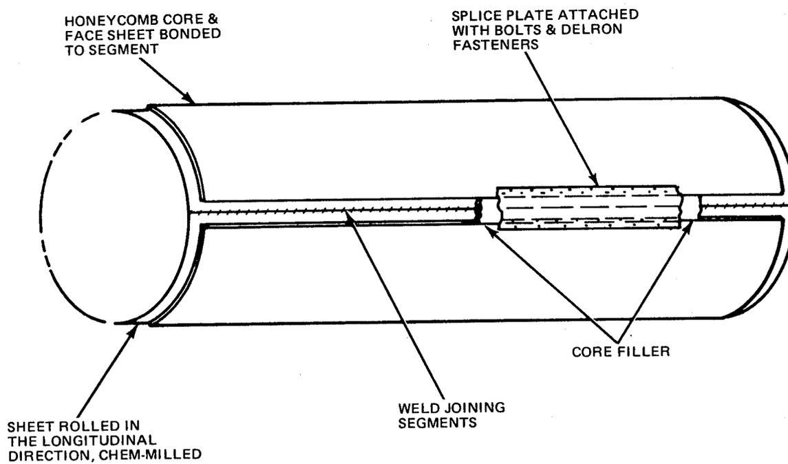
Fig. 67 Sandwich Construction, Method #3 for Concept 5, Orbiter LH<sub>2</sub> Tank
