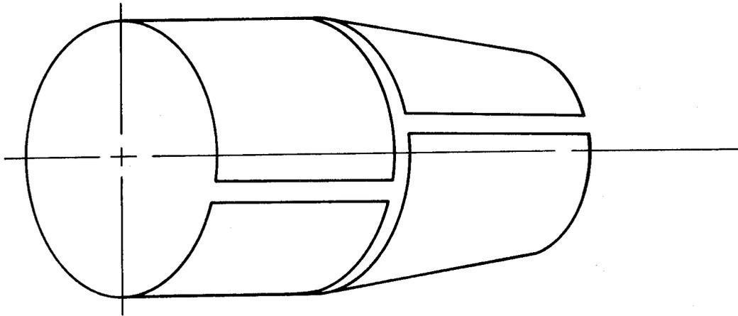
Fig. 64 Plates Rolled, Chem-Milled and Welded for Concept 2, Orbiter LO<sub>2</sub> Tank
