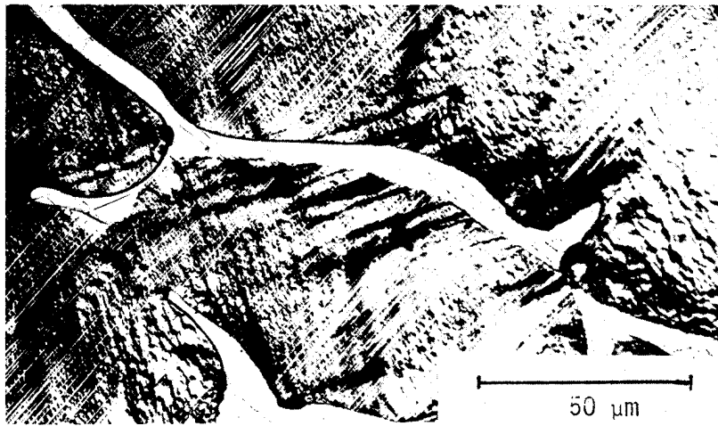
Figure 8. Same specimen as Figure 7, showing austenite deformation associated with twinning in the delta-ferrite. H_3PO_4 etch.
