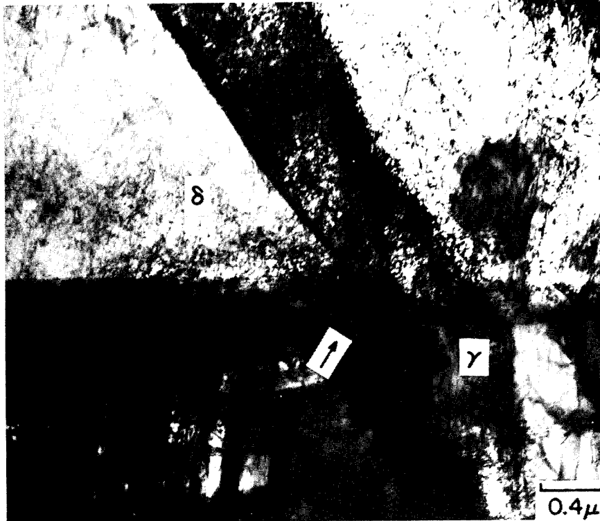
(b). In \gamma ahead of twin (arrow).
