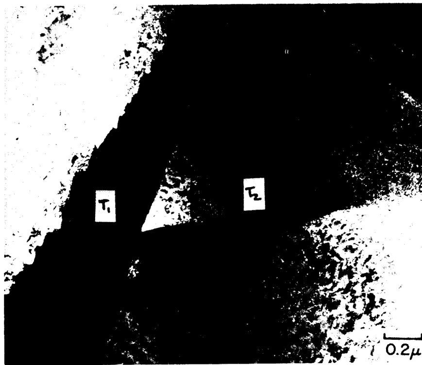
(c). Dark-field employing \delta matrix reflection.
