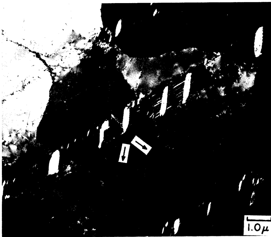
Fig. 21(b). Dark-field employing \alpha' reflection.
