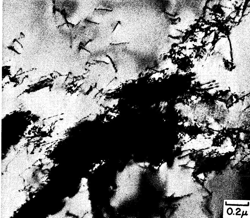
Fig. 20. 17.2 volume percent \delta , \epsilon=0.02 ; dislocations generated in vicinity of forming \alpha' . Transmission electron micrograph.
