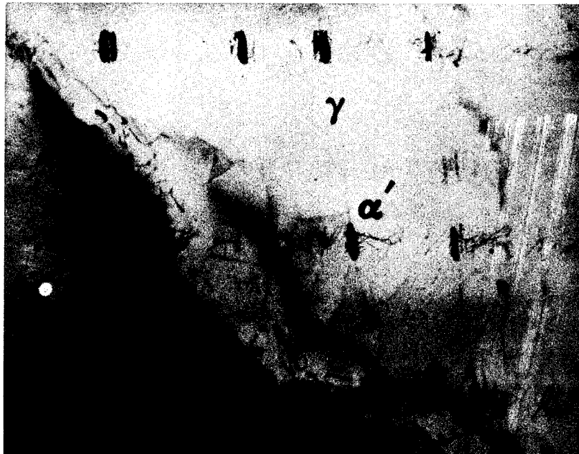
Fig. 4. Fe-18Cr-8Ni austenite strained 0.01 in tension with two active slip systems on \{111\} . Formation of \alpha' along \langle 1\bar{1}0 \rangle intersections of slip planes.
