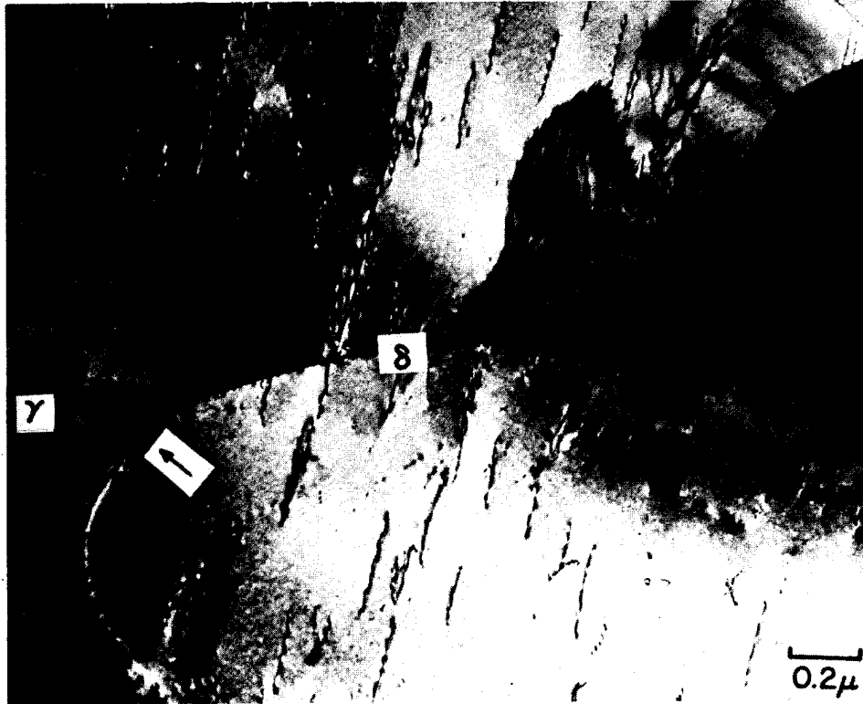
Fig. 7. 28.5 volume percent \delta , low angle boundary in \delta and cusp at boundary - \delta/\gamma interface (arrow). Transmission electron micrograph.
