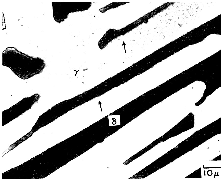
(b). 24 volume percent \delta , ledges on \delta/\gamma interface (arrows). Light micrograph, KOH electroetch.
