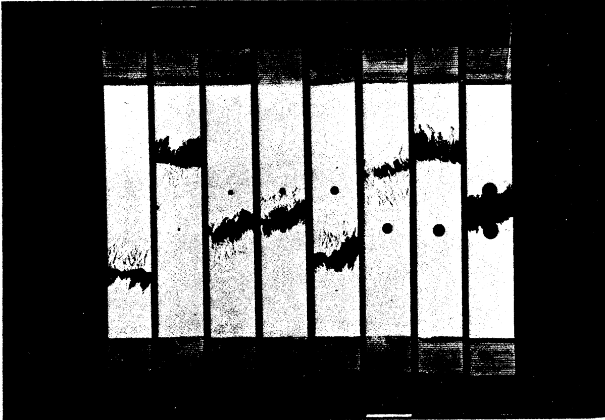
FIGURE 20. SMC-25 FRACTURED NOTCH SENSITIVITY SPECIMENS
