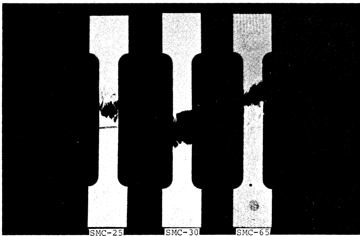
FIGURE 16. FRACTURED STRAIN RATE SPECIMENS
