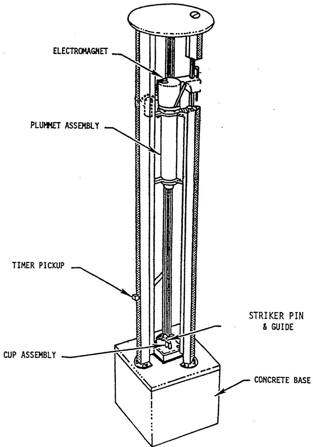
Figure 1: Mechanical Impact Testing Apparatus
