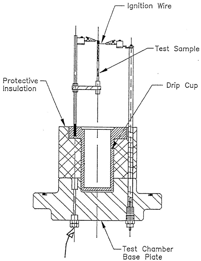
Figure 4. Promoted Combustion Test Apparatus
