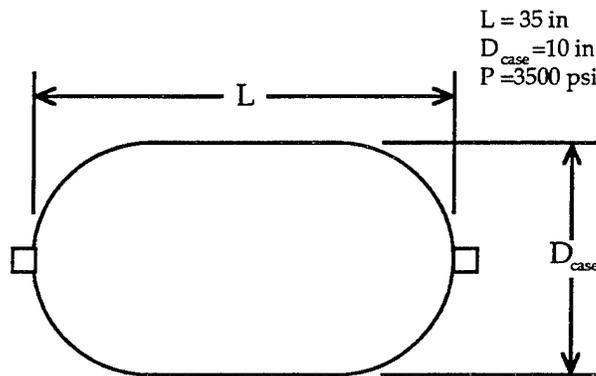
Figure 1. The Pressure Vessel.
