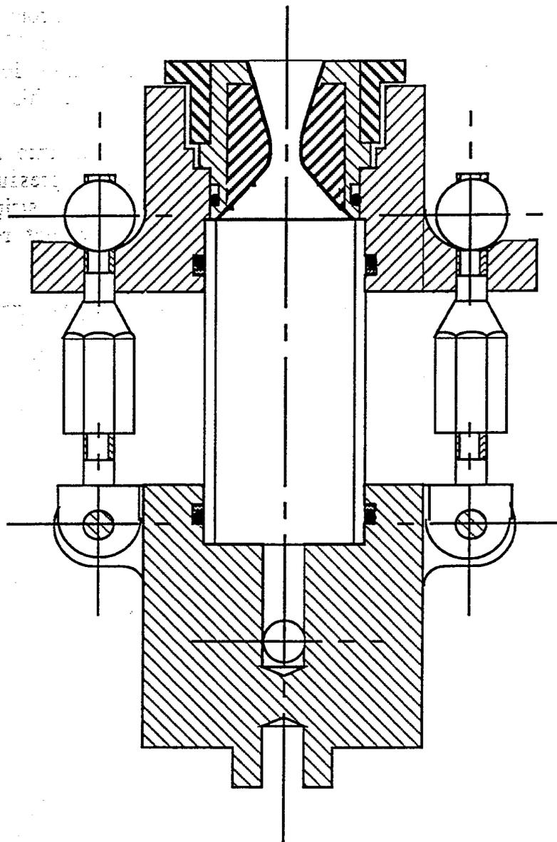
Fig. 5 TEST FIXTURE
