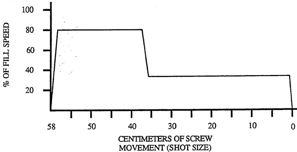
Fig. 17 FILL PROFILE FOR BOTH VECTRA MATERIALS
