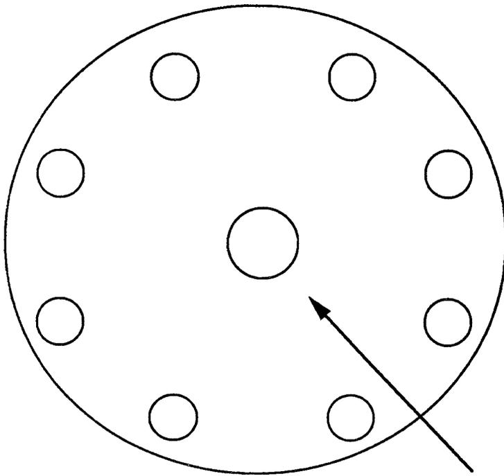
Thermocouple Inlet Port
