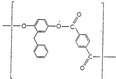
**FIGURE 2. THERMOTROPE STRUCTURE**
