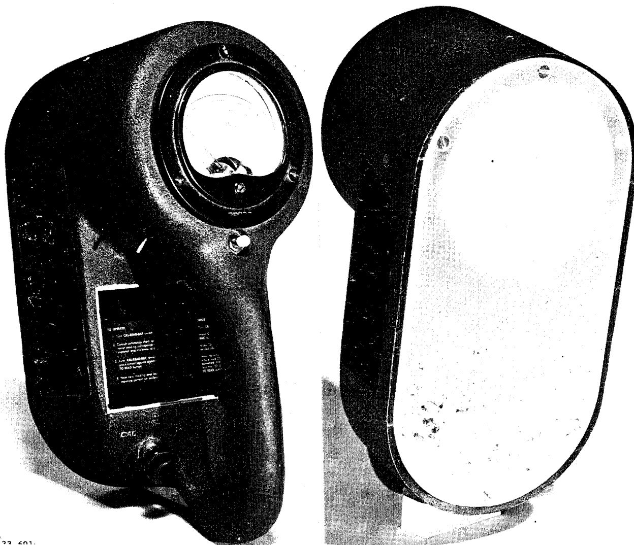
Figure 69.—A moisture meter for indicating percent moisture content of wood. The model shown is of the dielectric type.
