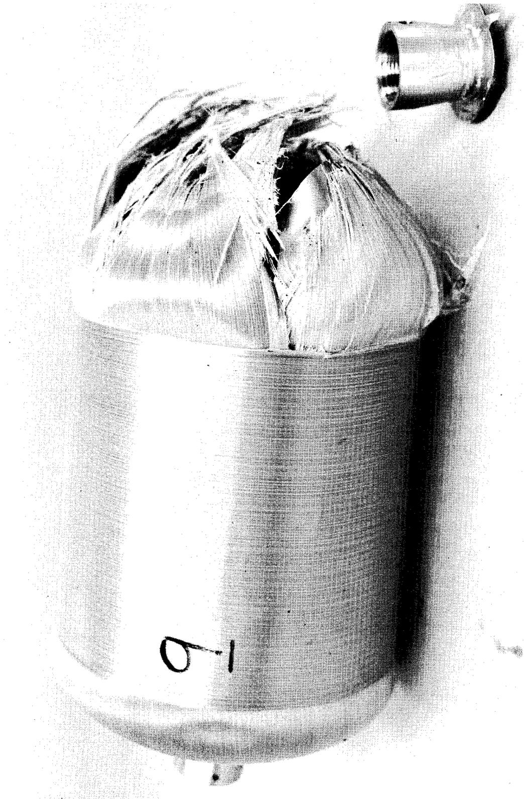
FIGURE 71 - VESSEL NO. 9 AFTER BURST TEST
