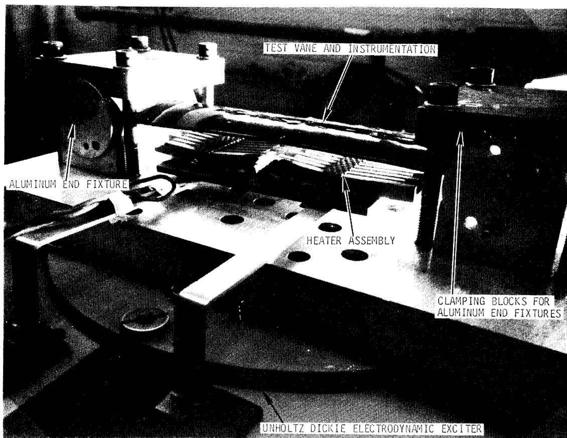
Figure 5-7 Fan Exit Guide Vane Fatigue Test Fixture and Heater Assembly
