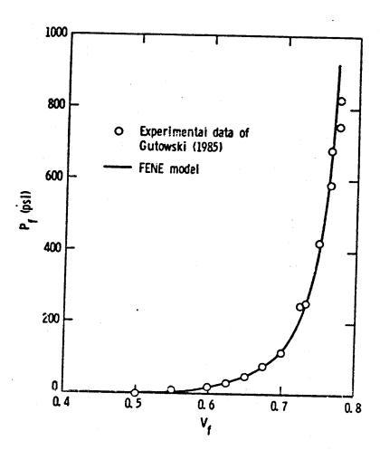
Figure 3. Comparisons between FENE model for the resistance forces of fiber bundles during prepreg lamination process and the experimental data
