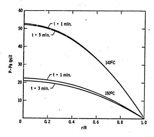
Figure 9. Predicted parabolic pressure distributions which are carried by the resin matrix inside the multi-layer B-stage 1080 glass fabric during isothermal curing at two different temperatures
