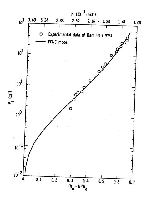
Figure 4. Comparisons between FENE model for the resistance forces carried by the glass fabric during lamination process and the experimental data
