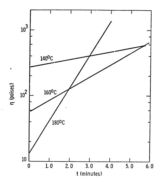
Figure 7. Chemoviscosity profiles for isothermal curing of B-stage epoxy resin [9] at three temperatures
