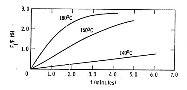
Figure 6. Fractions of applied load carried by the fiber bundles during isothermal processing of B-stage 1080 glass fabric
