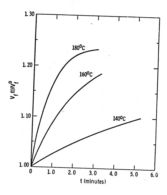
Figure 8. Changes of fiber volume fractions during isothermal processing of B-stage 1080 glass fabric
