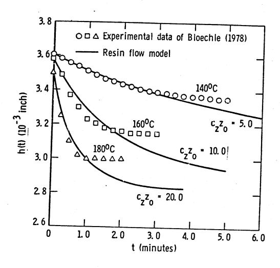
Figure 5. Comparisons between predictions of the resin flow model and the experimental measurements for isothermal processing of B-stage 1080 glass fabric at three different temperatures
