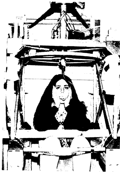
FIG. 13. Kowler in position for two-dimensional recording of rotations of her head by means of the magnetic-field search-coil technique. The head search coil is mounted on a dental bite plate. The field coils can be seen surrounding the subject who is using her hands to support her head.
