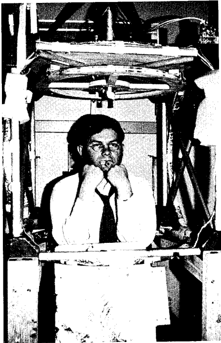
FIG. 18. Robinson in position for two-dimensional recording of rotations of his head by means of the magnetic-field search-coil technique. The head search coil is mounted on a dental bite plate. The field coils can be seen surrounding the subject who is using his hands to support his head.
