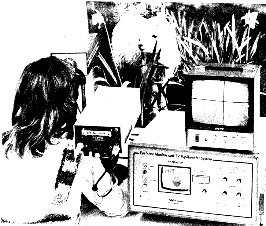
FIG. 1. Television scan type eye-movement measurement system with various operator indicators.
