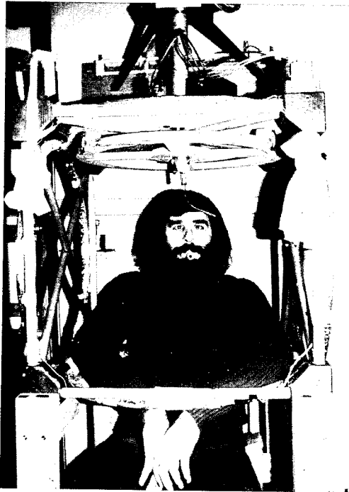
FIG. 9. Murphy in position for two-dimensional recording of rotations of his head by means of the magnetic-field search-coil technique. The head search coil is mounted on a dental bite plate. The field coils can be seen surrounding the subject.
