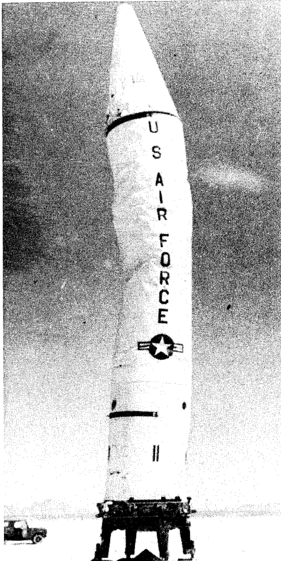
Damage to Titan Missile exposed to air blast
