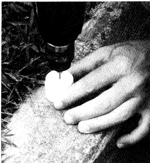
Figure B6. A hole is drilled in the PVC pipe cap (a), which is placed on the end of the pipe opposite the cross hairs (b)
