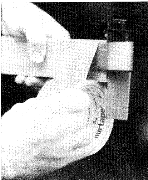
Figure B3. The canister is taped securely to the frame
