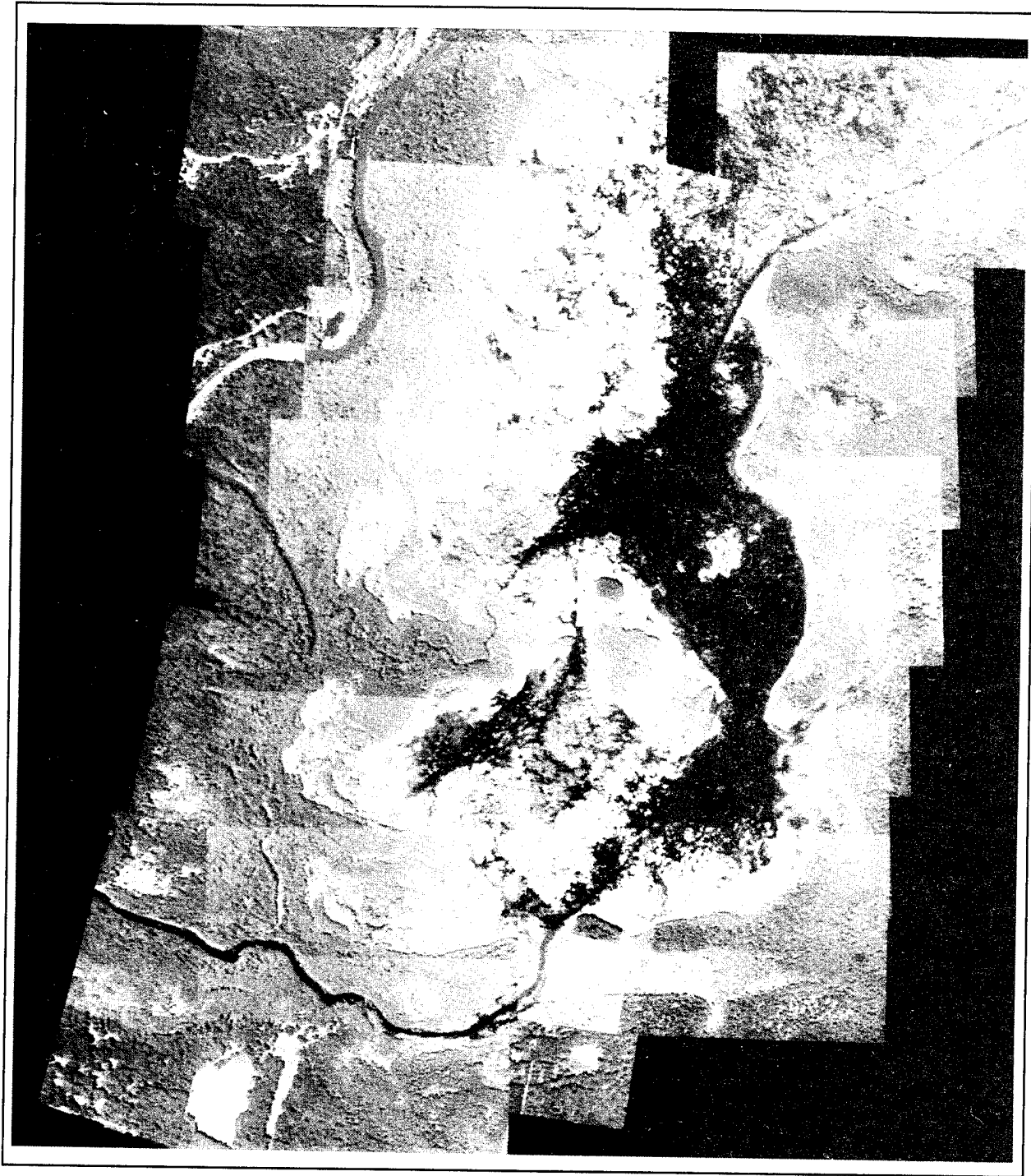
Figure 3. Example of large-scale study area mosaic of 3-band composite video imagery for the Carter Lake area of Caddo Lake (printed as monochrome for publication)
