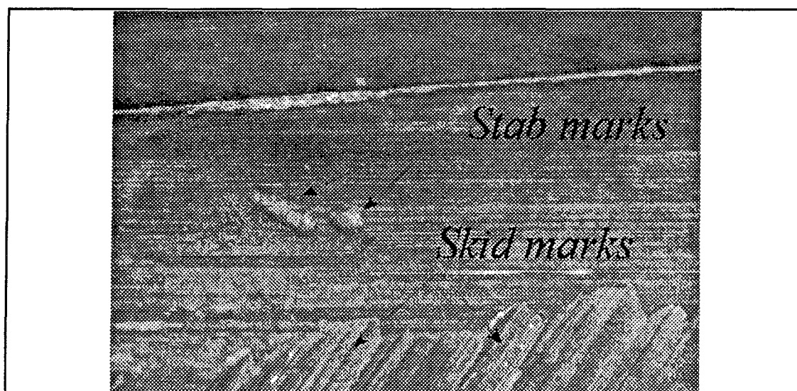
Figure 2 Bullet image showing skid marks and stab marks.
