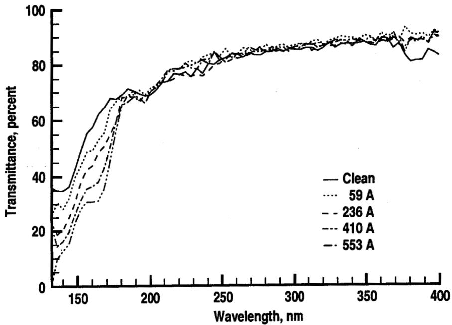
Figure 3. Transmittance as function of DC6-1104 film thickness.
