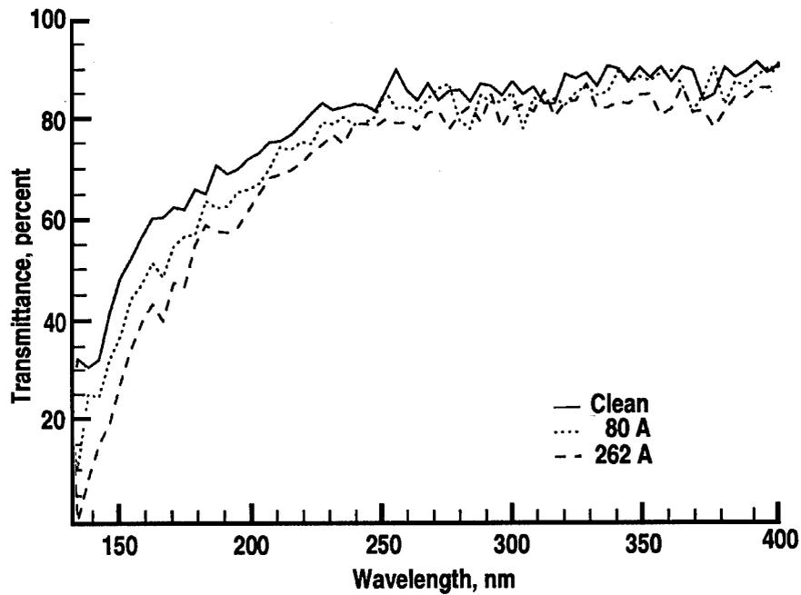
Figure 5. Transmittance as function of RTV-142 film thickness.
