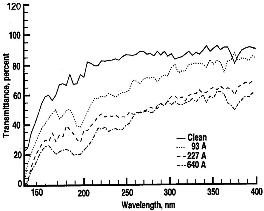
Figure 6. Transmittance as function of Uralane® film thickness.
