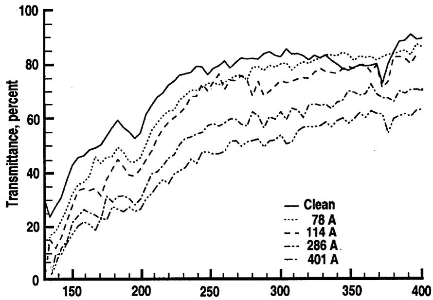
Figure 4. Transmittance as function of Solithane film thickness.
