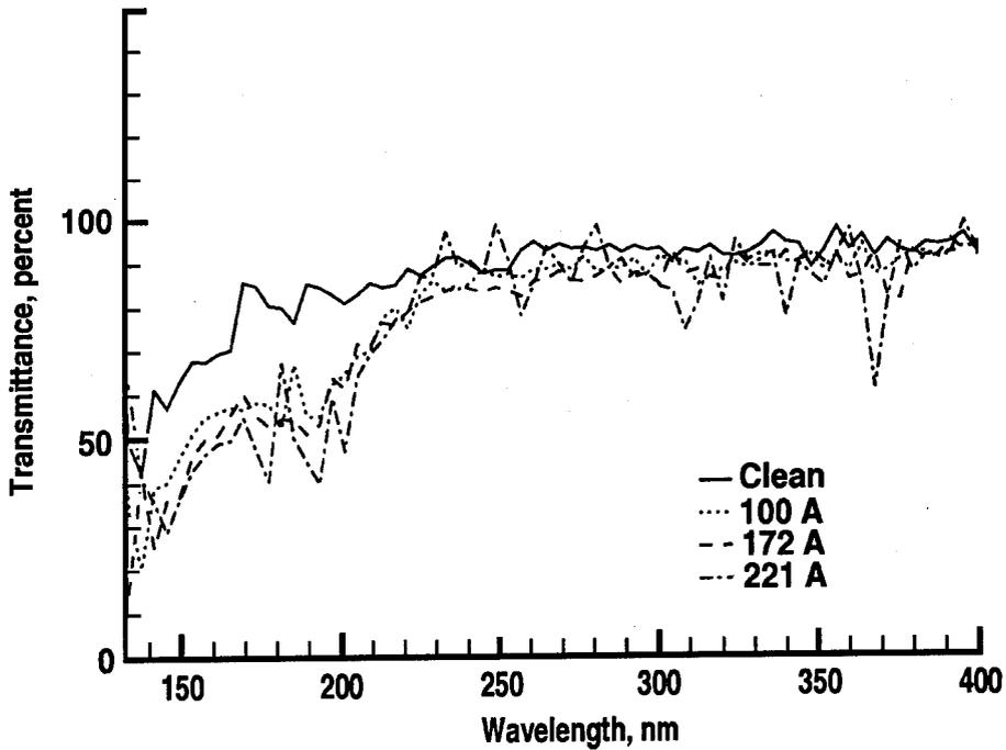
Figure 7. Transmittance as function of RTV-566 film thickness.
