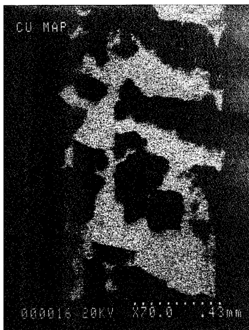
Figure 4.8 Copper EDS map of etched connector pin. Magnification: 70X.
