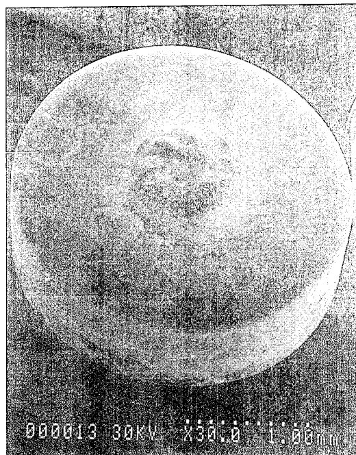
Figure 3.10 Contact from a 10 A circuit breaker cycled 20,000 times at rated dc load current at 28 Vdc. Magnification: 30X.
