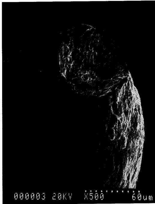
Figure 2.10 Figure 2.10 shows the cup-and-cone fracture surface and elongation typically associated with mechanical failure of a copper conductor.
