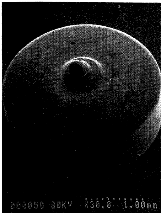
Figure 3.16 Close up of pip on negative contact. Magnification: 100X.
