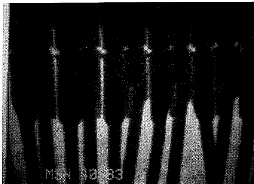
Figure 4.3 Microfocus x-ray radiograph of solder reflow anomaly on a connector. Note the missing solder in alternating contacts. Magnification: about 5X.
