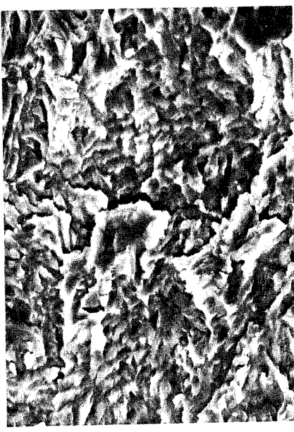
FIGURE 29 SEM fractograph of transgranular / ductile region on USARL-MD fatigue specimens. Mag. 1,500x.
