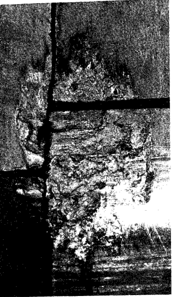
FIGURE 6 Macrograph of the severely galled region and vertical wear marks adjacent to the crack initiation site on the inner diameter bolt surface. Mag. 1.5x.
