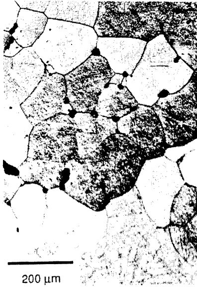
Figure 3. Equiaxed microstructure of a heat-treated 771.0 Al sample showing both angular and spherical cavities and secondary constituents.
