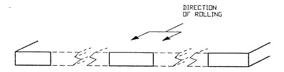
A. For plate thicknesses 0.250 to 0.500 inch, inclusive. Total number of samples from plate = 7 (3 per end plus one from center as shown in figure 2).
