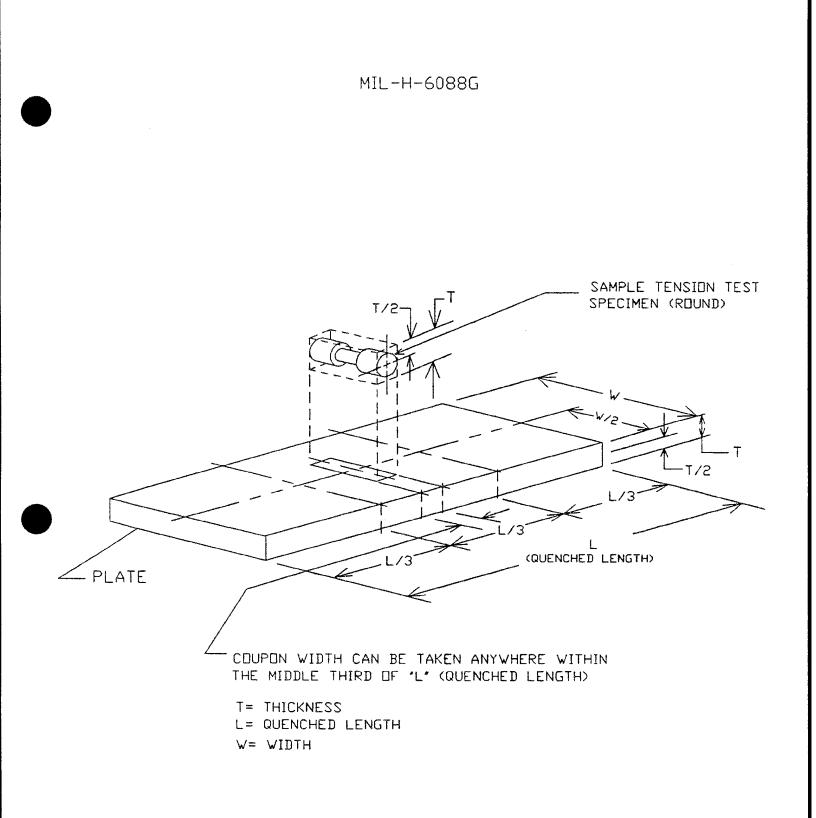
FIGURE 2. Allowable location to sample tension specimen from approximate location of center of plate.
