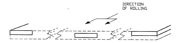
B. For plate thicknesses over 0.500 to 1.0 inches, inclusive. Total number of samples from plate = 11 (5 per end plus one from center as shown in figure 2).
