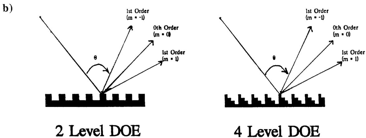
Figure 3. a) SEM of a linear diffraction grating, and b) the diffracted "orders" off the linear grating.
