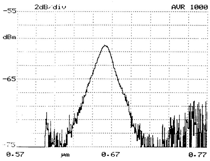
Figure 10. Optical spectrum output for an LED at 100mA.
