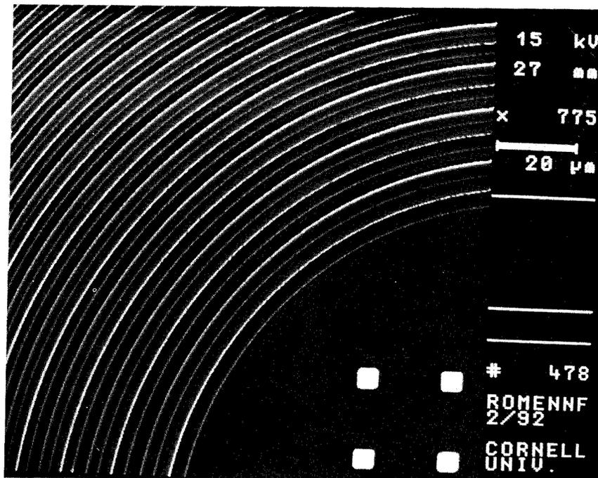
Figure 2. Scanning electron micrograph of 4-level focusing diffractive optic elements.
