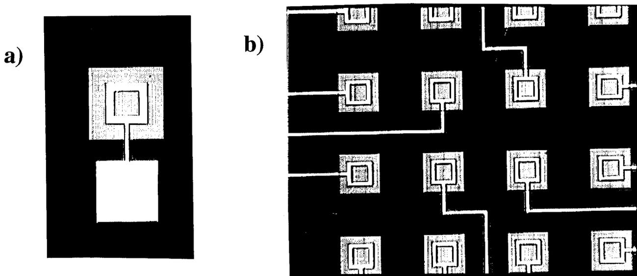
Figure 6 a) individual GaAsP LEDs and, b) an array of 16 50 X 50 $\mu\text{m}$  LEDs.
