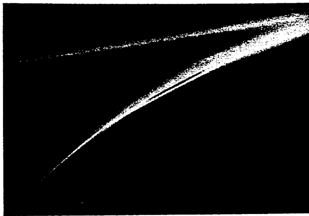
Fig. 1. Photomicrograph of stimulated beams inside a BaTiO 3 cat conjugator, showing the segmented bent trajectories of the light beams.
