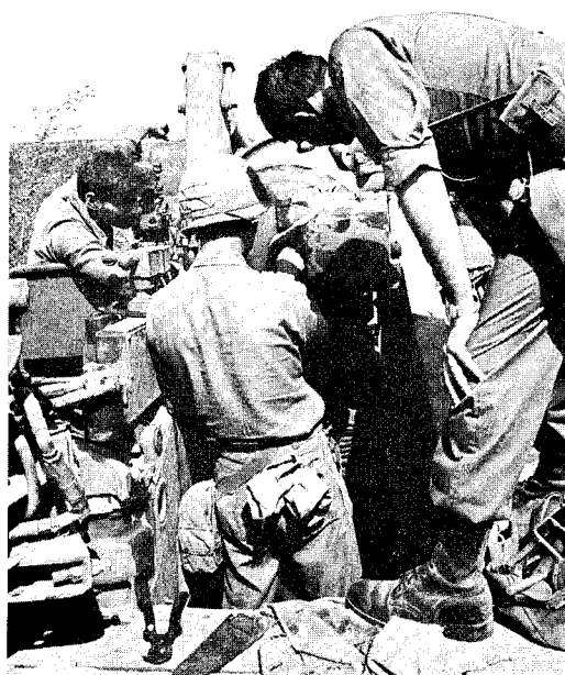
While other crew members watch, the section chief repairs the firing mechanism of an 8-inch self-propelled howitzer during his unit's annual training at Fort Drum, NY, in 1982. (US Army photo)
