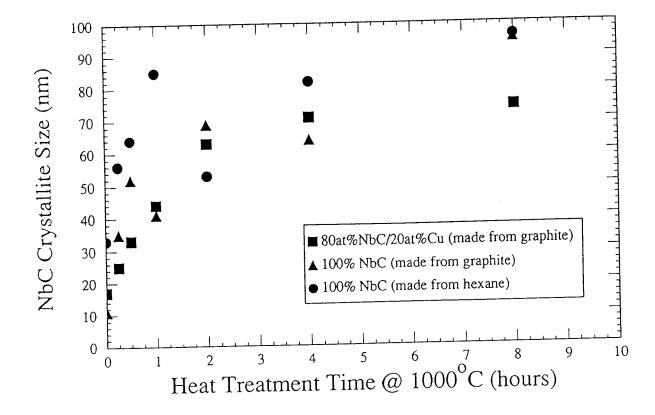
Figure 2: NbC crystallite size as a function of exposure time at 1273 K. Shown are x-ray crystallite sizes for as-synthesized powder (heat-treatment time of 0), for "quick hipped" powder (heat-treatment time of 1/4 hr) and for conventionally hipped powder (time=1 hr.) and for these materials after heat-treatment for extended times at the 1273 K. Consolidated structures slowly coarsen, but remain in the nanometer range even after extended thermal exposure at 1273 K.
