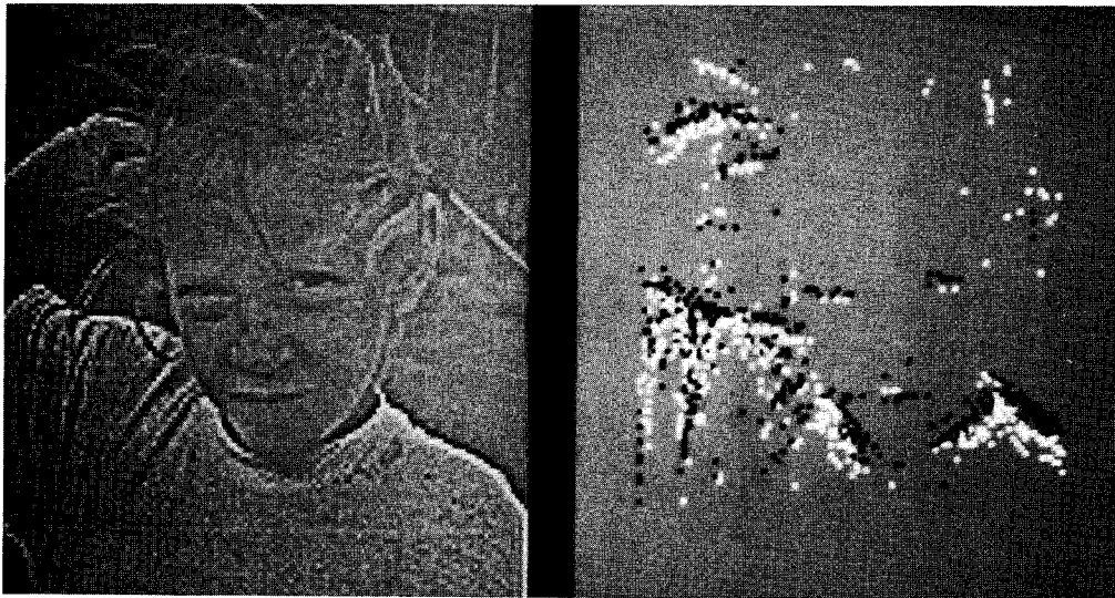
Figure 1.7 The left panel is the whitened image from figure 1.4. In the right panel white dots are placed at the positions of the upper extreme values of the distributions of the sum of pixels in a line shown in figure 1.6, and dark dots at lower extreme values. The extreme values obviously occur at the borders of objects in the image. Hence the combinations of pixel values that occur at edges are ones that would not be expected by chance.
