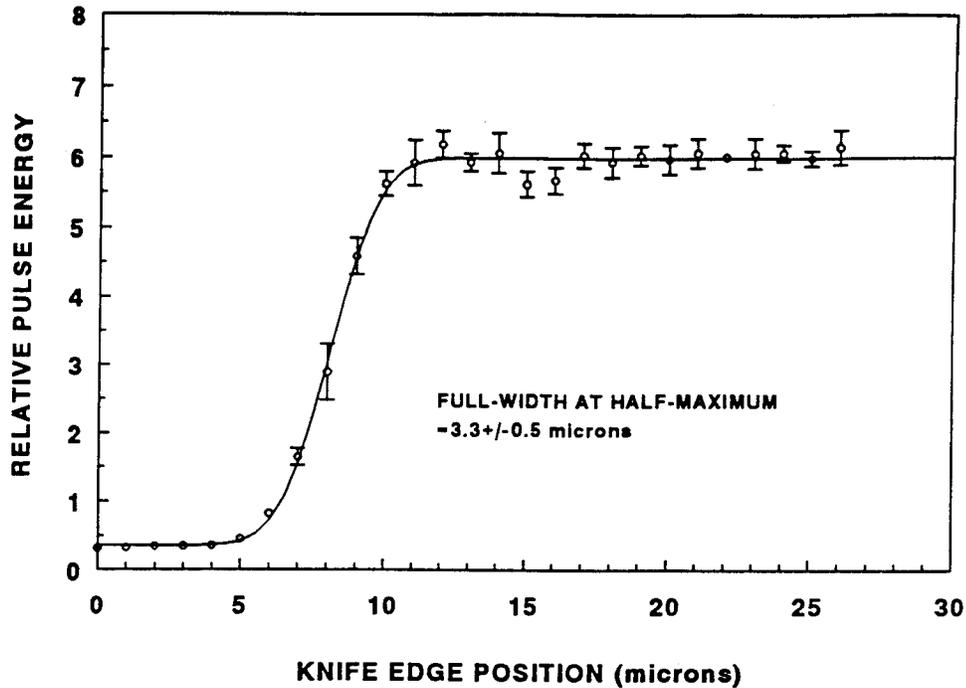
**Figure 6.** Measurement results for determination of the minimum spot size, for the focused 1060 nm radiation. The spot size was measured to be  $3.3 \pm 0.5 \mu\text{m}$ .
