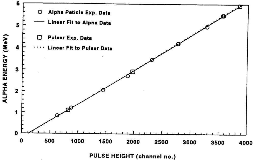
**Figure 8.** Experimental results for determination of alpha particle energy as a function charge collected, in terms of pulse height, from the MRD500 photodiode. The pulser reference data is also shown.
