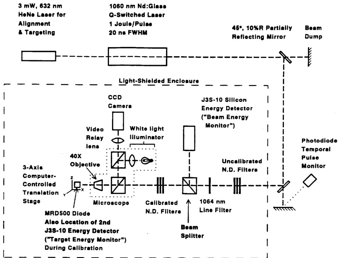
**Figure 3.** Experimental arrangement for laser SEU simulation.
