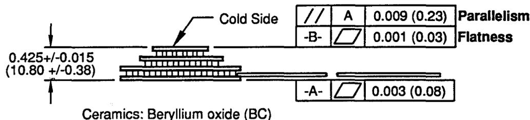
Dimensions in inches and (mm). Tolerances unless otherwise specified are ±.010 (0.25).
