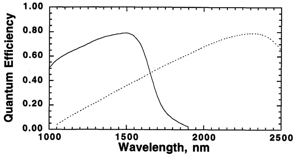
Figure 1 Quantum efficiency for InGAs detectors; data provided by Epitaxx. The solid line is for a 1.7  $\mu\text{m}$  cutoff detector, the dashed line is for a 2.6  $\mu\text{m}$  cutoff detector.
