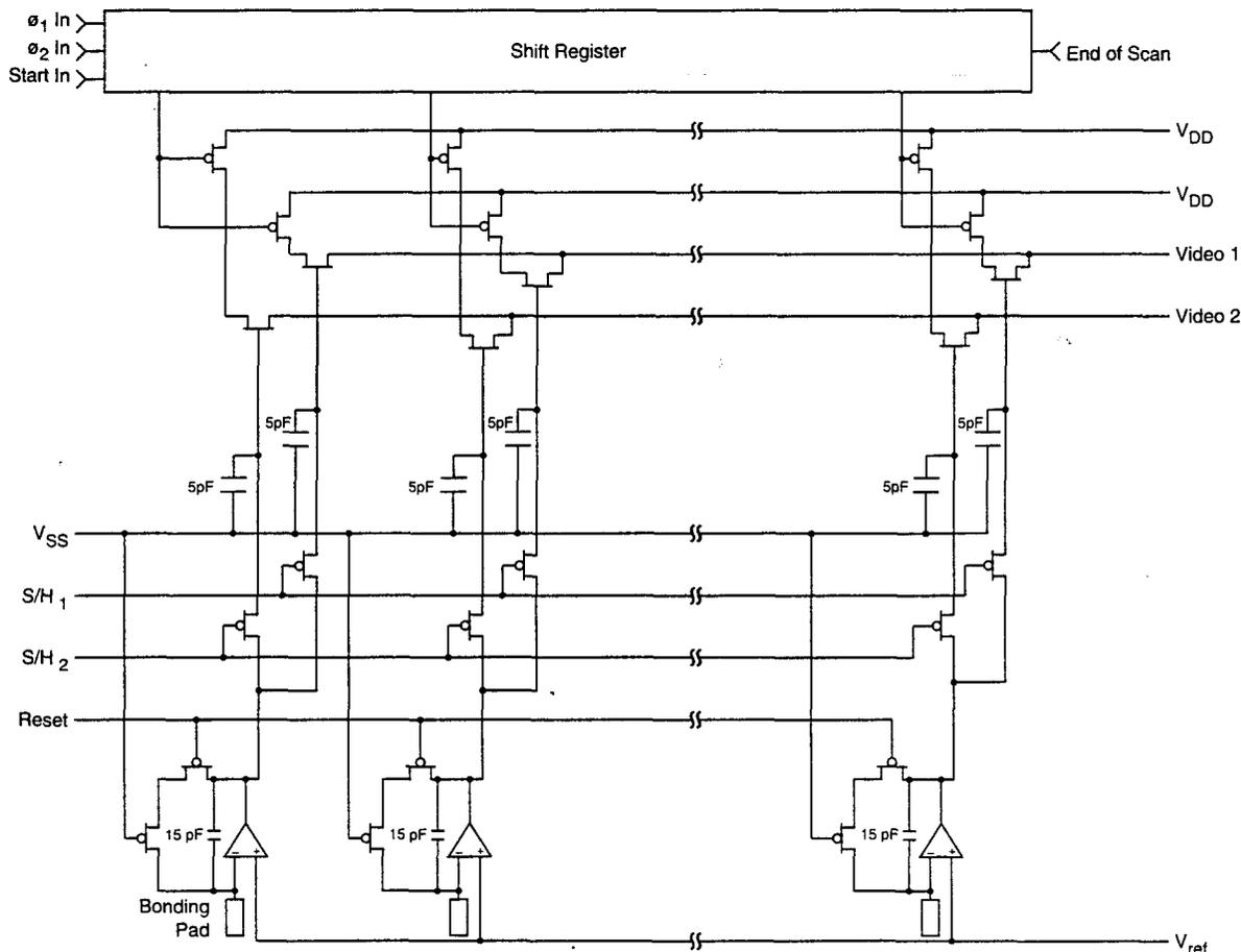
Figure 1. Simplified Block Diagram of the Multiplexer
