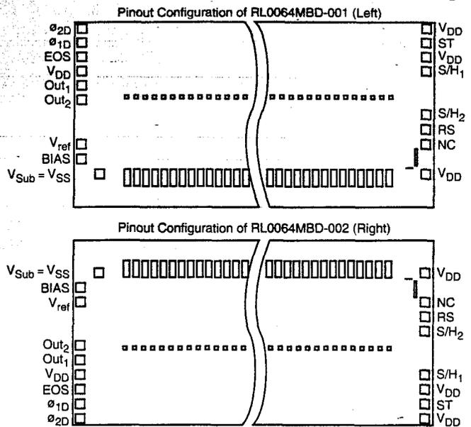
Figure 4. Pinout Configurations
