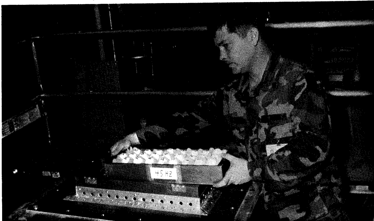
Figure A-2. Top of MTS ® table showing metal fixture and the bottom of wooden tray used to incubate eggs. For illustration purposes only, the eggs were numbered with a felt-tipped black marker.
