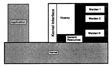
This figure shows the internal structure of a typical Odyssey client. Applications make requests on Odyssey objects. These requests are redirected through the kernel to the kernel interface of the Odyssey cache manager. The viceroy fields each request, handles generic operations, and passes all other operations on to individual wardens. Resources, such as cache space, are loaned to wardens by the viceroy. When necessary, the viceroy notifies applications of changes in resource availability.
