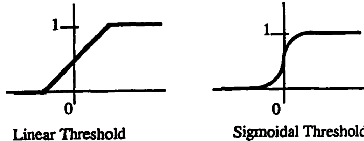
FIGURE 9. LINEAR AND SIGMOIDAL THRESHOLD
