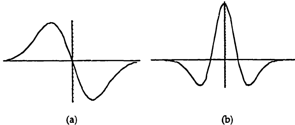
Figure 22. Wavelet basis functions: (a) first-order Gaussian derivative (FOGD), and (b) difference of Gaussian (DOG).
