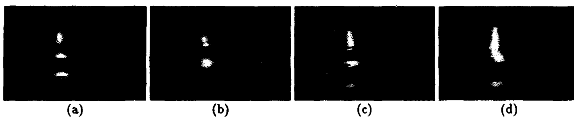
Figure 7: Double wavefront reflected and diffracted off a harbour wall. First wave (a). Reflection of first wave off harbour wall (b). Superposition of the first reflected wave and second wave (c). Wave Diffraction (d).
