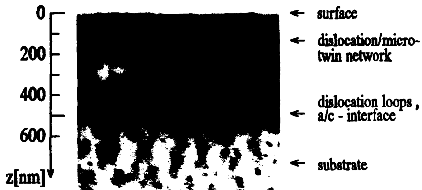
Fig. 4 Cross-section TEM - bright field image for an annealed (975°C/50 s) room temperature sample.
