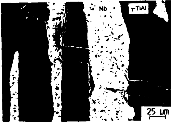
Fig. 10. SEM micrograph of fracture path morphologies in Nb/TiAl composites under monotonic loading. Note the extensive debonding at the interface compared to TiNb/TiAl composites.
