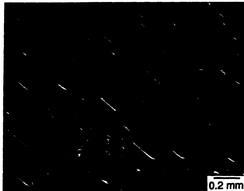
Fig. 9. SEM view of fatigue fracture surface, showing the extent of fiber pullout.
