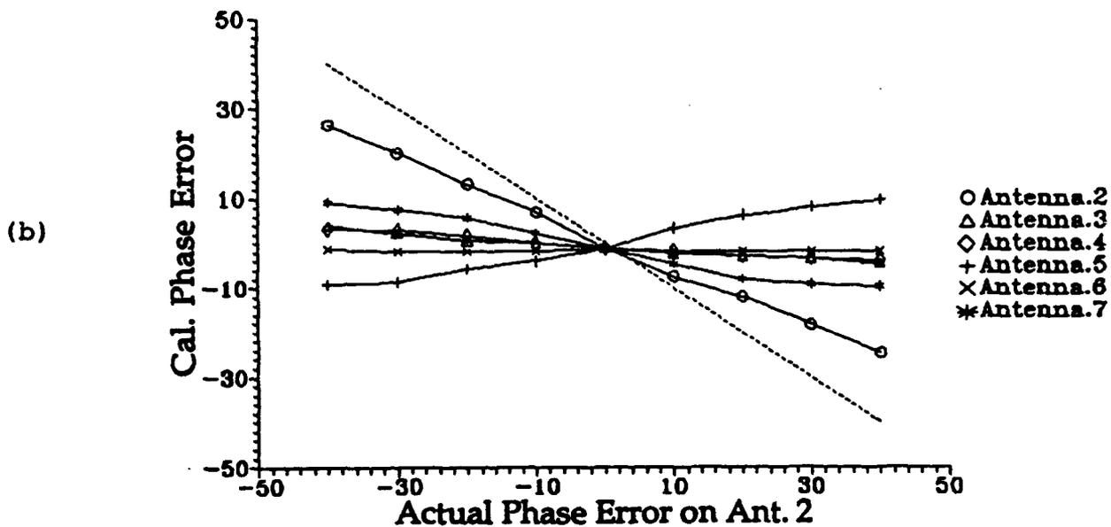
Figure 5. Calculated Phase Error Corrections Using Mode 2.
