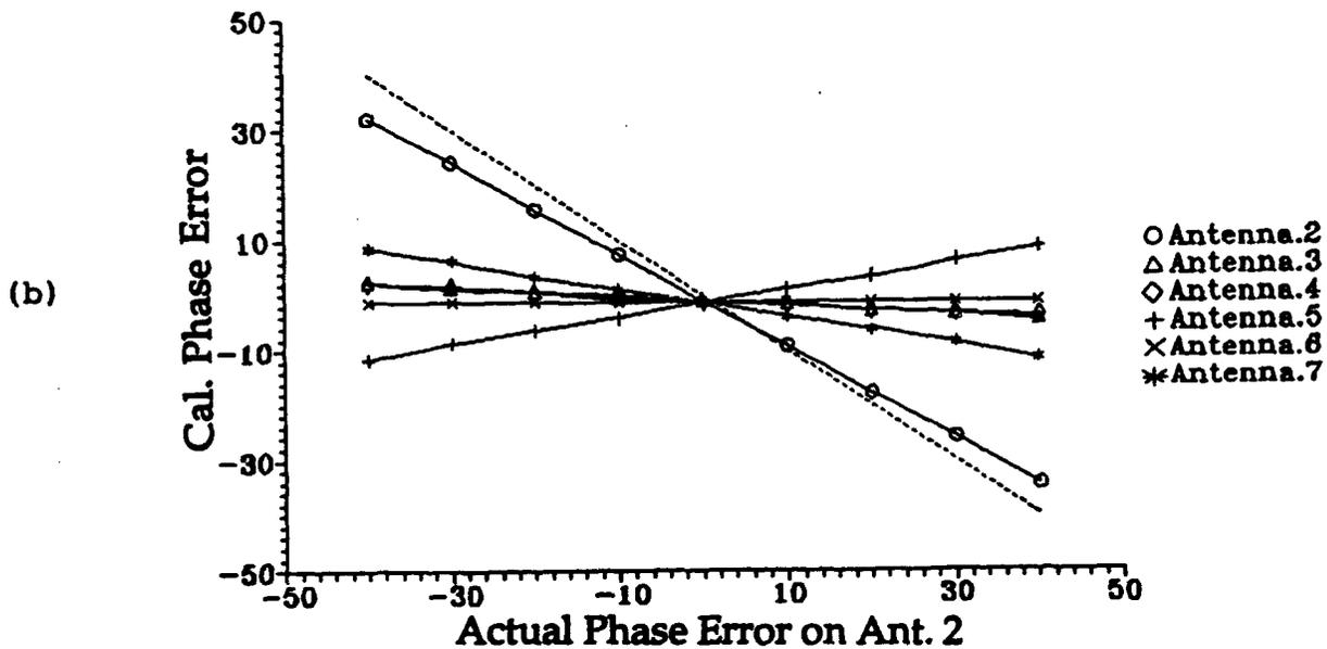
Figure 4. Calculated Phase Errors Using Mode 1.
