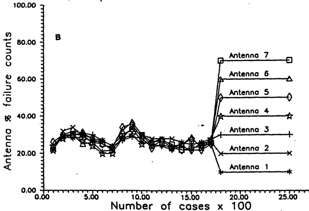
Figure 9. Number of Failure Counts for Phase Testing in Quality Control, Qaanaaq Digisonde 256, Days 87291 through 87293.
