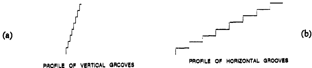
Fig.3. Michelson interferometer with two step mirrors, one with steps oriented horizontally, the other with steps vertically.
