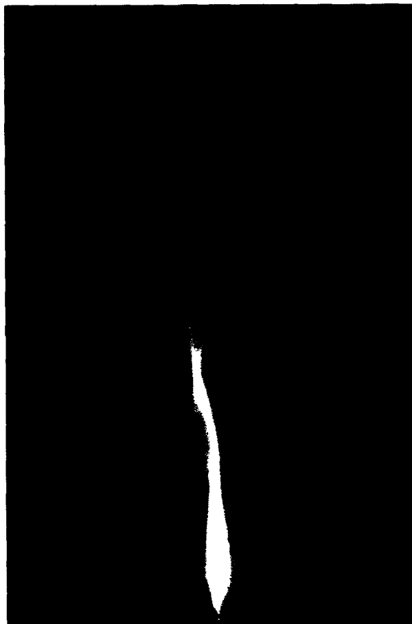
Fig. 2. Longitudinal view of self-focused filaments in the capillary tube configuration of the nematic.
