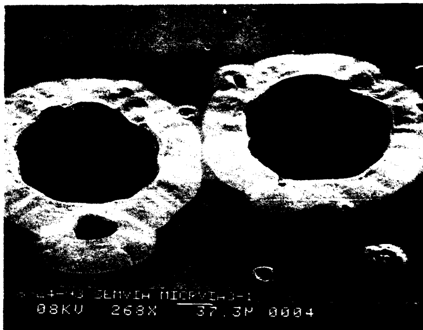
Figure 43. SEM view of silicon vias after Reactive Ion Etching (RIE) with preliminary operating parameters which caused pitting in Al mask and undercutting at via periphery. Etch depth, 95 mm.
