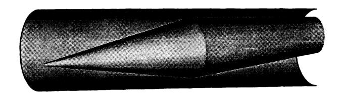
Fig. 26 General geometry of a canted, axisymmetric, three-dimensional projectile used in the numerical simulations. One-half of the full tube is numerically simulated by assuming a plane of symmetry. The computational grid is 150x50x50 in the axial, radial, and azimuthal directions respectively.
