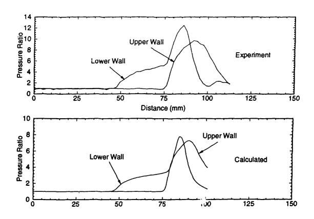
Fig. 31 Comparison of calculated (bottom) and experimental (top) tube wall pressure traces from a canted projectile with estimated angle of attack of 3° and a nose tip translation of 6.5 mm. Superdetonative velocity regime, 1920 m/sec (Mach 5.3) or 110% of the CJ speed. Non-reacting mixture of 2.7CH<sub>4</sub>+7.8N<sub>2</sub>.
