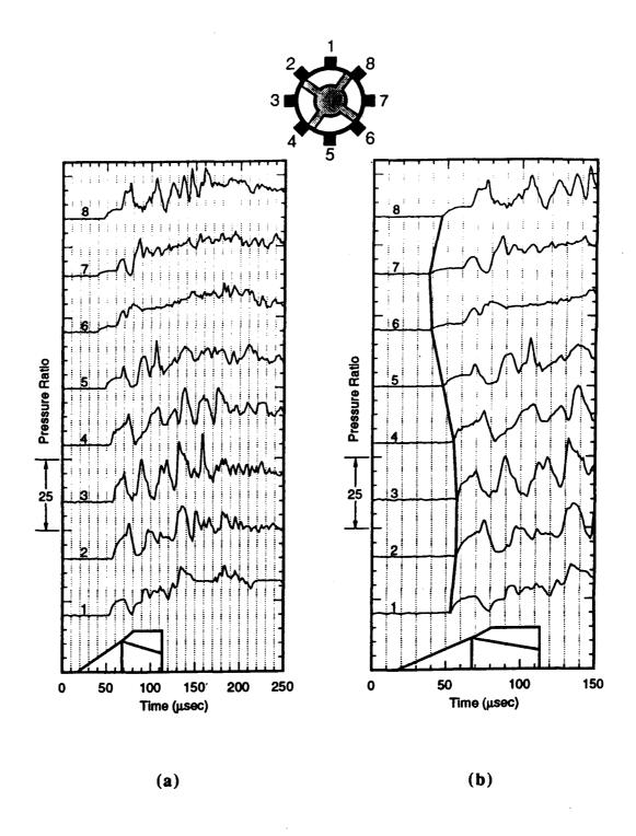
Fig. 20 Tube wall pressure traces from HITS data for a canted projectile traveling at 1560 m/sec (Mach 4.3) or 89% CJ speed. Reacting propellant mixture is 2.7CH<sub>4</sub>+2O<sub>2</sub>+5.8N<sub>2</sub>.
