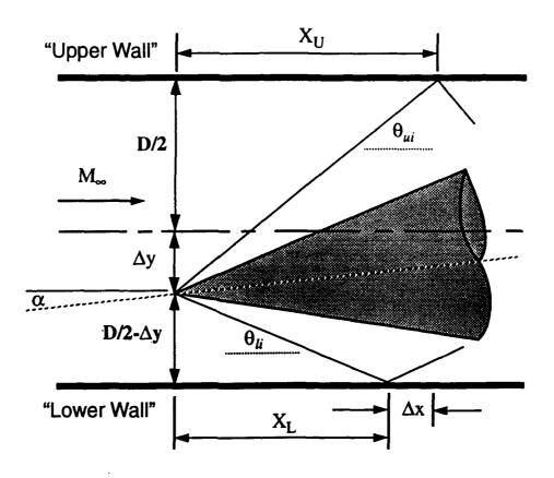
Fig. 21 Notation for determining location of nose tip.
