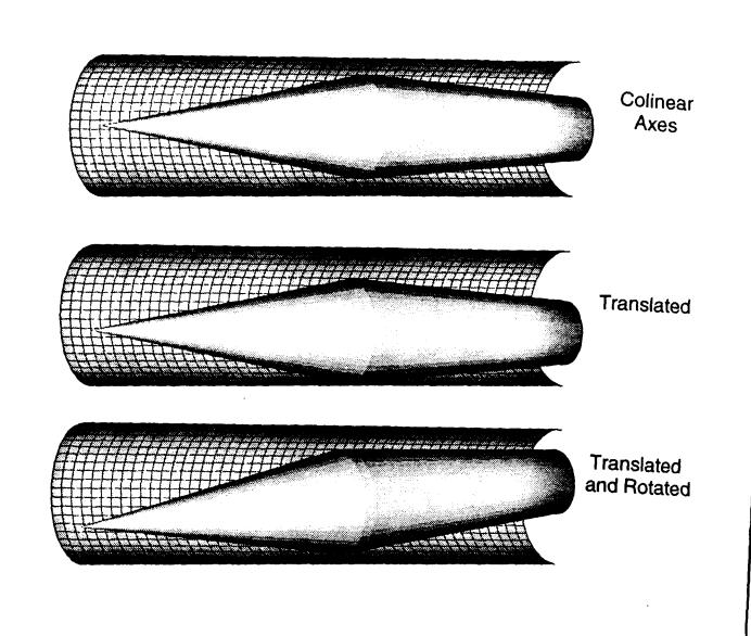
Fig. 18 Three possible positions of a projectile relative to the tube wall.
