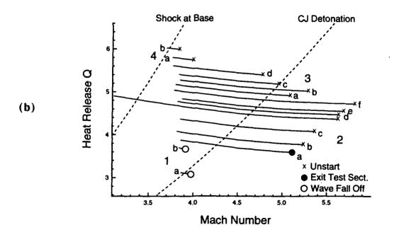
Fig. 14 Low Mach number (M = 3.8) transition experiments:
