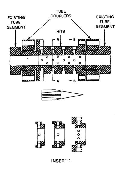
Fig. 5 Highly instrumented tube section and inserts, with projectile shown for scale.
