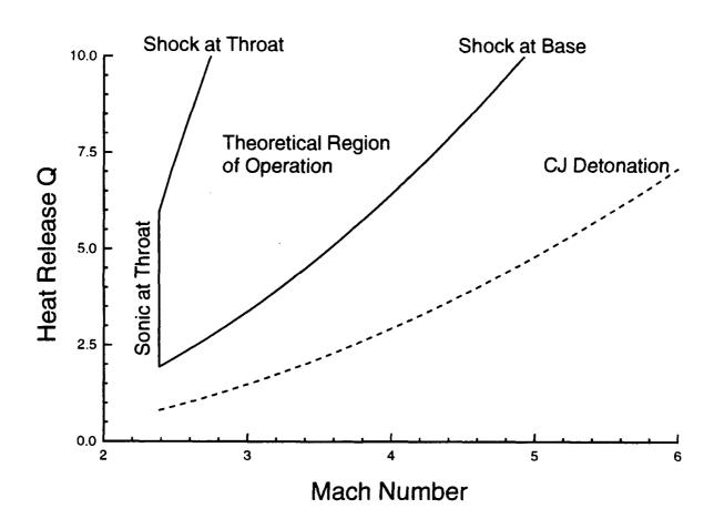
Fig. 8 Operational envelope of the ram accelerator as predicted by one-dimensional theory.
