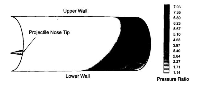
Fig. 32 Three-dimensional surface plot of the calculated tube wall pressure distribution resulting from canting at an angle of attack of 3° and having a nose tip translation of 6.5 mm. Superdetonative velocity regime, 1920 m/sec (Mach 5.3) or 110% of the CJ speed. Surface shading is proportional to pressure. Non-reacting mixture of 2.7CH<sub>4</sub>+7.8N<sub>2</sub>.
