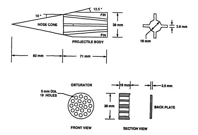
Fig. 6 Projectile configuration used in experiments.
