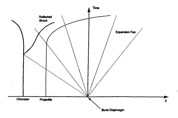
Fig. B-2 Wave diagram of a zero velocity start ram accelerator.
