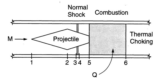
Fig. 7 One-dimensional, quasi-steady model of the thermally choked ram accelerator flow field.
