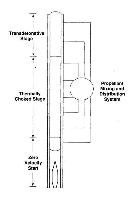
Fig. 36 Schematic of ram accelerator system for launching the LEAP.
