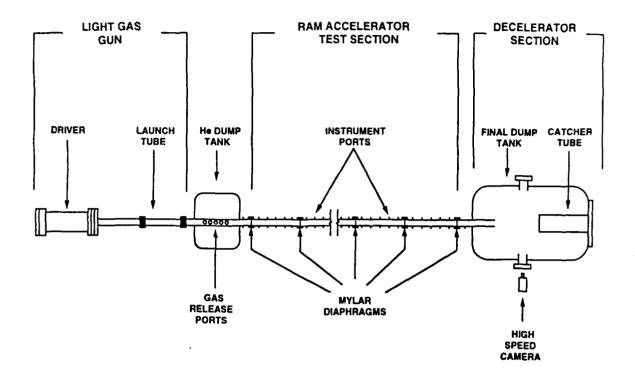
Fig. 4 Ram accelerator experimental facility.
