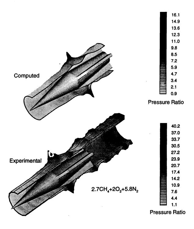
Fig. 22 Comparison of tube wall pressure from experiment (bottom) in reactive mixture to calculated (top) for same gas without reactions. Projectile velocity is 1440 m/sec (Mach 4) or 82% CJ speed. Pressure proportional to both shading and radial distance.
