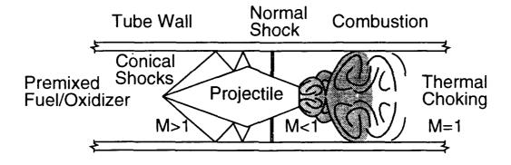
Fig. 1 Schematics of conventional supersonic ramjet and ram accelerator.
