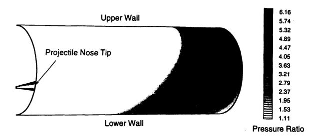
Fig. 30 Three-dimensional surface plot of the calculated tube wall pressure distribution resulting from projectile having an angle of attack of 4.5° and a nose tip translation of 7.5 mm. Subdetonative velocity regime, 1560 m/sec (Mach 4.3) or 89% of the CJ speed. Surface shading is proportional to pressure.
