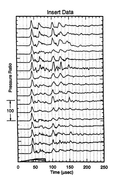
Fig. 33 Tube wall pressure traces from an unstart. Projectile velocity is 2060 m/sec (Mach 5.7) or 118% CJ speed. Note the large amplitude shock wave and the remains of the initial conical shock generated by the projectile nose cone. Reacting propellant mixture is 2.7CH<sub>4</sub>+2O<sub>2</sub>+5.8N<sub>2</sub>.
