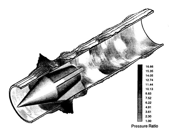
Fig. 24 Representation of tube wall pressure distribution determined from experimental data presented in Fig. 23. Projectile shown for fin orientation and scale.
