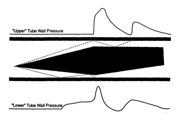
Fig. 19 Illustration of the differences in arrival time of the initial conical shock and the pressure magnitude after its reflection at the opposing sides of a tube for a canted projectile.
