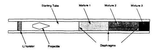
Fig. B-1 Components of a zero velocity start ram accelerator.
