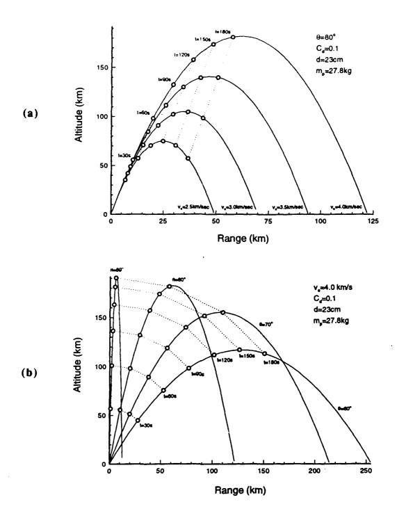
Fig. 38 Trajectories for 30-cm bore ram accelerator launching system:
