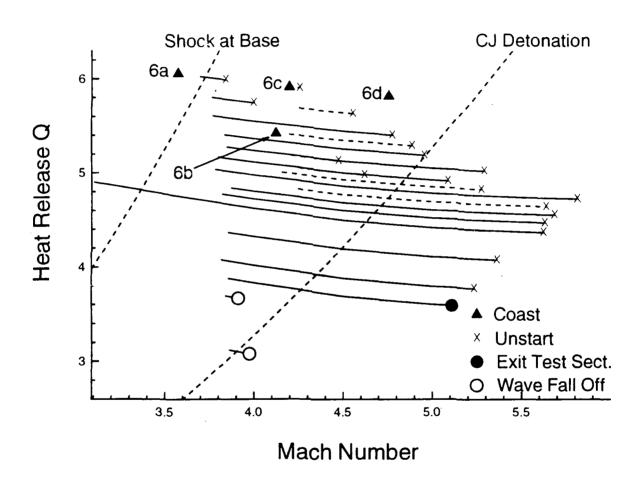
Fig. 17 Observed limits to ram accelerator operation. The triangles indicate experiments in which the projectile successfully coasted several meters in a mixture without unstarting. Dashed lines represent the higher Mach number transition experiments (cf. Fig. 15).
