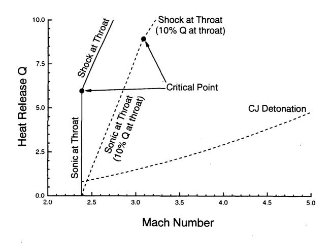
Fig. 9 The effect on the operational envelope of a 10% release of the total Q at the throat. The unstart mechanism changes at the critical point.
