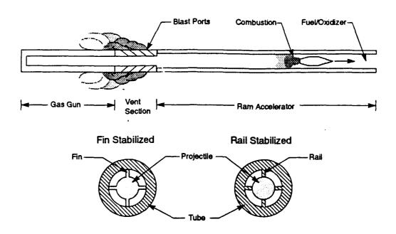
Fig. 2 Ram accelerator with initial launcher. Subcaliber projectile requires fins or rails to center it within the tube.
