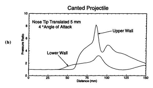
Fig. 27 Non-reacting calculations of upper and lower tube wall pressure ratio for an axesymmetric projectile traveling at 1450 m/sec (Mach 4.0) or 83% CJ speed in 2.7CH<sub>4</sub>+2O<sub>2</sub>+5.8N<sub>2</sub>.
