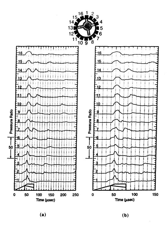
Fig. 25 Tube wall pressure traces from HITS data for a canted projectile traveling at 1920 m/sec (Mach 5.3) or 110% CJ speed. Non-reacting propellant mixture is 2.7CH<sub>4</sub>+7.8N<sub>2</sub>.
