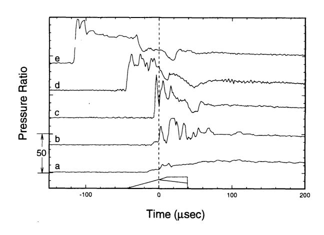
Fig. 11 The evolution of an unstart as seen by tube wall mounted pressure transducers. Time is measured relative to the passing of the projectile throat. Each probe is approximately 40 cm apart. The projectile is traveling at Mach 5.
