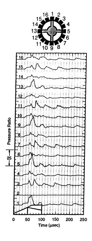
Fig. 23 Tube wall pressure traces from experiment in a non-reacting mixture of 2.7CH<sub>4</sub>+7.8N<sub>2</sub>. Projectile velocity is 1410 m/sec (Mach 3.9) or 81% CJ speed of the equivalent reacting mixture.
