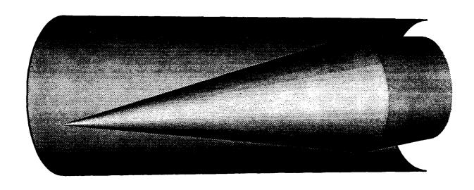
Fig. 28 General geometry of a canted axisymmetric projectile used in the remainder of the numerical simulations. One-half of the full tube is numerically simulated by assuming a plane of symmetry, while only the first 2/3 of the projectile length (102 mm) is simulated. The computational grid is 150x50x50 in the axial, radial, and azimuthal directions respectively.
