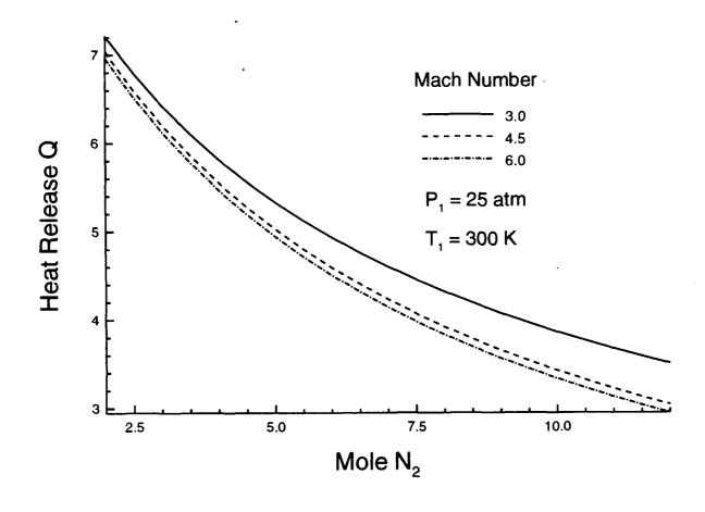
Fig. 12 Thermally choked heat release as a function of nitrogen dilution for 2.8CH<sub>4</sub>+2O<sub>2</sub>+XN<sub>2</sub>.
