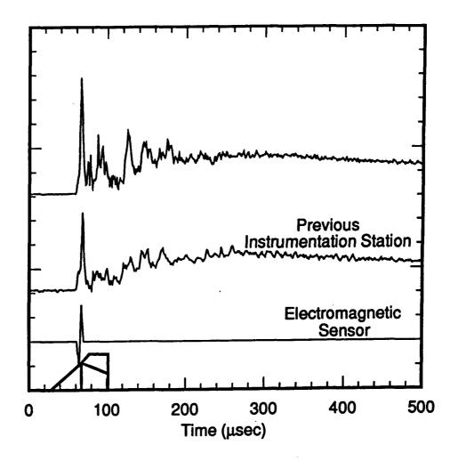
Fig. 34 Comparison of data from trace 1 of Fig. 33 to that of an instrumentation station approximately 22 cm upstream (opposite in direction of projectile motion) with the same azimuthal orientation. Magnetic sensor data correlate projectile position with the pressure traces. Note difference in shock pressure peak amplitude.
