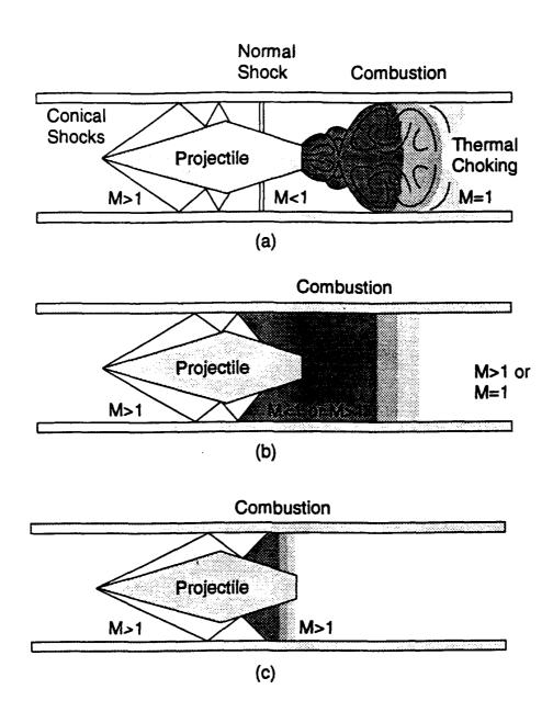
Ram accelerator propulsive cycles for three different velocity regimes:
