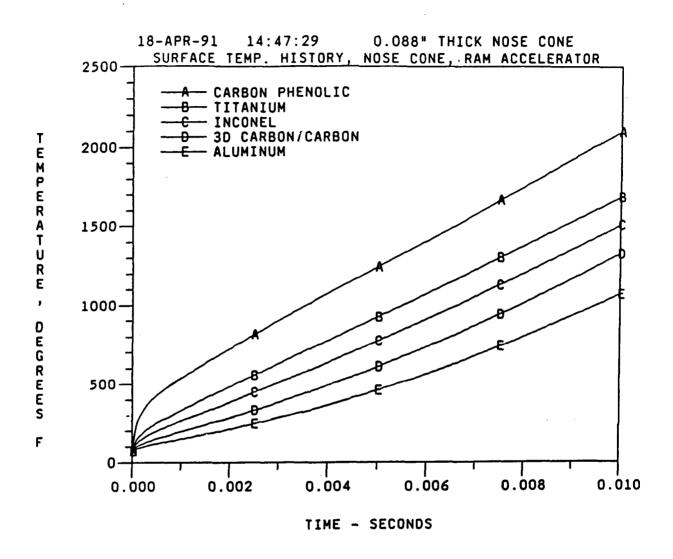
Fig. 39 Surface temperature history of 12.5° half-angle nose cone accelerated in a 33 atm propellant mixture from Mach 2.4 to Mach 7.
