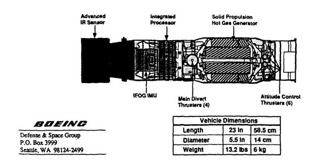
Fig. 35 Schematic of LEAP configuration proposed by the Boeing Company for rocket launch.
