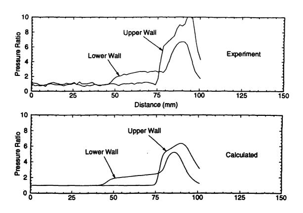
Fig. 29 Comparison of calculated (bottom) to experimental (top) tube wall pressure profiles from a canted projectile with estimated angle of attack of 4.5° and a nose tip translation of 7.5 mm. Subdetonative velocity regime, 1560 m/sec (Mach 4.3) or 89% CJ speed.
