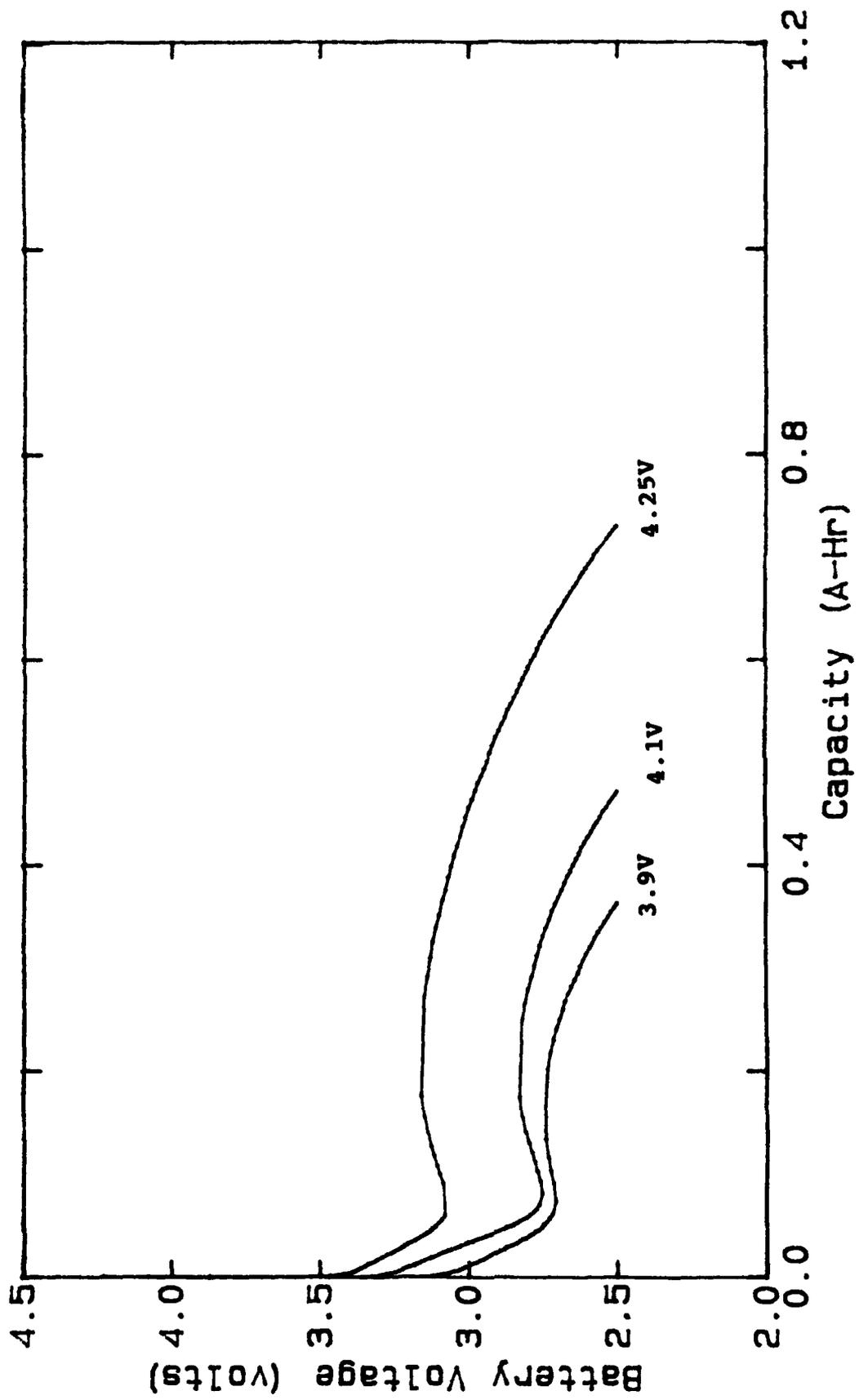
FIGURE 8. DISCHARGE CAPACITY AT 0.5 AMPERE AT -20°C AFTER CHARGE TO 4.25, 4.1, AND 3.9 VOLTS AT 25°C.
