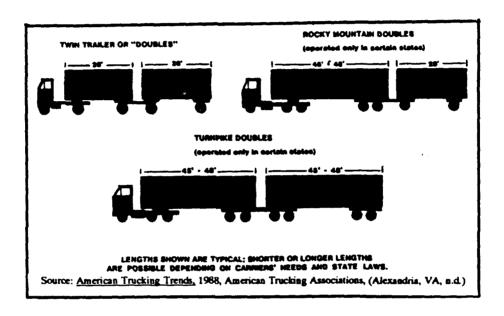
These configurations provide certain types of trucking operations an additional flexibility and efficiency in the use of equipment that is impossible to achieve with conventional tractor-trailer combinations. But, most motor carriers are currently prevented from operating LCVs nationally. A brief discussion of federal regulation on motor vehicle sizes and weights is necessary to understand why.
