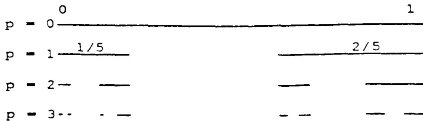
Figure 5.3: Recursive operation for building a multifractal Cantor measure. The Cantor measure is obtained at the limit of this iterative procedure.
