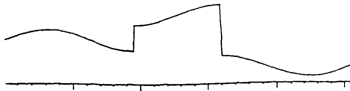
Figure 6.1d: Signal reconstructed from the wavelet transform local maxima shown in Figure 6.1c.
