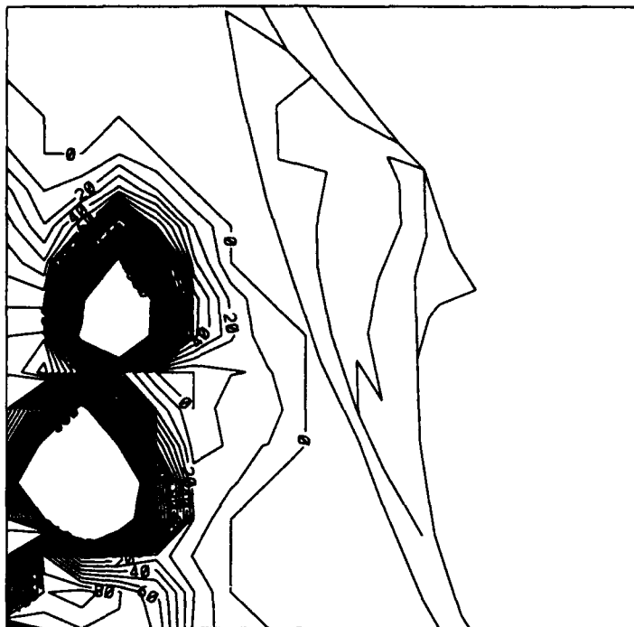
Figure 3.44: Condensate mixing ratio (g/g), elevation = 48.6 m, contour = 1 E-5 g/g, maximum contour = 39 E-5; 00Z 30 July
