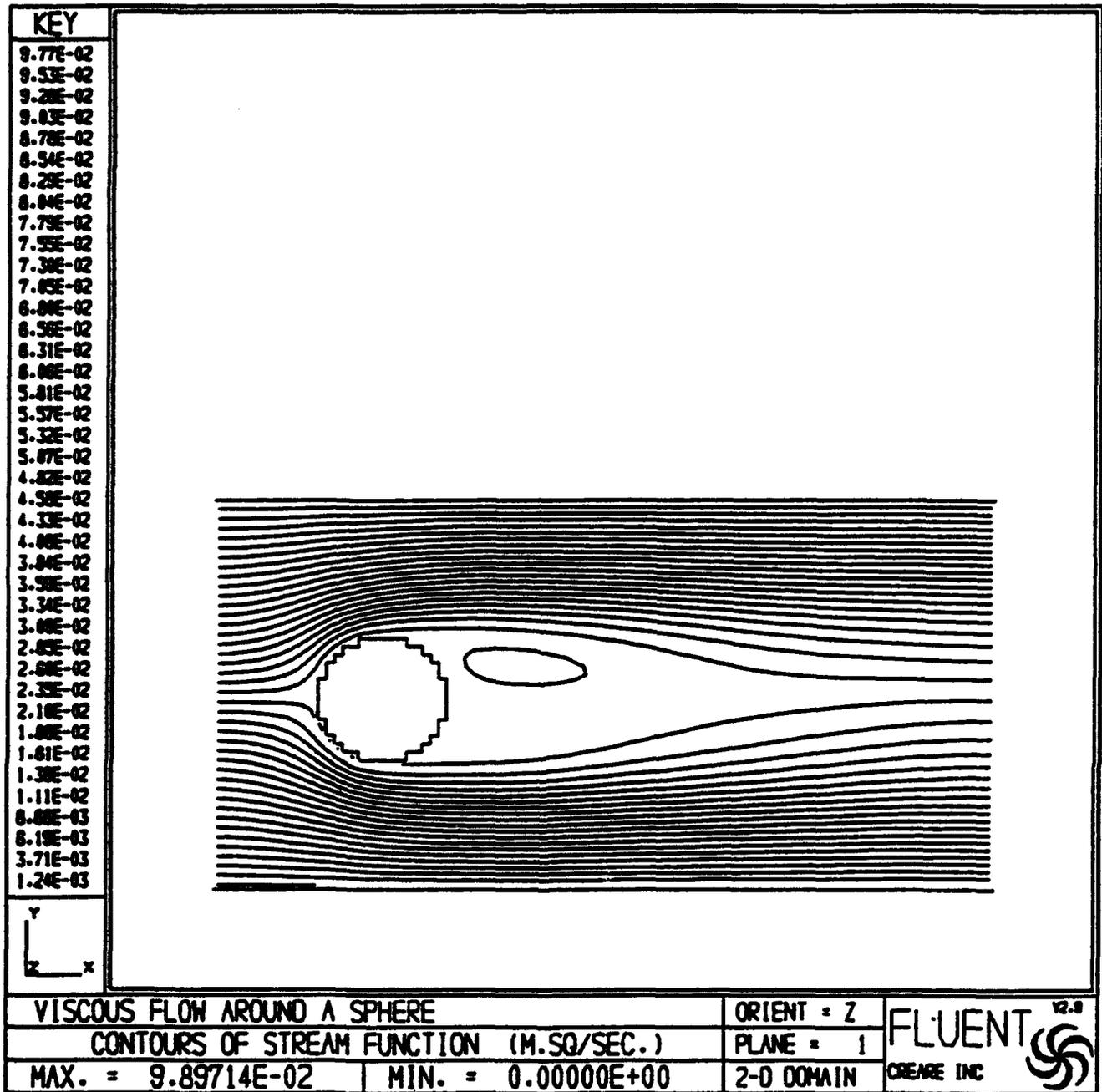
Figure (3) - FLUENT Generated Streamlines For Flow of Air Around a UV Lamp in a Uniform Flow Field
