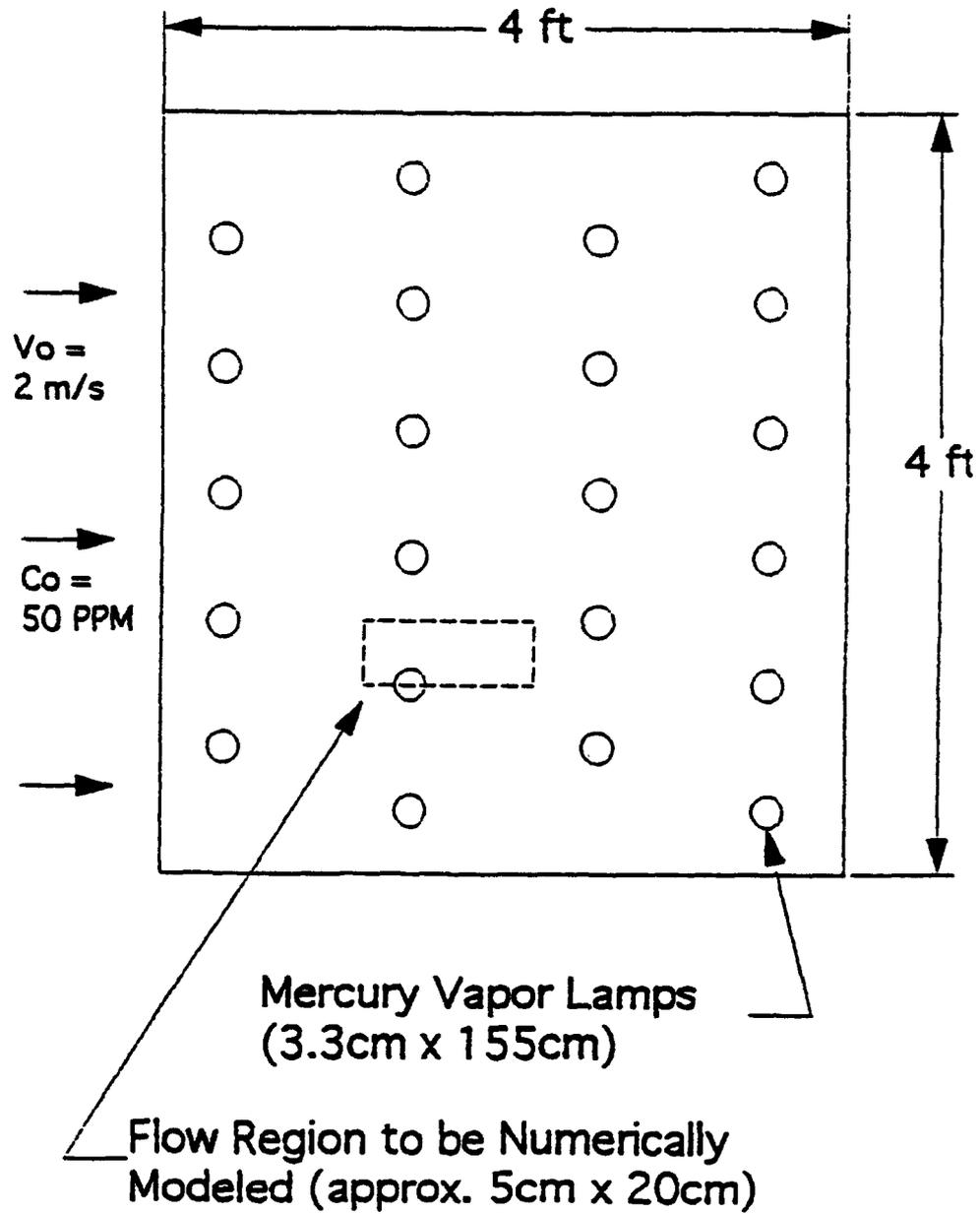
Figure (2) - VOC Pollution Control Device Photolytic Reactor
