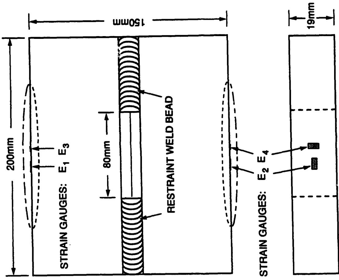
Fig. 12. Schematic illustration of a strain gauge instrumented Y-groove specimen (after Matsuda et al [1984]).
