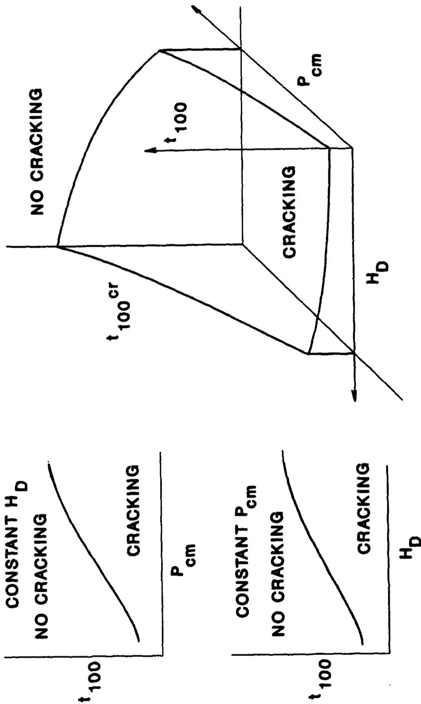
Fig. 15. Schematic response surface for hydrogen cracking resistance.
