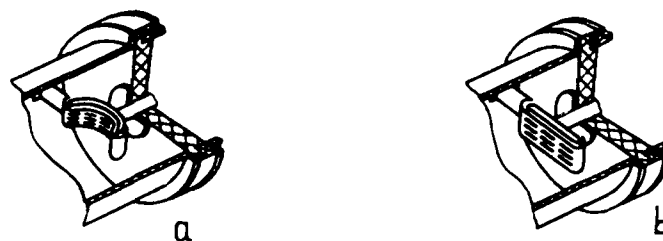
Fig. 2. Schematic diagrams of magnetically insulated diodes. a - strip diode; b - focusing diode.
