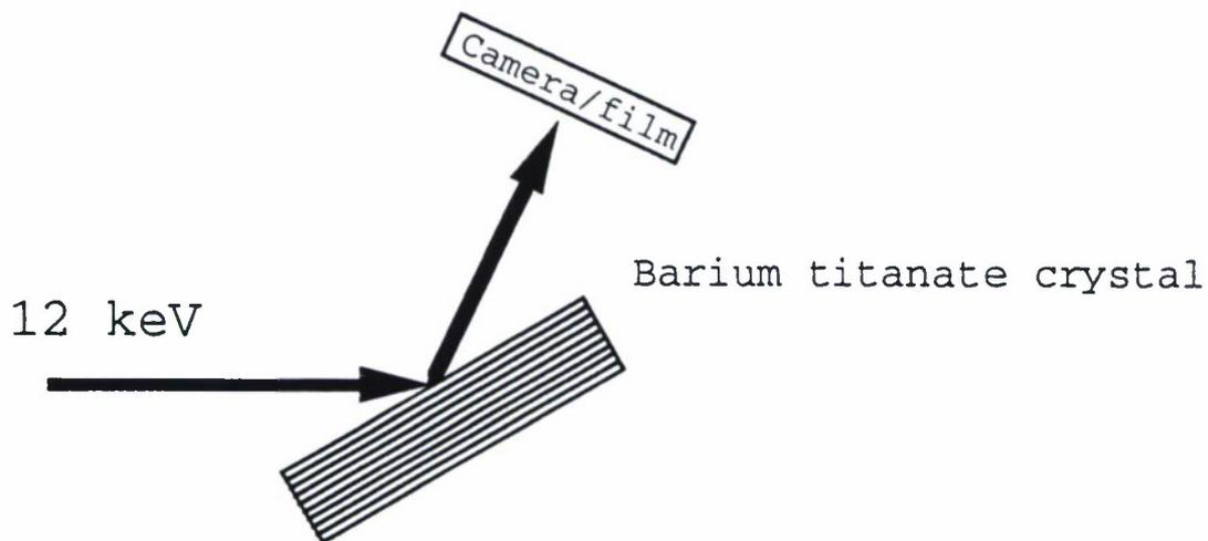
Figure 1: Schematic representation of diffraction imaging geometry.
