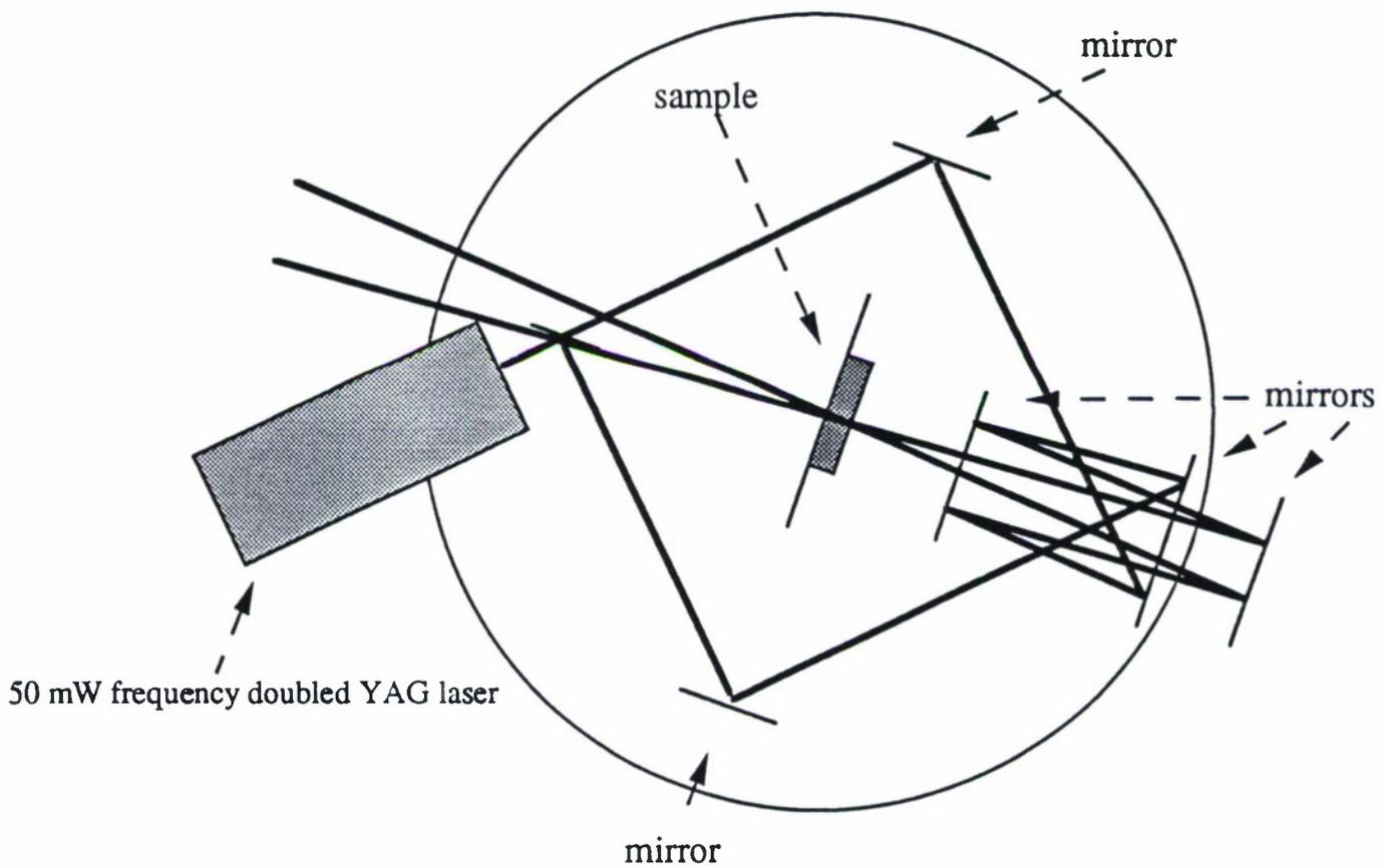
Figure 16a: Schematic of the apparatus used to write photorefractive gratings on beamline X23A3 at the National Synchrotron Light Source. The beam from the laser is split, and the two resulting beams are interfered at the crystal to produce the grating. The complicated beam path is to achieve a small angle between the beams necessary for long period ( $>50\mu\text{m}$ ) gratings. The entire assembly rotates as a unit to allow changes in Bragg angle without altering the grating.
