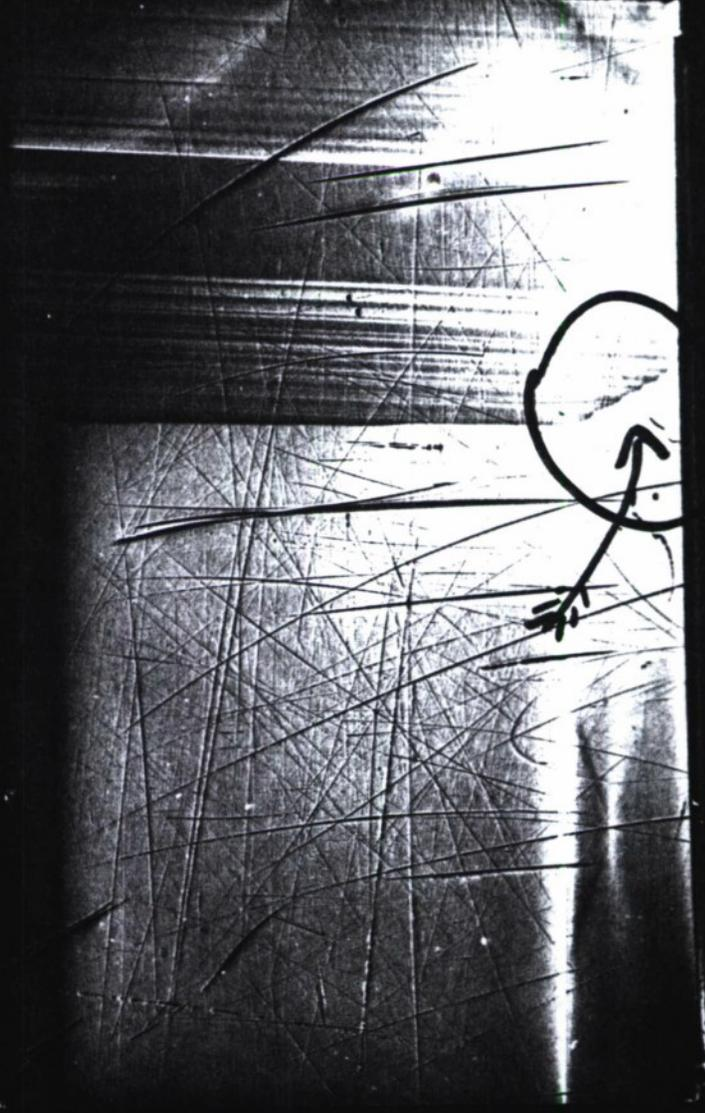
Figure 11: (400) diffraction image of crystal 20F18-2 in Bragg geometry at 10keV, showing growth faceting, facet competition, and growth striations.
