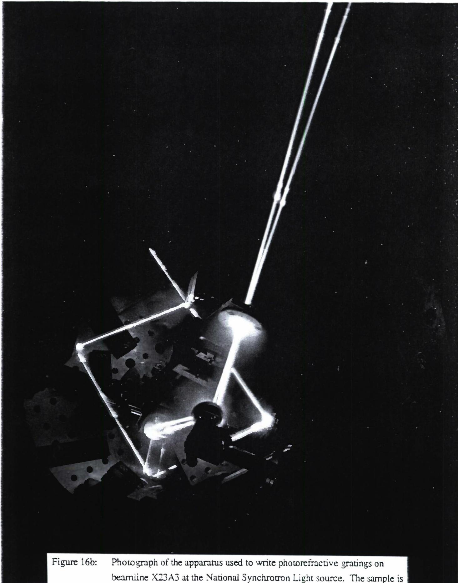
Figure 16b: Photograph of the apparatus used to write photorefractive gratings on beamline X23A3 at the National Synchrotron Light source. The sample is near the center of the photo, where the beams intersect.
