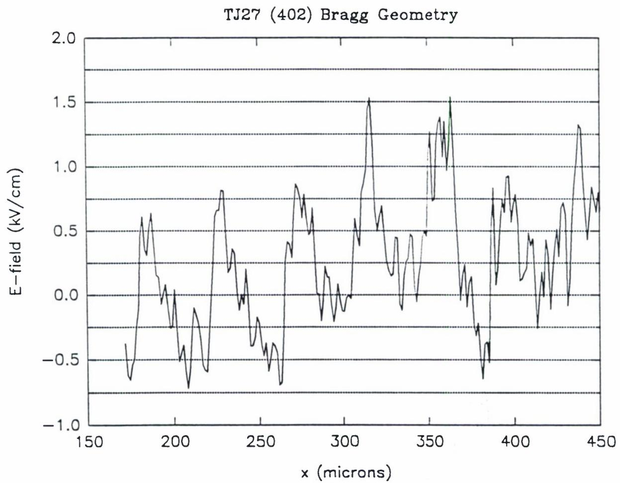
Figure 19: Photorefractive space charge field calculated from (402) Bragg geometry rocking curve sequence at 12keV.
