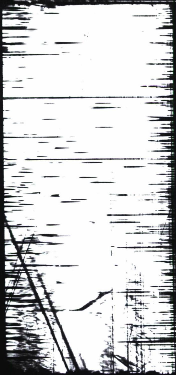
Figure 4: (002) diffraction image of crystal BTUC2 in Laue geometry (transmission) at 12keV. The linear features running horizontally are edge dislocations, and needle or spike like features running vertically are 180 degree domains.
