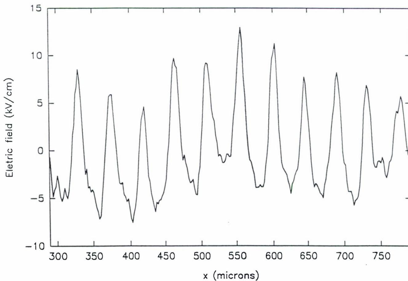
Figure 21: Photorefractive space charge field calculated from (400) Bragg geometry rocking curve sequence at 12keV.
