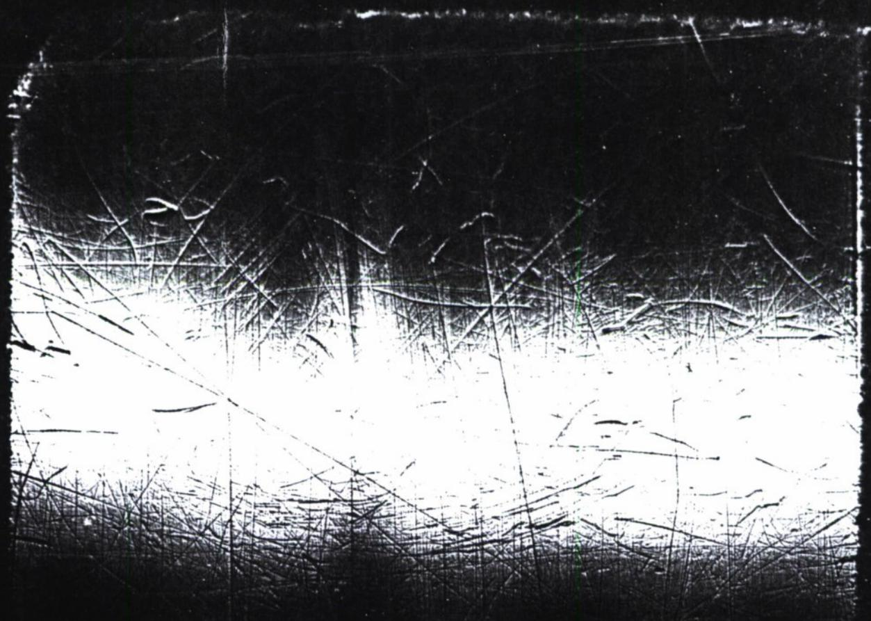
Figure 13: (800) diffraction image of SBN sample SBNSU1 in Bragg geometry at 8keV, showing surface scratches and lattice warping.
