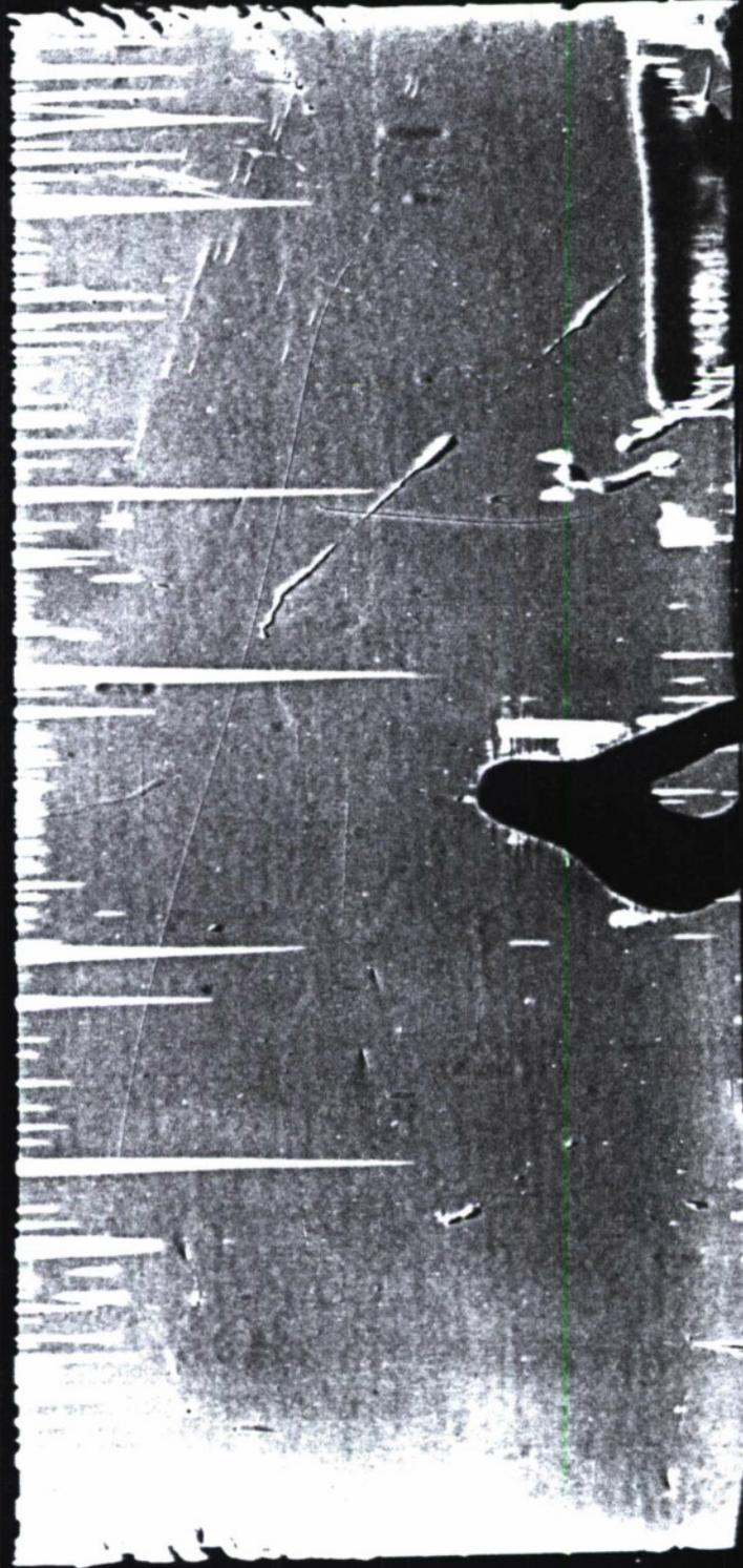
Figure 9: (402) diffraction image of crystal BTUC2 in Bragg geometry at 12keV, showing shrinkage of domains after application of 360 V/cm electric field parallel to c-axis.
