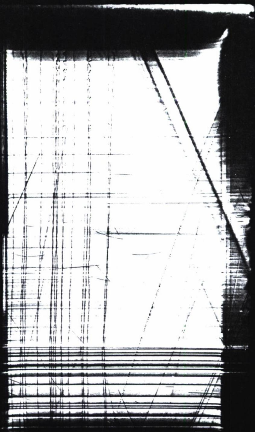
Figure 10: (020) diffraction image of crystal BTUC2 in Laue geometry at 12keV, showing growth striations, and screw dislocations running horizontally.
